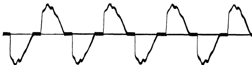
Fig. 70. Alternating e.m.f. impressed upon rectifier tube.
