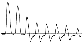
Fig. 47. Starting current of a 25-cycle transformer.
