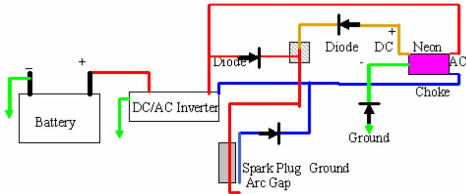
You could also use a higher voltage transformer instead of the neon choke but these are often custom-made.
