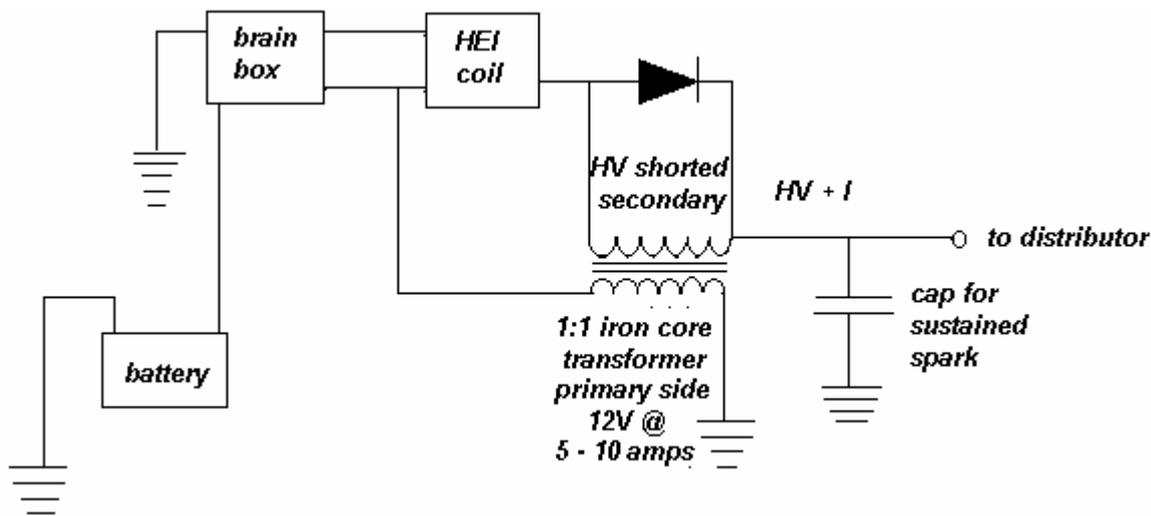
Option 3: The switching transistor is done away with and current is sourced from the electronic ignition circuit ("brain box") and passed directly to both the ignition coil and the transformer. This simplifies the wiring but may possibly halve the total amount of power sent to both. The effect of extra current demand through the brain box to power both coils is unknown. There is the danger of frying the brain circuitry.
