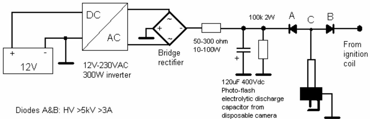
The inverter charges up the 120uF Photo-flash capacitor to about 300Vdc. The resistor (or lamp or an inductor) is used to limit the charging current to the capacitor. The polarities of the bridge rectifier, capacitor and two diodes are reversed, because it seems that the engine's ignition circuit gives a better spark in the negative direction.
