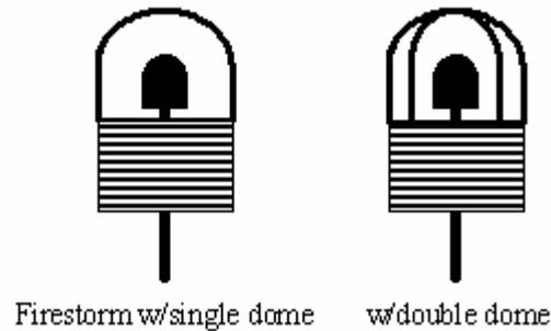
If these plugs ever come onto the market, they have very good potential for plasma fog jet engines as they create a plasma ball type explosion around the electrode. Till then you will have to make your own which could be done by welding a small dome onto the central electrode and then a wire dome over the top. Prototypes may not look that pretty, but they should work.
