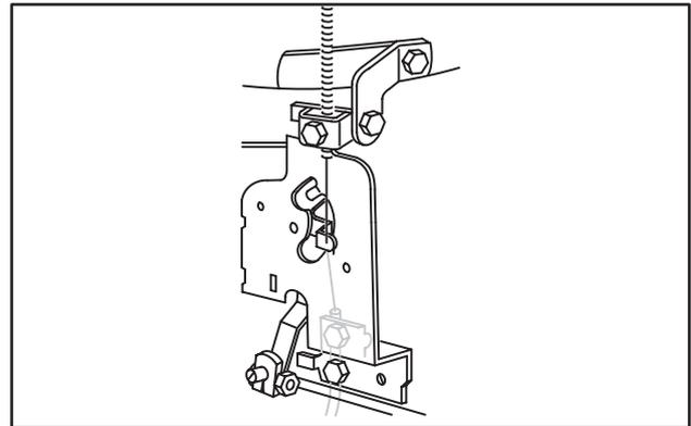
**Fig. 10 – Early Style, 170700, 171700, 190700, 191700, Swivel Control Bracket for Briggs & Stratton One Piece Flo-Jet Carburetors**
