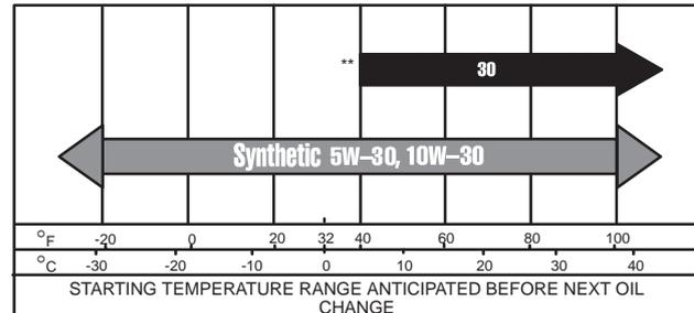
\* Air cooled engines run hotter than automotive engines. Use of non-synthetic multi-viscosity oils (10W-30, etc.) in ambient temperatures above 40° F (4° C) will result in high oil consumption. If multi-viscosity oil is used, check oil level more frequently to prevent engine damage due to lack of lubrication.
