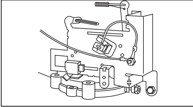
**Fig. 6 – 194700, 195700, 196700, 254700, 257700, 258700, 259700, 28A700, 28B700, 28C700, 28D700, 28E700, 28M700, 282700, 283700, 285700, 286700, 288700, 289700 with Horizontal Rack & Pinion control for Briggs & Stratton/Walbro LMT Carburetors**
