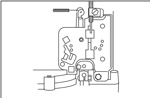
**Fig. 7 – 170700, 190700, 191700, 192700, 193700, 194700, 195700, 196700, 220700, 252700, 253700, 254700, 257700, 256700, 258700, 280700, 28A700, 28B700, 28C700, 28D700, 28M700, 283700, 286700, 289700 with Vertical Rack & Pinion Control for Briggs & Stratton/Walbro LMT Carburetors**
