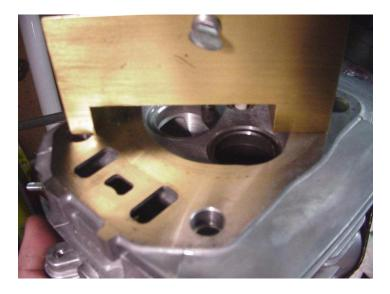
C. Measure from surface of head to lowest machined area in the bowl of the port. This dimension will be:
