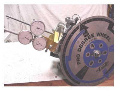
Cam will be checked with indicator reading off the top end of tappets, which will provide zero clearance. The inverted radius of the top of the tappet presents some problem to get accurate readings and to prevent binding of indicator stem. Indicator holder and positions are very critical in this operation. Zero indicator on base circle of cam. Be sure that compression release does not affect zeroing exhaust indicator. Zero dial indicator after exhaust bump (0.050) ref.
