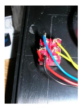
This photo shows the original SPDT gating switch changed for a DPDT version allowing the normally 'open' part of the circuit to be bridged and the gating side of the circuit to function as normal.
