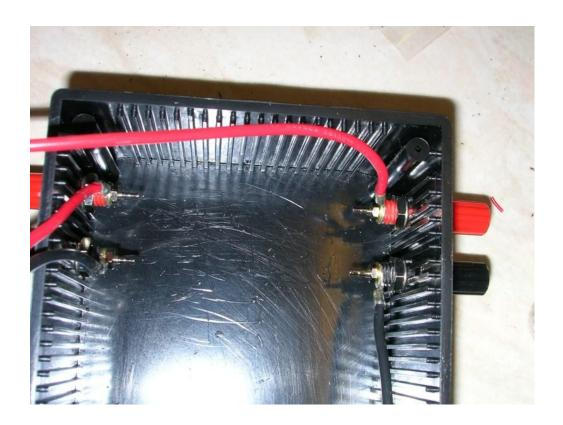
6. The next picture shows the PCB mounting arrangement. This consists of 2off 3mm bolts secured with 2off nuts each to act as spacers.
