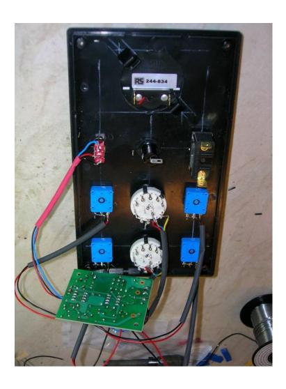
5. We supply a number of crimp connectors and solder ring terminals with the kit. We prefer to connect to the 4mm input/ output terminals using the 4mm ring terminals, you can equally solder direct to these if you wish.
