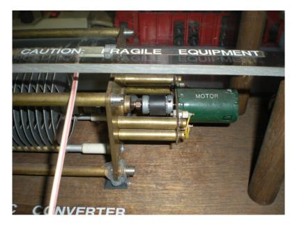
The fourth picture shows an end view when the rotor plates are in alignment with the stator plates. This is the position for highest capacitance in that section.
