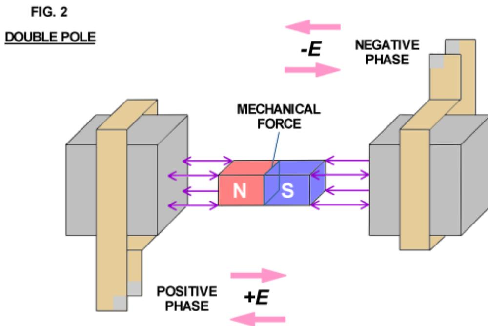
It is desirable that the mechanical energy produced or consumed be of rotational form in order to operate pumps, engines, turbines, etc. The method of producing rotary force, without the use of mechanical rectifiers known as commutators, was discovered by Nikola Tesla in the late 1800s and is known as the rotating magnetic field.
