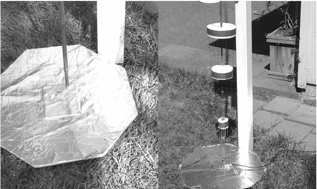
Photo 6: All-Band Antenna measurement setup, simple vertical with good grounding (left) and with SWTL launcher and VHF antenna on top (right). In addition to the hexagonal aluminum foil disk, which provides a good VHF ground, an 8' ground rod near the wooden post is also connected to the disk and this arrangement is left in place for all measurements even though the disk is not necessary when the launcher is in place.
