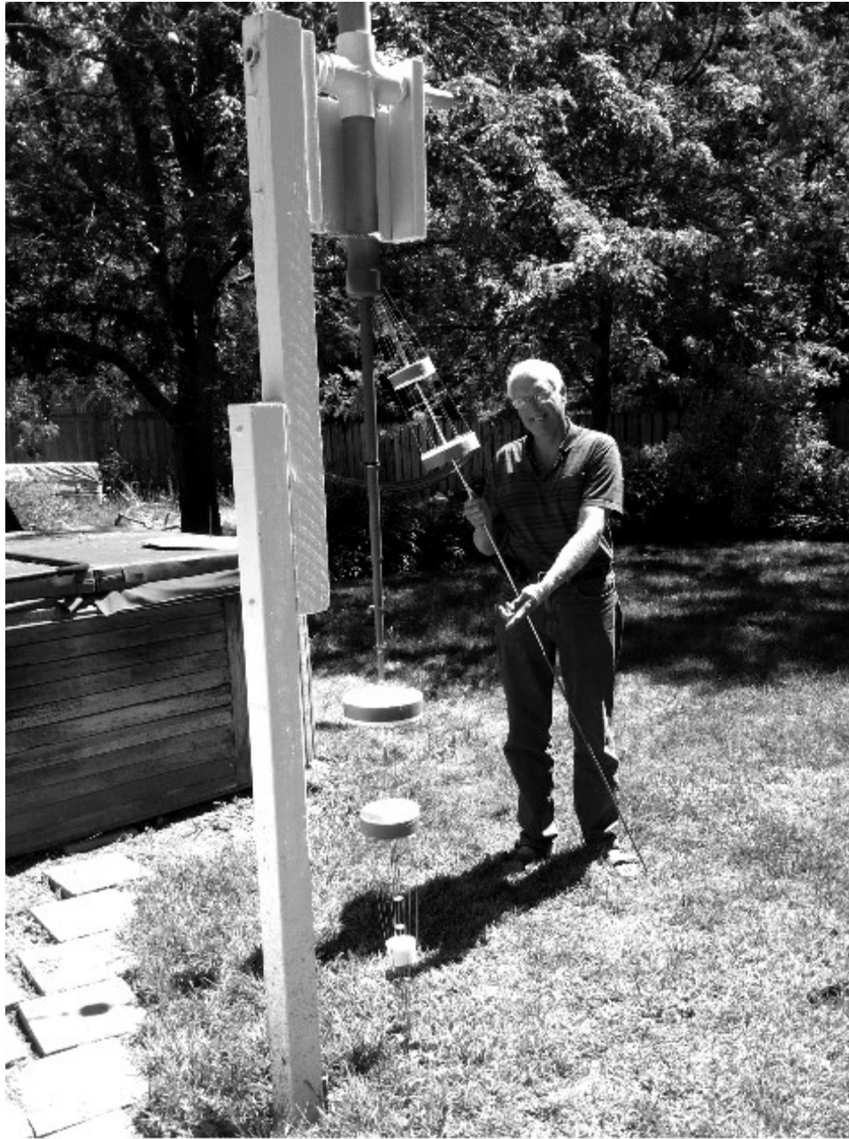
Photo 7: N6GN holding a bottom launcher and pointing at a second launcher installed at the base of the All-Band HF/VHF/UHF antenna. The tilter detail can be seen in this photograph and can be constructed similarly. Use the largest size plastic pipe that is practical to allow as much air space around the aluminum tubing as possible.
