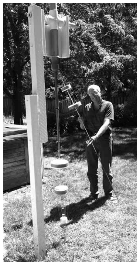
Photo 1 — N6GN holding a bottom launcher and pointing toward a second launcher installed at the base of the All-Band HF/VHF/UHF antenna. The PVC tilter can be seen in this Photo. Styrofoam doughnuts have been added to keep the center conductor concentric with the outer cone.
