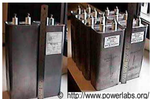
7 AEROVOX Energy Discharge Capacitors, rated at 5200V, 23uF (311J) each. ESL is 150nH. Peak current 5000A repetitive (12.5kA non-repetitive)
