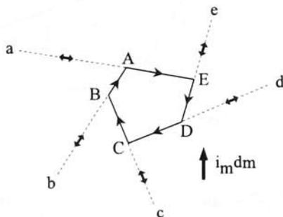
Figure 1.16 : Grassmann's angle-current representation of a closed circuit
