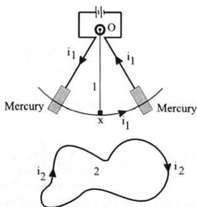
Figure 1.7 : Ampère's wire-arc experiment
