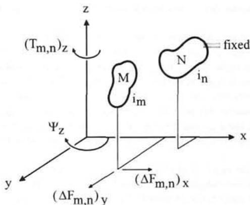
Figure 1.11 : Parameters used for electrodynamic torque calculations
