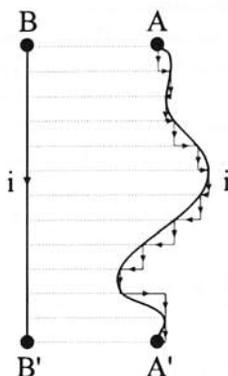
Figure 1.9 : Equivalence of bent and straight wire sections
