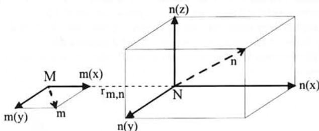
Figure 1.4 : Resolved component vector representation of the two general current elements of figure 1.3
