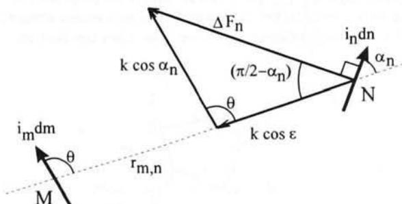
Figure 1.17 : Force triangle used to prove equality of Eqs. 1.58 and 1.59
