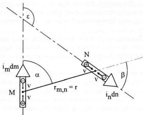
Figure 1.18 : Weber's model of two current elements
