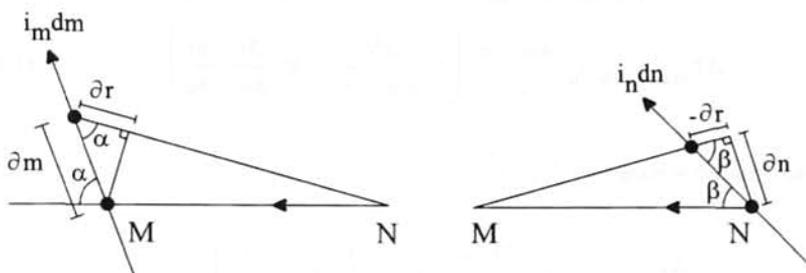
Figure 1.6 : Partial differentials of the distance vector with respect to displacements of current elements
