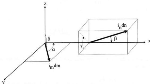
Figure 1.5 : Angles for determining the direction cosines of two general current elements
