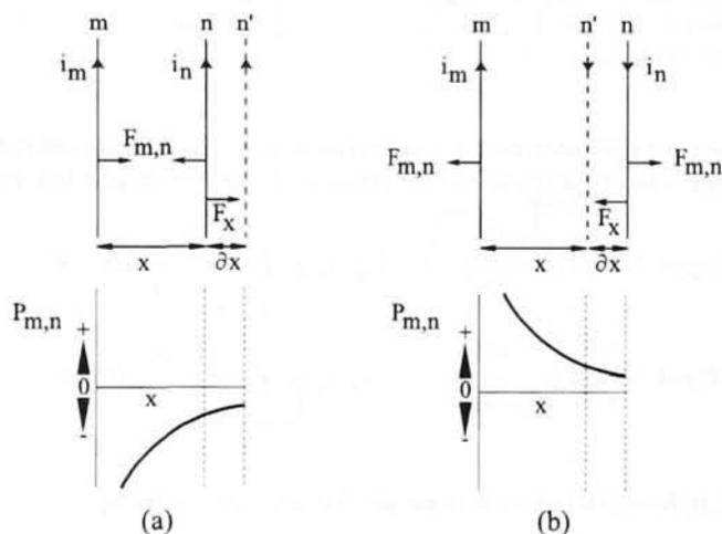
Figure 1.10 : Electrodynamic potential energy of straight and parallel currents
