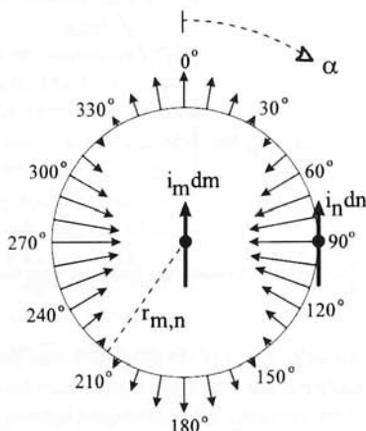
Figure 1.15 : Polar diagram of the Ampère force between two parallel current elements with a constant distance of separation
