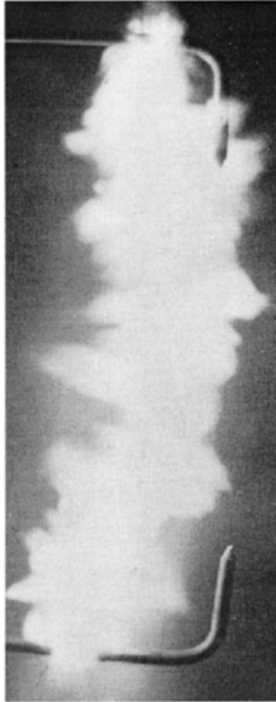
Figure 2. Trowbridge's (1907) photograph of a cold fog explosion. The arc is \sim 40 cm long.
