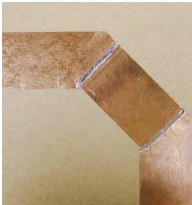
Figure 1. Soldered Antenna Corners
