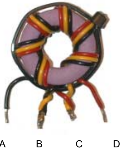
Figure 23. How to Wind The BALUN
