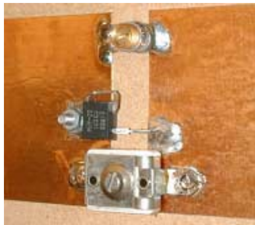
Figure 12. Resonant Capacitors and Damping Resistor
