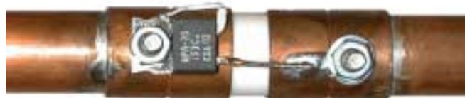
Figure 3. Assembled Tube with Damping Resistor
