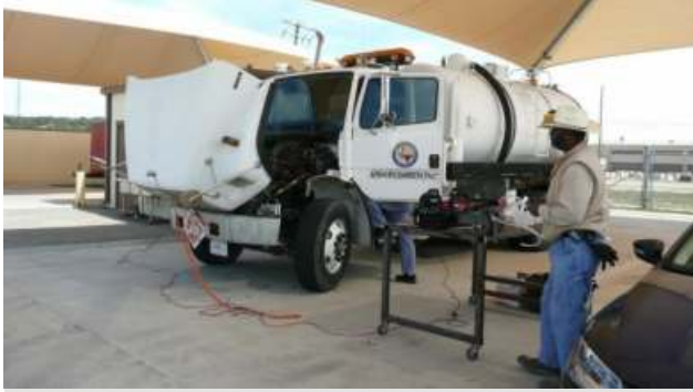
Todd Fowler, CHI's president, works to establish baseline fuel economy prior to installation of his firm's hydrogen fuel injection system. (Photo: CHI)
