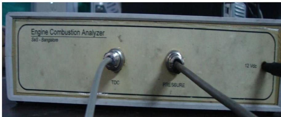
**Figure 4.12** Photographic view of combustion analyzer
