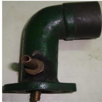
**Figure 4.14** photographic view of OEH gas induction point
