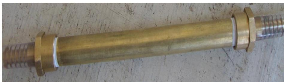
**Figure 4.24 Photographic view of flame trap**
