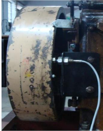
**Figure 4.11** Photographic view of crank angle detector
