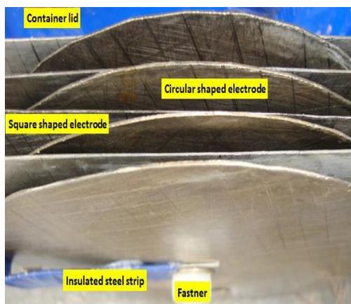
**Figure 4.18** Photographic view of stack of electrodes
