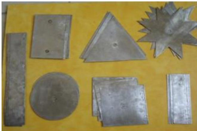
**Figure 4.20** Photographic view of various shapes of electrode
