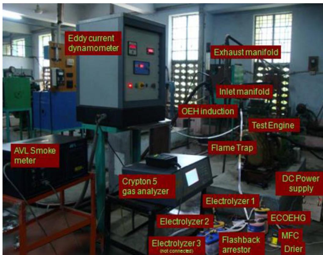
**Figure 4.1** Photographic view of experimental set up
