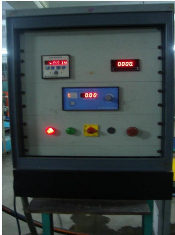
**Figure 4.3** Photographic view of control panel of eddy current dynamometer
