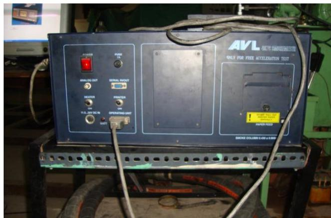
**Figure 4.8 Photographic view of smoke meter**
