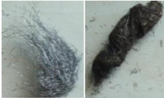
**Figure 4.25** Photographic view of steel wool before and after backfire from engine
