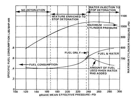
Enriching the air/fuel ratio is another method of preventing detonation when the engine is in the supercharged condition. This method will work up to a certain limit and beyond that the engine will detonate regardless of how rich the mixture is. At this point either water or water-alcohol injection are required to prevent detonation.
