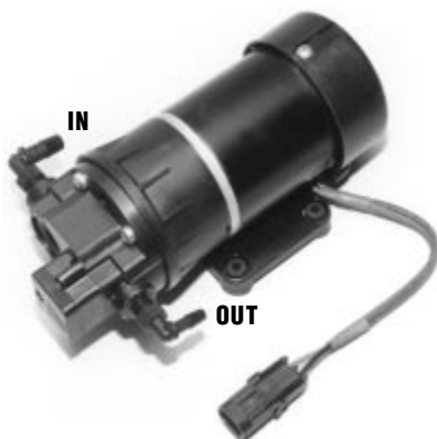
TYPICAL HIGH-PRESSURE GASEOUS INTERCOOLING™ PUMP • A25011 SHOWN WITH 40°-3/8" BARBED HOSE INLET AND 90°-1/4" BARBED HOSE OUTLET
