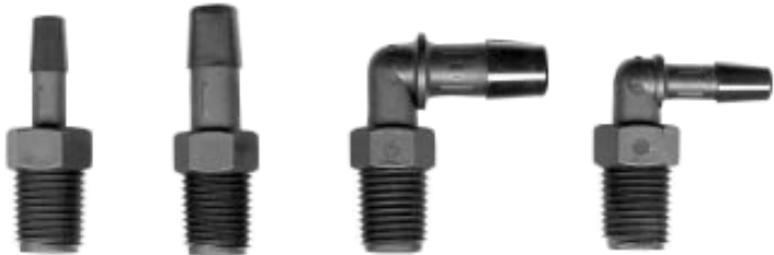
1/4" MPT x 1/4" BARB A4-4BN 1/4" MPT x 3/8" BARB A4-6BN 1/4" MPT x 3/8" BARB ELBOW L4-6BN 1/4" MPT x 1/4" BARB ELBOW L4-4BN
