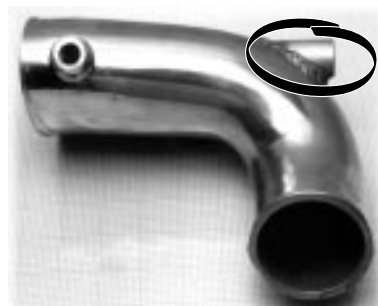
TYPICAL WELD-O-LET NOZZLE ADAPTOR ON AIR DISCHARGE TUBE 1077
