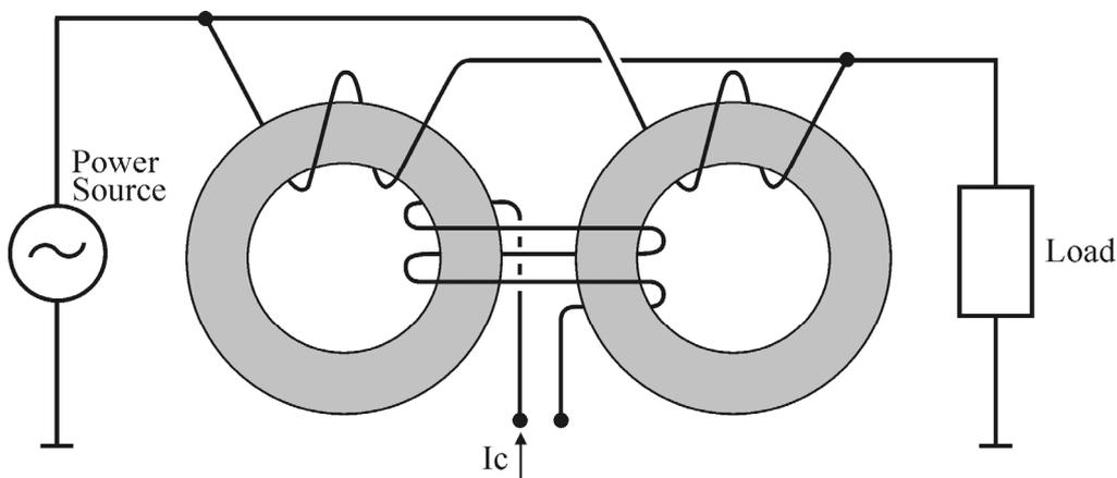
Fig. 8. Two cores with parallel power windings
