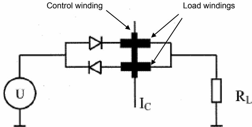
Fig. 30. Principal circuit of a one-phase magamp
