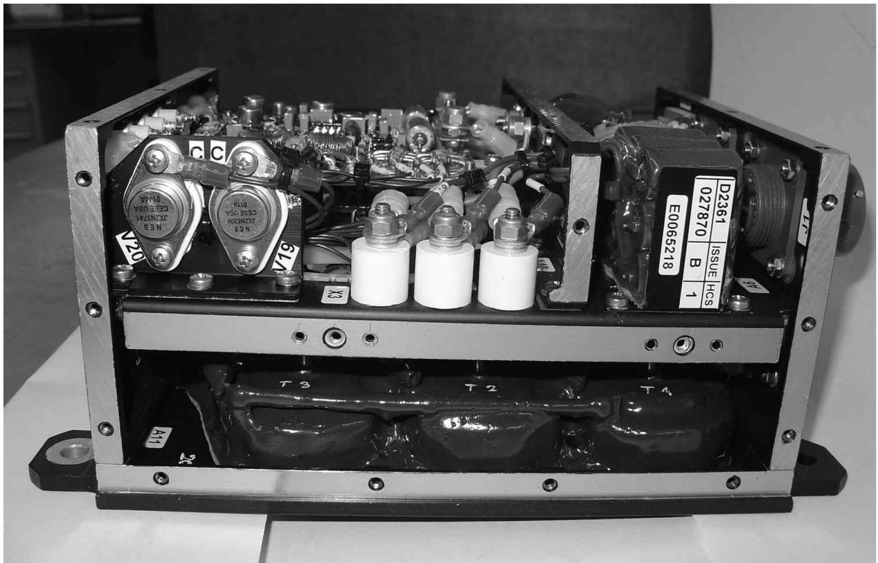
Fig. 28. The final assembly of the magnetic amplifier (photo Euroatlas)
