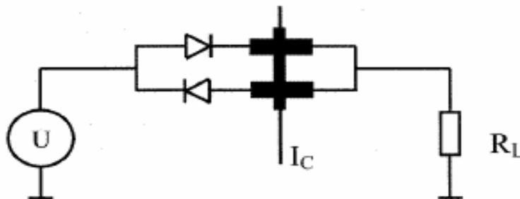
Fig. 16. The one-phase self saturating magamp
