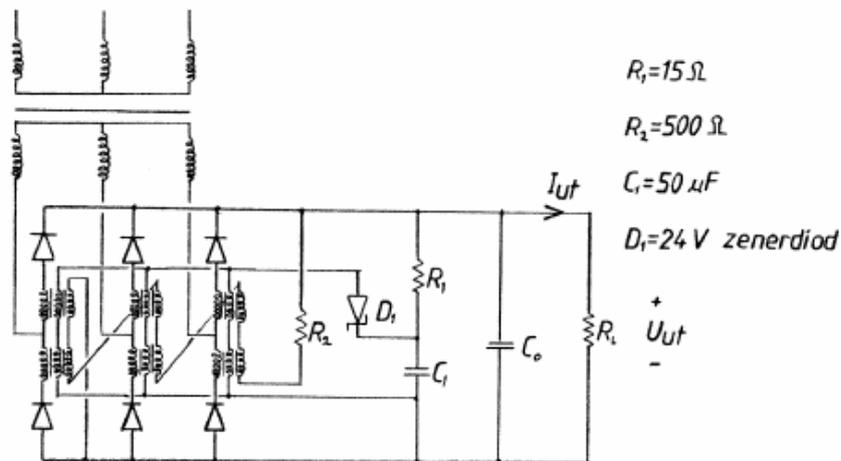
Fig. 58. Shows a TRU with controlled output voltage [46].
