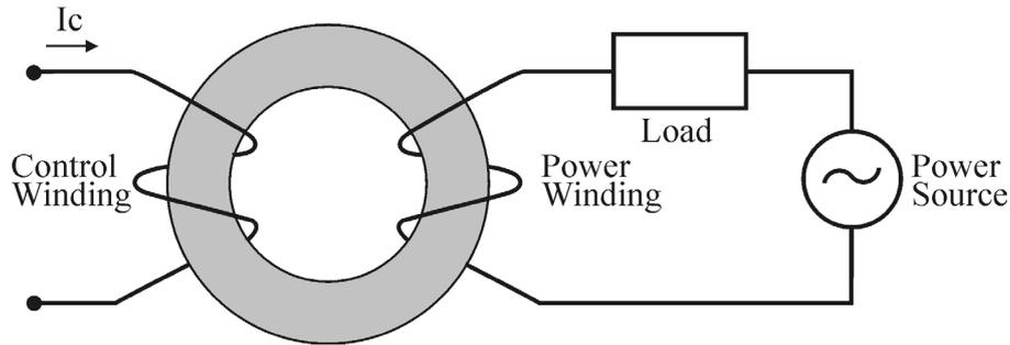
Fig. 5. The one-core magnetic switch
