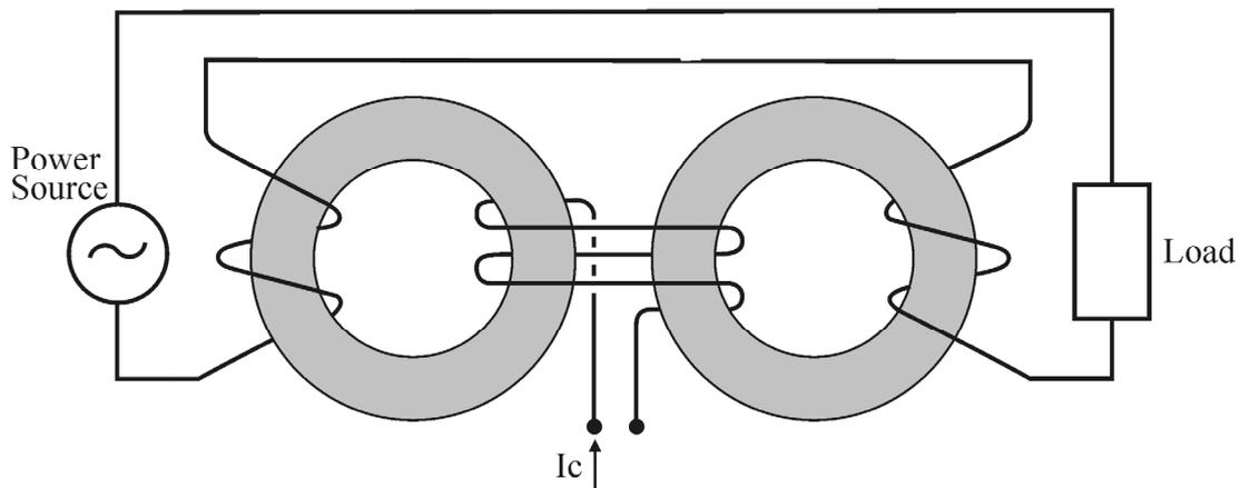
Fig. 7. Two cores with a common control winding
