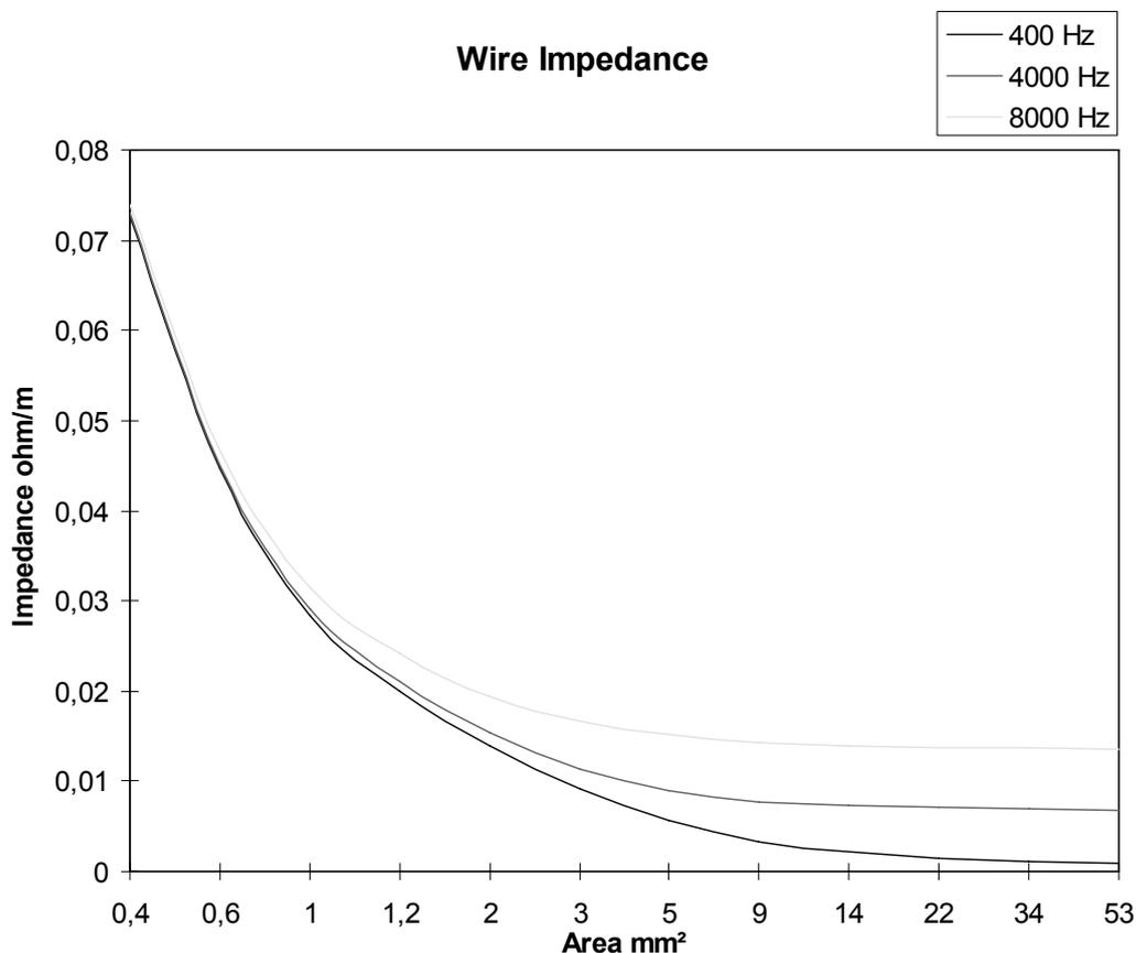
Fig. 56. Shows the absolute value of the one phase wire impedance, for a three phase system as a function of the conductor copper area for  $d/a=3$
