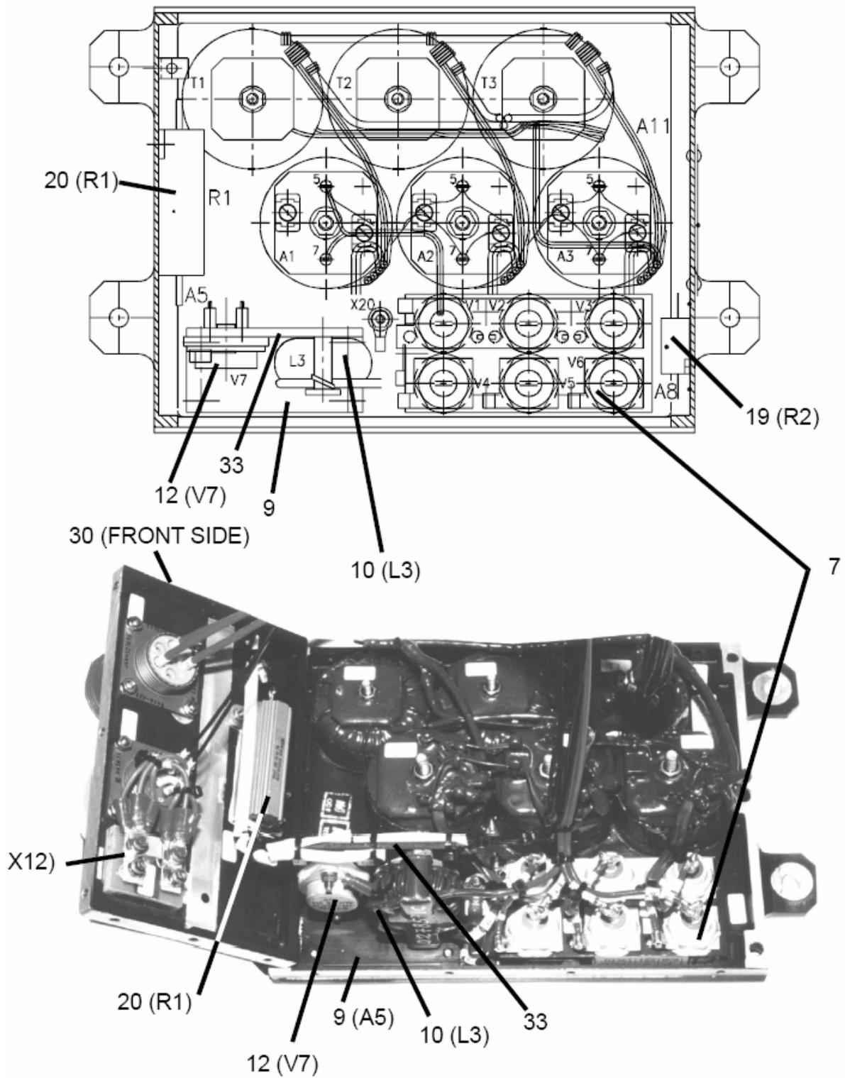
Fig. 27. The layout for three-phase magamp (photo Euroatlas)
