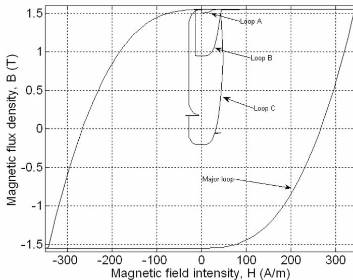
Fig. 37. Minor loop simulation at 4 kHz
