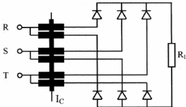
Fig. 17. The three-phase self saturating magamp
