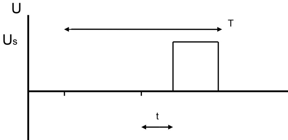
Fig. 15c. The output signal from the Ramey magamp
