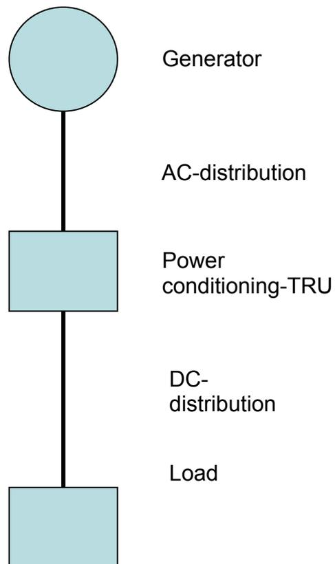
Fig. 57. Shows a simplified aircraft power supply system
