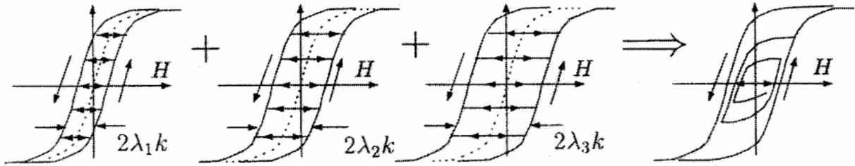
Fig. 33. Weighted superposition of the contribution from minor loops
