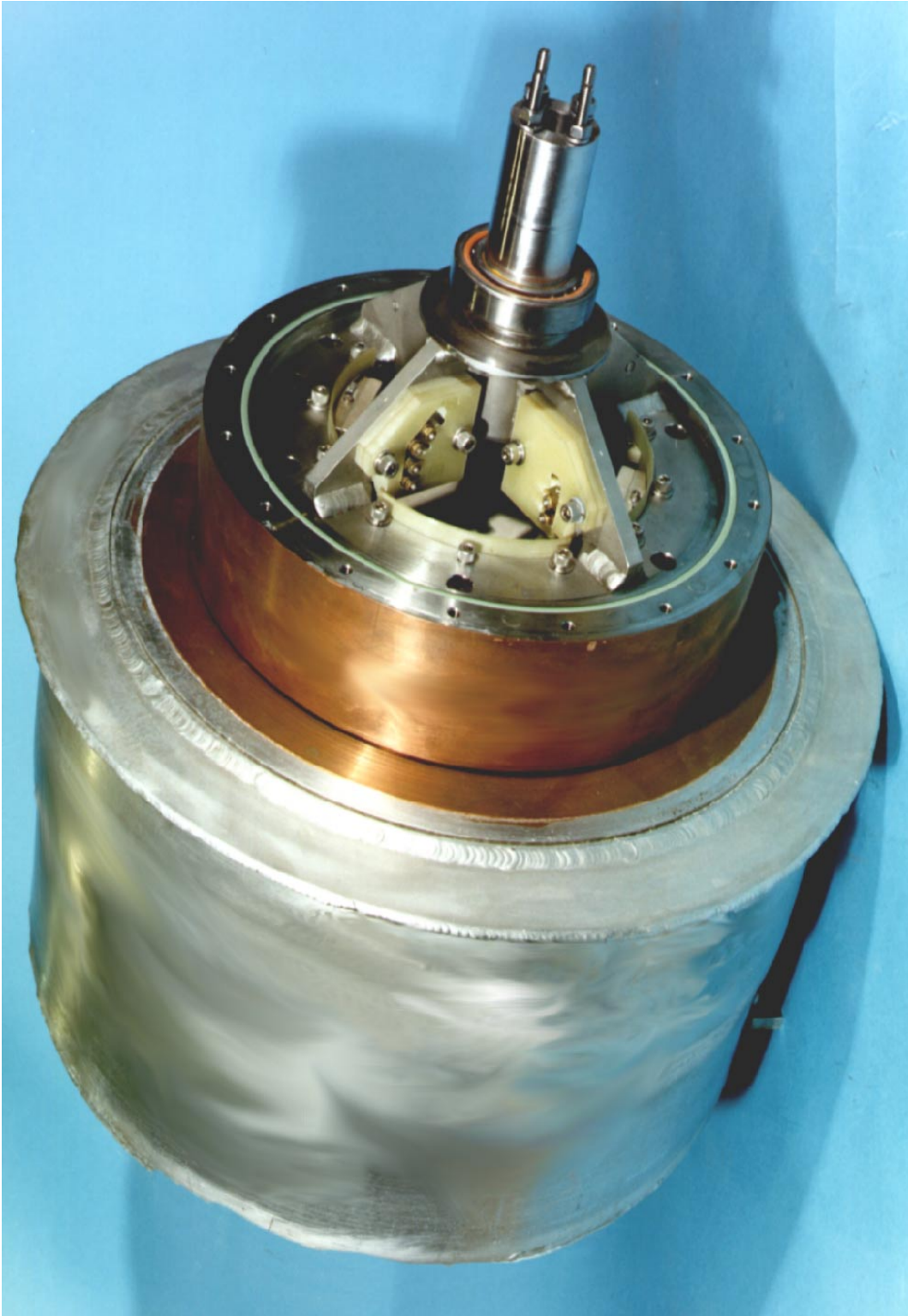
Figure 1. A 1-MW cryogenic motor successfully built and tested for aerospace applications (1991).
