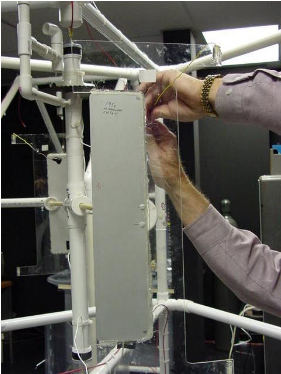
Figure 9. Closeup view of a TDT thruster on the end of the rotor arm.
