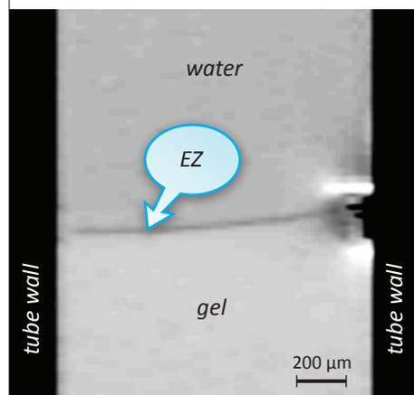
**Fig. 3.16** MRI map of relaxation times. The lower half of a capillary tube was filled with polyvinyl alcohol gel, while the upper half was filled with water. The dark band, corresponding to the gel’s EZ, indicates more molecular restriction.
