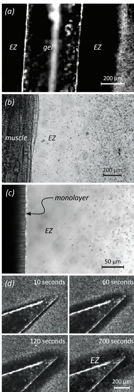
**Fig. 3.9** Examples of microsphere-excluding zones, viewed in an optical microscope. (a) polyacrylic acid gel; (b) muscle; (c) a self-assembled monolayer on gold. (d) Nafion polymer, time series.
