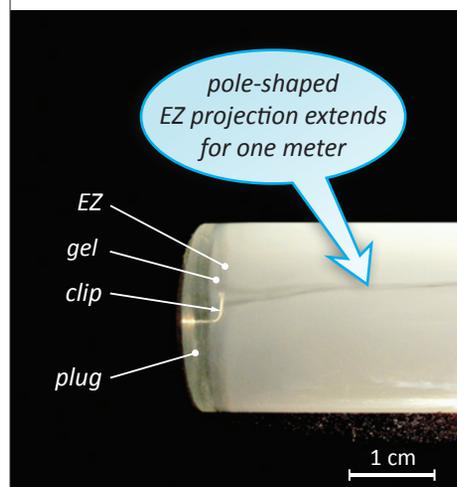
**Fig. 3.8** *Long EZ projection. The disc-like gel creates a disc-like EZ that wedges into a long pole-like projection. The projection can extend at least one meter.*
