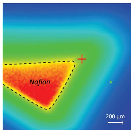
**Fig. 3.14** Triangular specimen of Nafion in water examined using infrared absorption. Color differences indicate differences of absorption. Blue is lowest.
