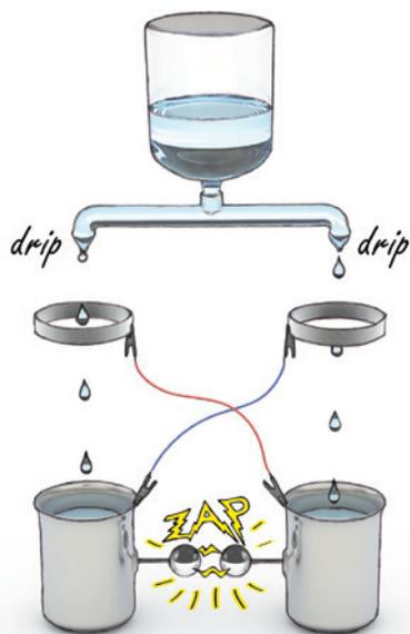
**Fig. 1.6** The Kelvin water-dropper demonstration. Rising water levels create a high-voltage discharge. Why does this happen?
