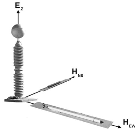
Figure 3: Schematic setup of SR receiving station: vertical antenna receives the electric field and the two buried horizontal antennas receive the north-south and east-west magnetic field components.
