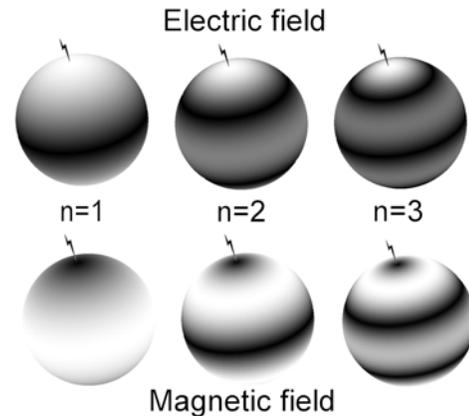
Figure 2: Electric and magnetic fields of the first three SR modes.
