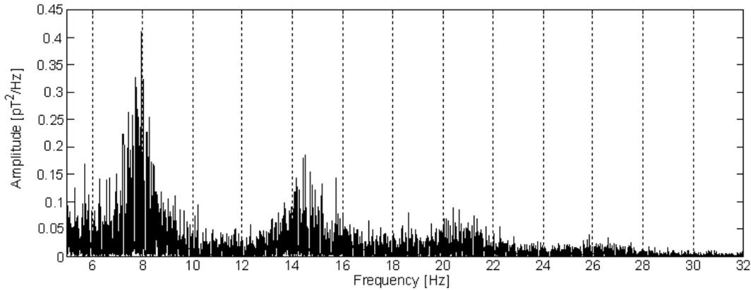
Figure 1: Schumann resonances in a sample spectrum of ELF natural electromagnetic signal (magnetic field north-south component) recorded at Mitzpe Ramon (32N, 34E) station, Israel
