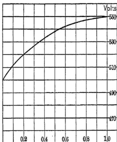
FIG. 88. Compounding Curve.
