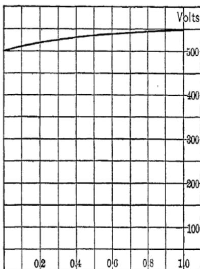
FIG. 87. Compounding Curve.
