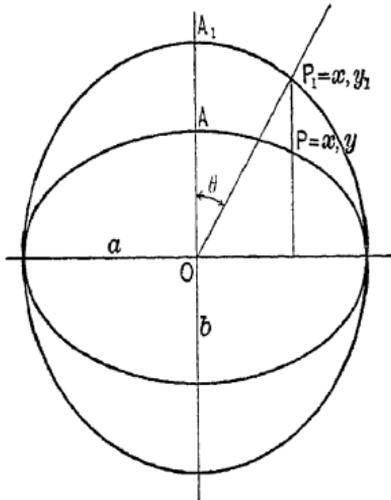
FIG. 93. Rectification of Ellipse.
