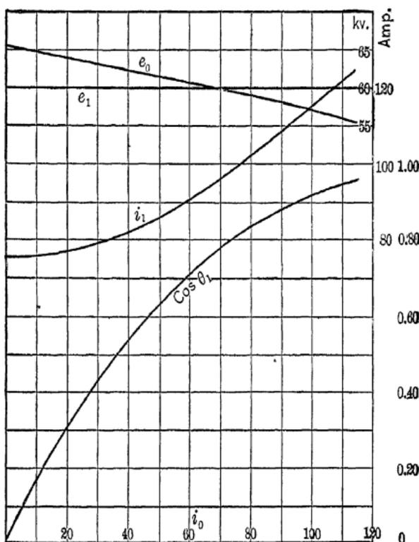
FIG. 86. Transmission Line Characteristics.
