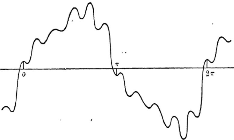
FIG. 44. Generator e.m.f. wave.
