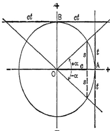
FIG. 33. Functions of Negative Angles.
