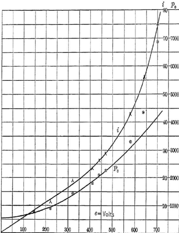
FIG. 59. Excitation Power of Induction Motor.
