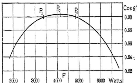
FIG. 53. Power-factor Maximum of Induction Motor.
