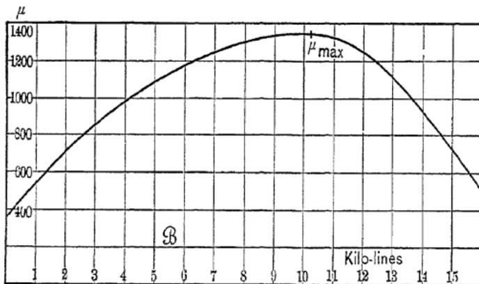
FIG. 52. Permeability Curve.
