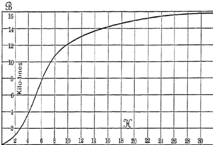
FIG. 51. Magnetization Curve.
