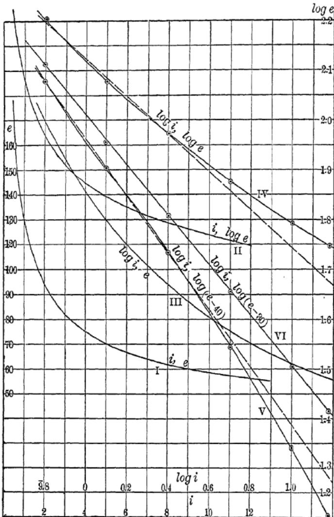
FIG. 80. Investigation of Volt-ampere Characteristic of Magnetite Arc.
