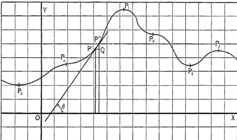
FIG. 50. Graphic Solution of Maxima and Minima.
