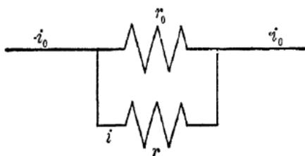
FIG. 56. Shunted Resistor.
