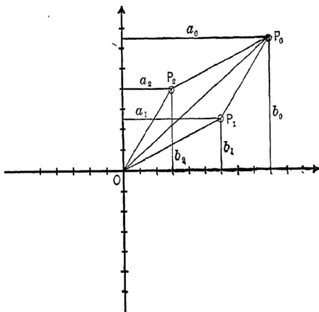
FIG. 15. Addition and Subtraction of Vectors.
