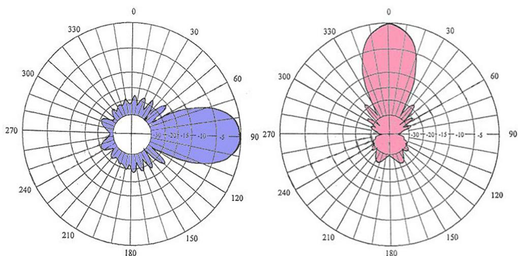
**Figure A.3.** Horizontal and vertical linear momentum radiation (Poynting vector) diagrams of the lobes of the COTS Yagi–Uda antennae used in the interferometer. The diagrams show the usual complicated pattern of the secondary lobes.
