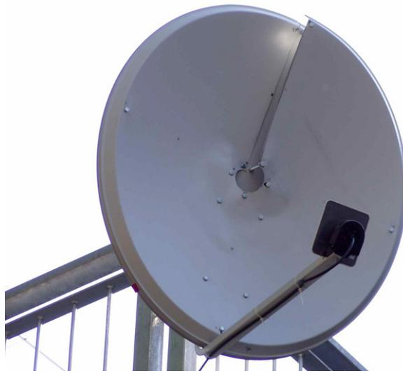
**Figure A.4.** The helicoidal parabolic antenna.
