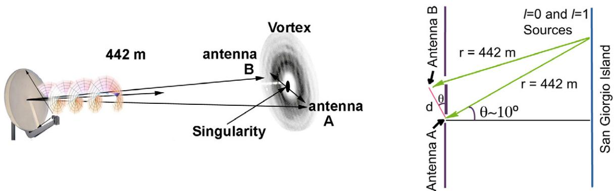
**Figure A.6.** Sketch of the experiment in San Marco (not to scale). From left to right: the transmitting antenna, the twisted radio beam and the two antennae A and B aligned with the singularity of the beam. The two receiving antennae were positioned so that the singularity was located on the baseline between the two antennae at the midpoint of the segment AB. Rightmost panel: schematic representation of the experiment.
