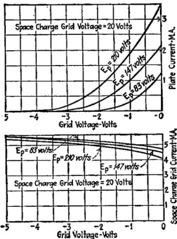
FIG. 31.—Characteristic curves of space-charge grid triode.
