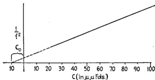
FIG. 28.—Plot of  $1/f^2$ , where  $f$  is the resonant frequency, as a function of external tuning capacity. The value of negative capacity  $C_0$  at which the extrapolated line intercepts the capacity axis is the distributed capacity of the coil, and the slope of the line is a measure of the coil inductance.
