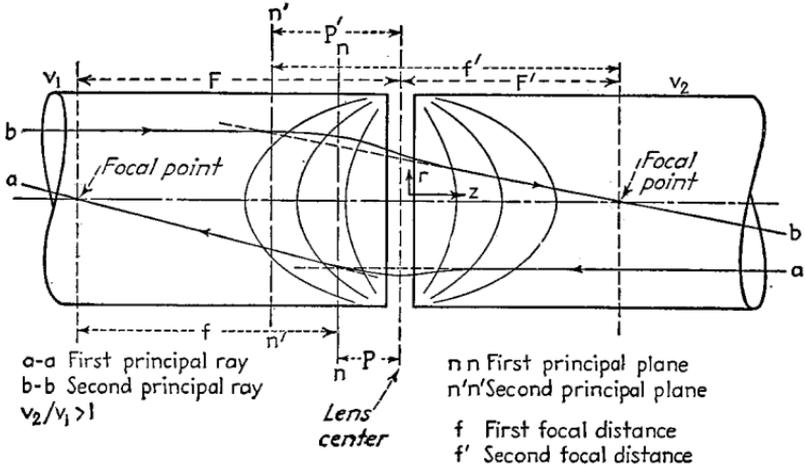
FIG. 43.—Terminology of thick electron lens.
