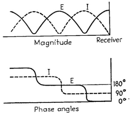
FIG. 45.—Variation of the phase of voltage and current on an open-circuited transmission line with increasing distance to the load.
