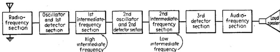
FIG. 26.—Schematic diagram of triple-detection receiver.
