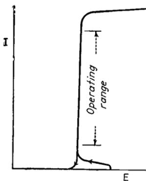
FIG. 60.—Current-voltage characteristics of a cold-cathode diode.
