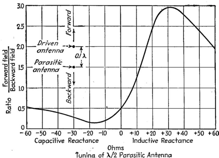
FIG. 46.—Effect of tuning of parasitic antenna on ratio of fields in forward to backward direction in a typical case.
