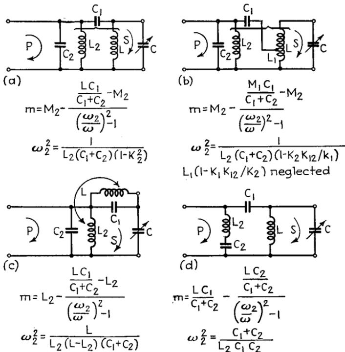
FIG. 34.—Circuits with complex coupling in which the equivalent mutual inductance varies according to a different law from that applying to Figs. 28–33.
