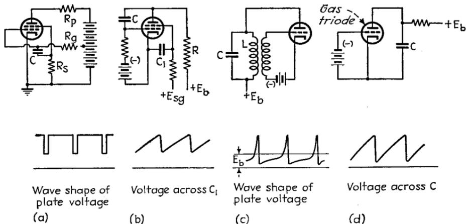
FIG. 35.—Miscellaneous types of relaxation oscillators, together with voltage wave shapes developed in circuits.
