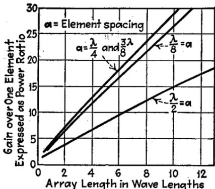
FIG. 36.—Gain of end-fire array as a function of array length for various element spacings. These curves are calculated on the assumption that the individual antennas are vertical doublets and that the array length is in a horizontal direction.
