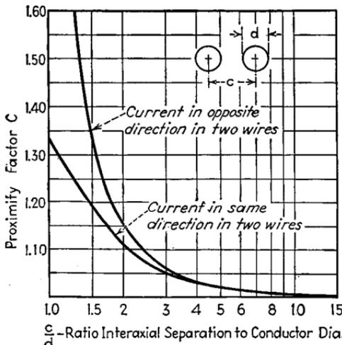
FIG. 6.—Proximity factor in parallel cylinders or tubes for very high frequencies.
