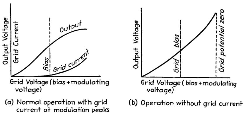
FIG. 5.—Characteristics of grid-modulated amplifiers under various conditions.
