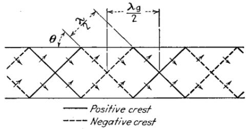
(a) Wave fronts corresponding to Fig. 119 b
