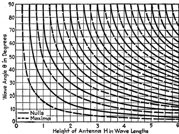
FIG. 23.—Chart showing the vertical angles at which the factor  $[2 \sin(2\pi \frac{H}{\lambda} \sin \theta)]$  is maximum and zero. These represent the vertical angles at which the reflections from the ground cause complete reinforcements and complete cancellation, respectively, of the radiation.
