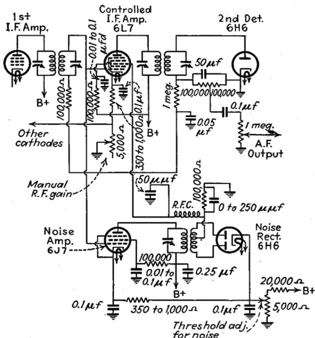
FIG. 24.—Noise-suppressor system in which a noise pulse that is stronger than the desired signal can be made to silence the receiver momentarily.
