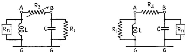
FIG. 30.—Schematic diagram of resistance-tuned oscillator.
