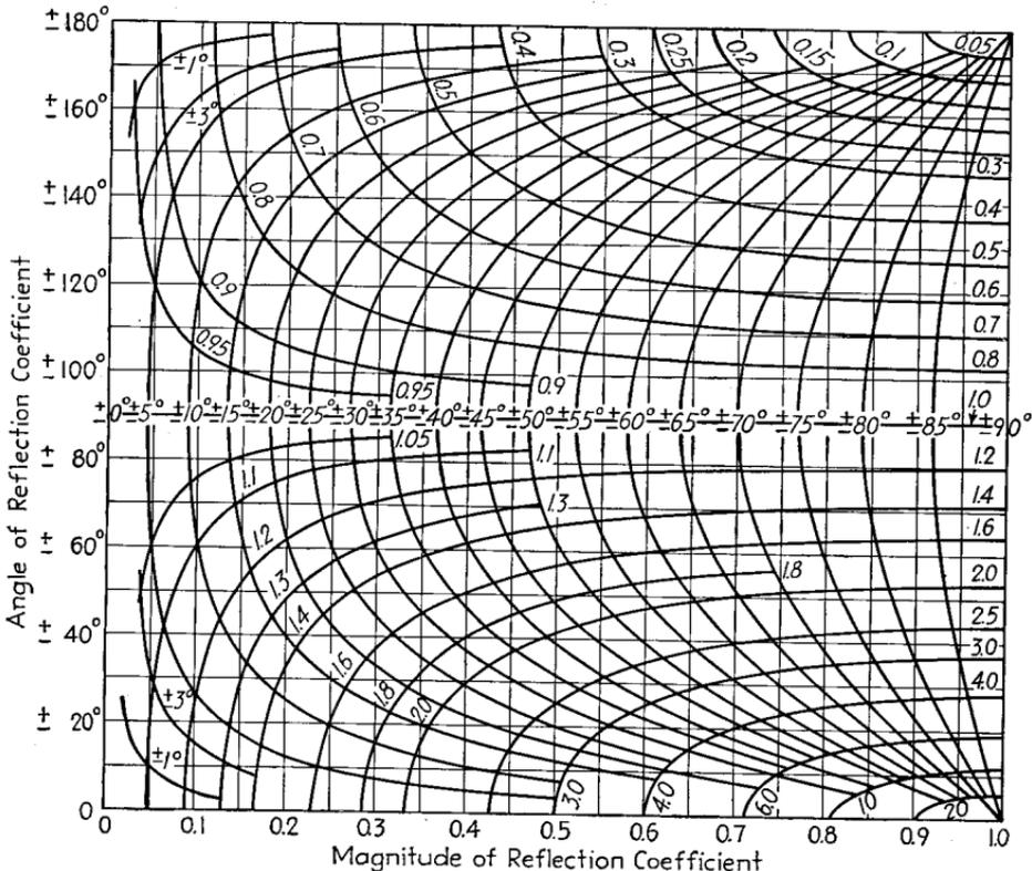
FIG. 42.—Chart giving the magnitude and phase of the reflection coefficient at the load in terms of the vector ratio  $Z_L/Z_0$  of load to characteristic impedance. The numbers on the curvilinear system of coordinates represent the magnitude and phase of the ratio  $Z_L/Z_0$ .
