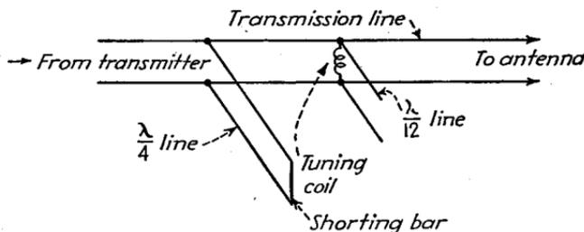
Fig. 9.—Suppression of harmonics by resonant transmission lines.
