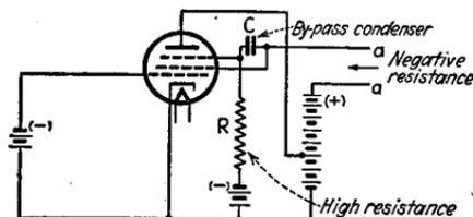
FIG. 34.—Retarding field or transitron method of producing a negative resistance.
