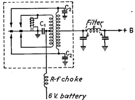
Fig. 17.—Circuit of synchronous vibrator power supply.
