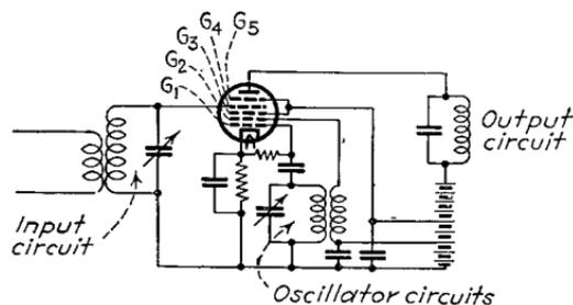
FIG. 42.—Circuit of typical pentagrid-converter tube.
