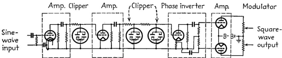
FIG. 76.—Schematic circuit diagram of square-wave generator employing clipping of a sine wave.
