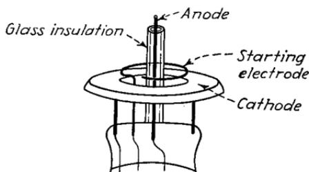
FIG. 61.—A cold-cathode discharge tube with starter electrode.
