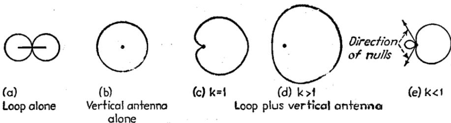
FIG. 52.—Directional patterns obtained by combining a vertical antenna with a vertical loop. The quantity  $k$  represents the contribution of the vertical antenna to the output, as compared with the loop contribution.
