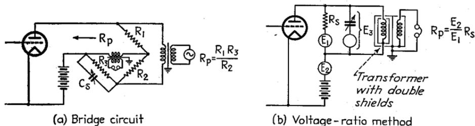
FIG. 65.—Circuits for measurement of electrode resistance.
