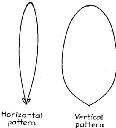
FIG. 68.—Typical field pattern of sectoral horn excited by a  $TE_{0,1}$  wave. For the case shown, the flare angle is  $30^\circ$ , the horn length  $R$  is  $11\lambda$ , and the vertical aperture is one wave length.
