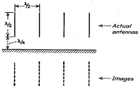
FIG. 34.—Diagram of simple broadside array illustrating notation.
