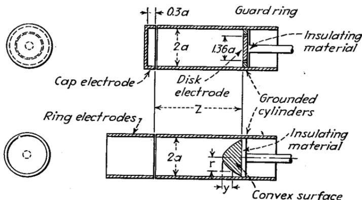
FIG. 87.—Mutual-capacity attenuator. The best shape of the convex surface is that represented by the equation  $\epsilon^{-2.4y/a} = J_0(2.4r/a)$ .
