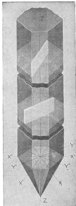
FIG. 7.—Illustration showing the natural quartz crystal and the relation of the electric or  $X$ , the mechanical or  $Y$ , and the optical or  $Z$  axes to the crystal structure. The upper section shows a  $Y$  (or  $30^\circ$ ) cut plate, while the plate in the center section is  $X$ - (or Curie-) cut. The third  $Y$  axis,  $Y''Y''$ , is not shown because the perspective of the drawing makes it coincide with the  $ZZ$  axis.
