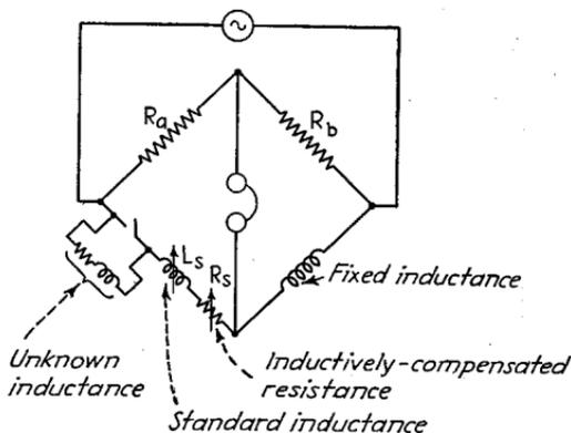
FIG. 8.—Substitution measurement of small inductances using a general-purpose bridge with a variable inductance and an inductively-compensated resistance as standards.
