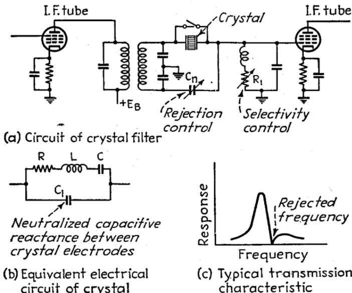
FIG. 23.—Typical crystal coupling arrangement used in single-signal receiver.
