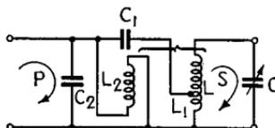
$$m = \frac{M_1 C_1}{C_1 + C_2} + \frac{M_2 + \frac{M_1 C_1}{C_1 + C_2}}{\left(\frac{\omega}{\omega_2}\right)^2 - 1}$$
