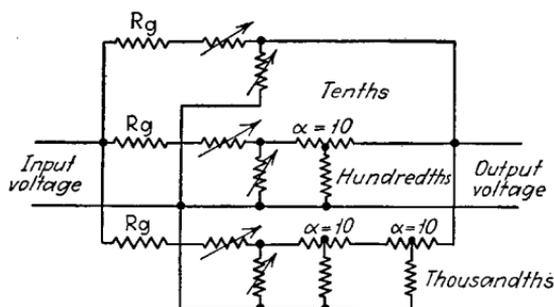
FIG. 83.—Circuit diagram of decimal attenuator.
