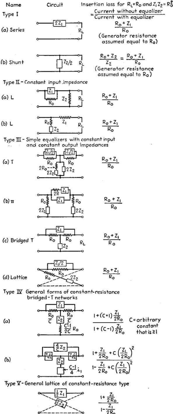
FIG. 111.—Equalizer networks and corresponding insertion loss formula.
