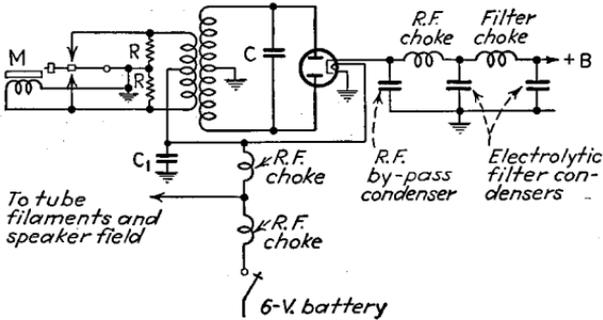
Fig. 16.—Circuit of nonsynchronous vibrator power supply.
