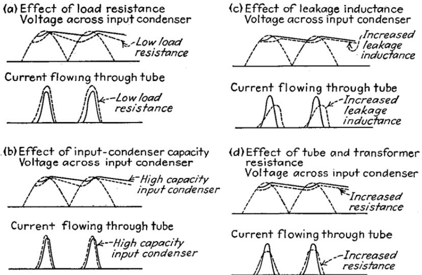
FIG. 10.—Effect of circuit parameters on behavior of rectifier operated with condenser-input filter.
