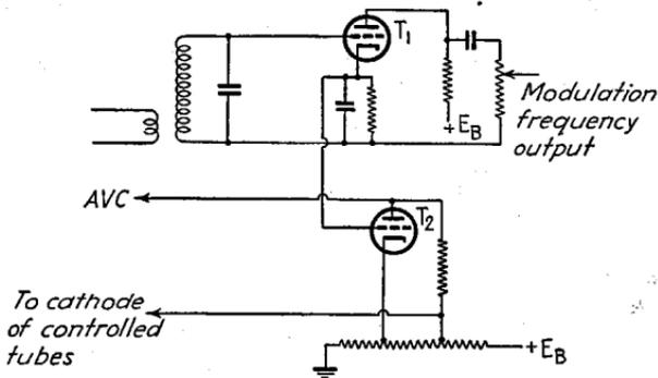
FIG. 14.—Automatic-volume-control system using plate detector.
