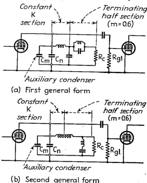
FIG. 55.—General two-terminal coupling networks based upon low-pass filters. The constant  $k$  sections are Type II sections of Table 2, Sec 3.
