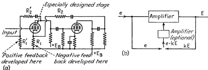
FIG. 40.—Alternative methods of obtaining behavior similar to that obtained with negative feedback.
