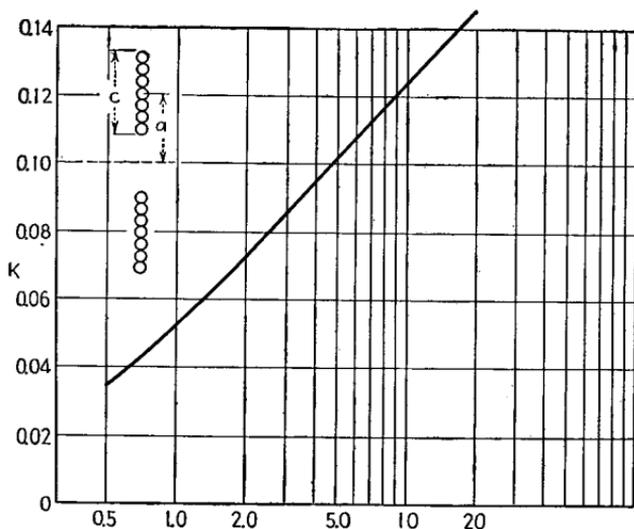
FIG. 24.—Factor  $K$  for flat spiral coil used in Eq. (45).
