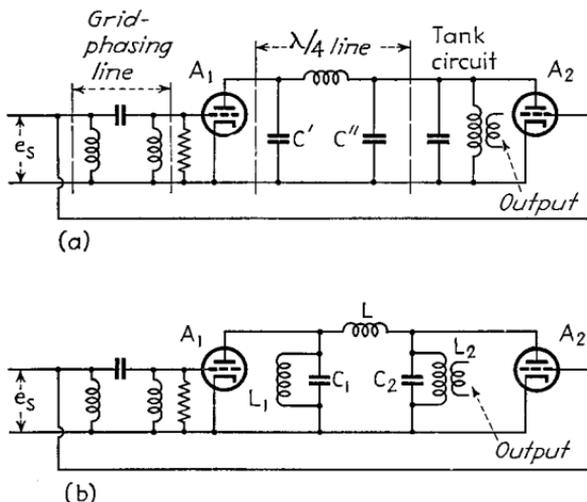
FIG. 82.—Schematic diagram of high-efficiency linear amplifier.
