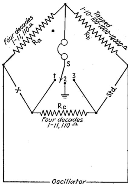
FIG. 5.—Circuit details of a typical general-purpose bridge.
