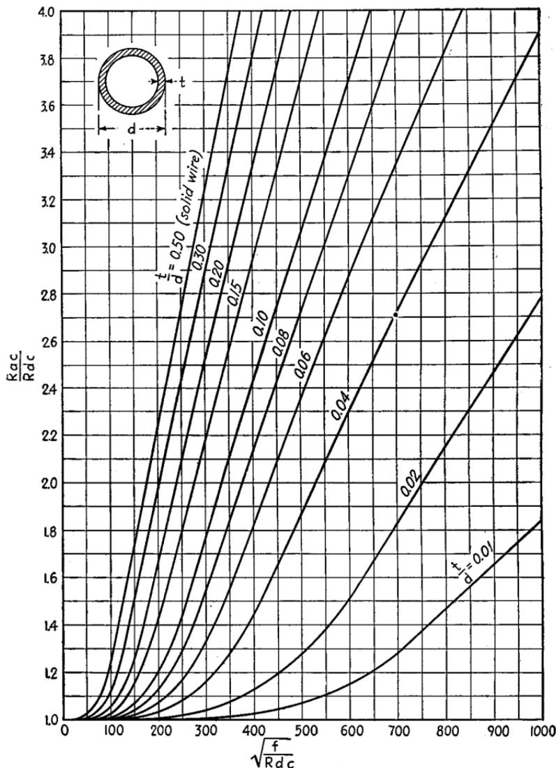
FIG. 2.—Resistance ratio of isolated nonmagnetic tubular conductors in terms of parameter  $\sqrt{f/R_{dc}}$ , where  $f$  is the frequency in cycles, and  $R_{dc}$  the direct-current resistance per thousand feet.
