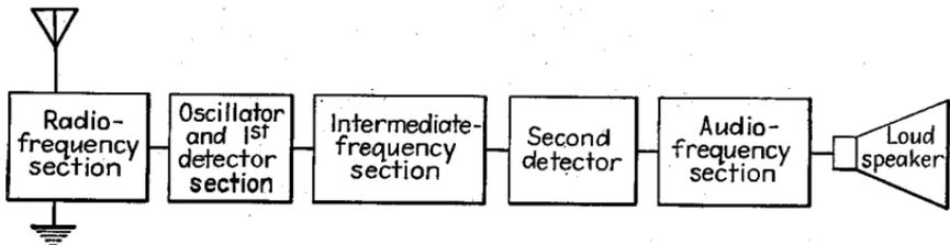
FIG. 10.—Schematic diagram of superheterodyne receiver.
