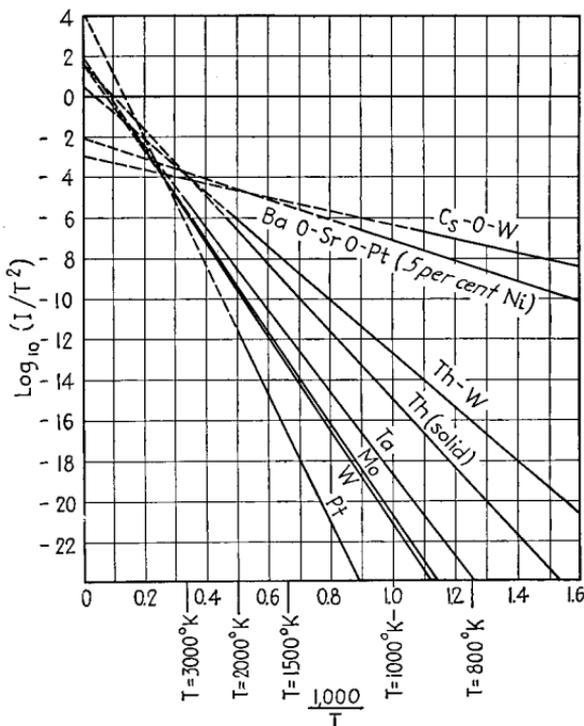
FIG. 5.—Determination of emission equation constants.
