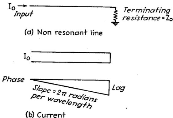
FIG. 5.—Current and phase distribution in a nonresonant antenna.
