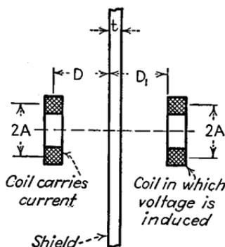
FIG. 89.—Diagram illustrating nomenclature in Eq. (152).
