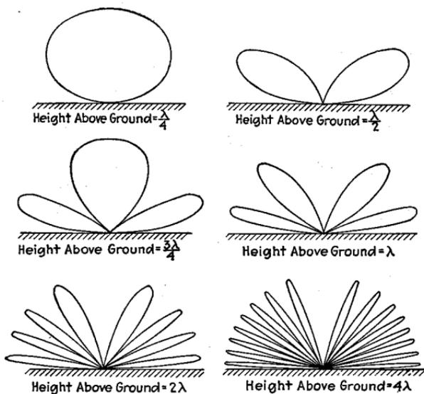
FIG. 22.—Polar diagram of the factor  $|2 \sin(2\pi \frac{H}{\lambda} \sin \theta)|$  for various values of  $H/\lambda$ , showing how the height above earth affects the directional characteristics of the antenna.
