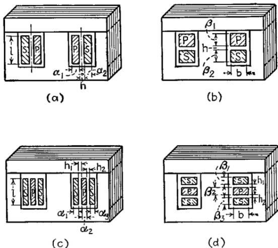
FIG. 70.—Typical coil arrangements in audio transformers.
