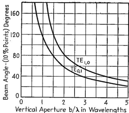
FIG. 69.—Width of beam in vertical plane for sectoral horns of various heights excited by  $TE_{0,1}$  and  $TE_{1,0}$  waves. The term beam angle is here used to indicate the angle included between the points of the major lobe, where the field intensity is 10 per cent of the maximum.
