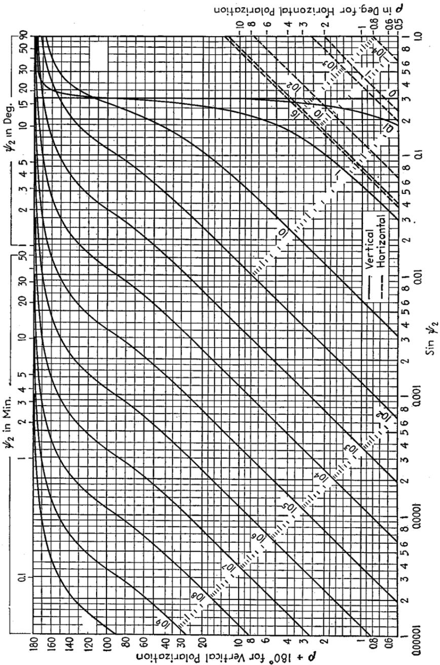
Fig. 26b.—Magnitude and phase of reflection coefficient for  $\epsilon = 10$ . The number on each curve gives the value of the quantity  $x = (\sigma_{\text{emu}}/f_{\text{mc}})18 \times 10^{14}$  to which it applies, and  $\psi_2$  is the angle of incidence (see Fig. 24).
