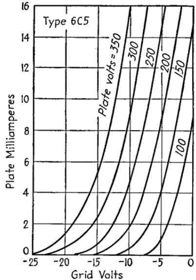
FIG. 14.—Plate-current-grid-voltage characteristics of a triode.
