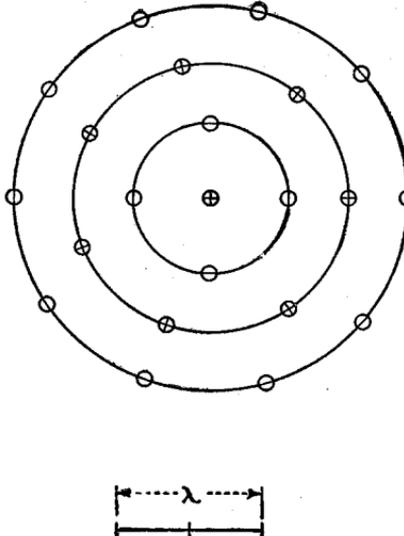
FIG. 55.—Plan view of  $J_0$  antenna array with  $m = 4$ , having a gain of 2.3. The circles represent array elements, those with a (-) inside having the current flowing  $180^\circ$  out of phase with the currents in the antennas marked (+). The radii of the successive rings are  $0.52\lambda$ ,  $0.95\lambda$  and  $1.39\lambda$ , and the relative currents in the individual antennas are 1, 0.50, 0.41, and 0.36 for the successive rings.
