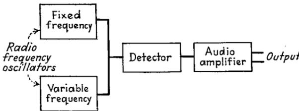
FIG. 27.—Schematic diagram of beat-frequency oscillator.
