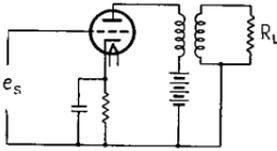
(b) Exact Equivalent Circuit of Power Tube and Transformer
