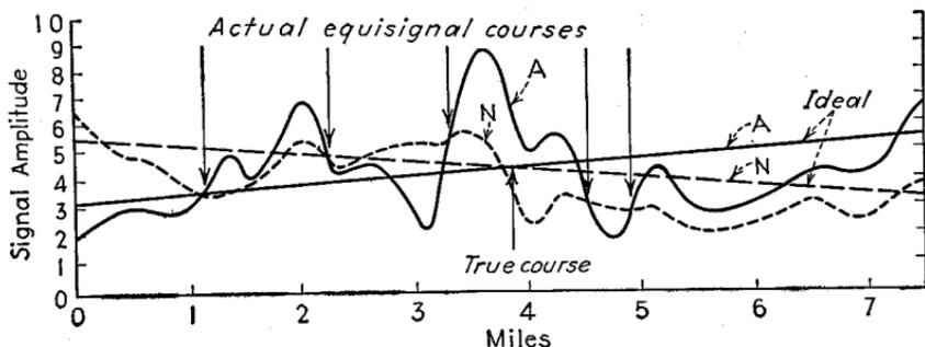
FIG. 16.—Experimentally observed field strength of A and N signals obtained by flying at right angles to the course laid down by a radio-range system under conditions where there are an excessive number of multiple courses.
