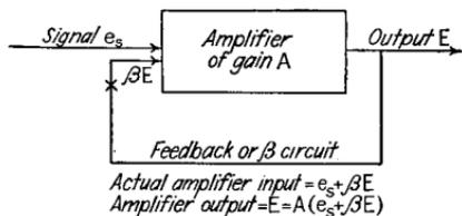
FIG. 31.—Schematic diagram of feedback amplifier.
