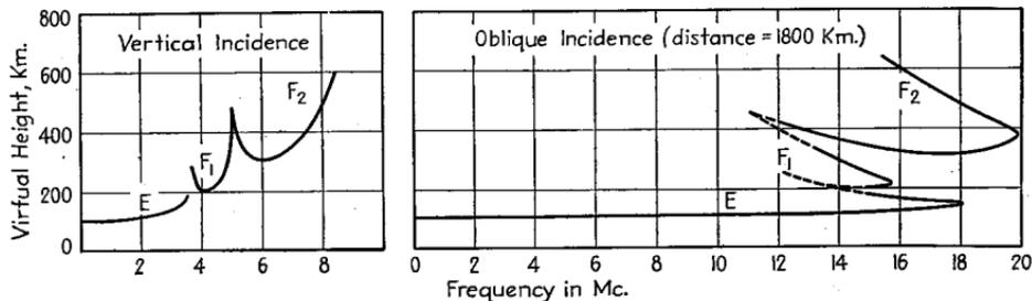
FIG. 62.—Curve of virtual height as a function of frequency for oblique incidence, together with corresponding curve for vertical incidence.
