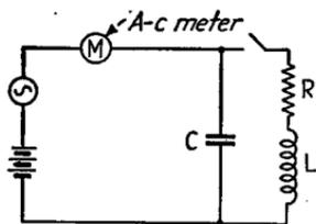
FIG. 12.—Constant-impedance method of measuring large inductances.
