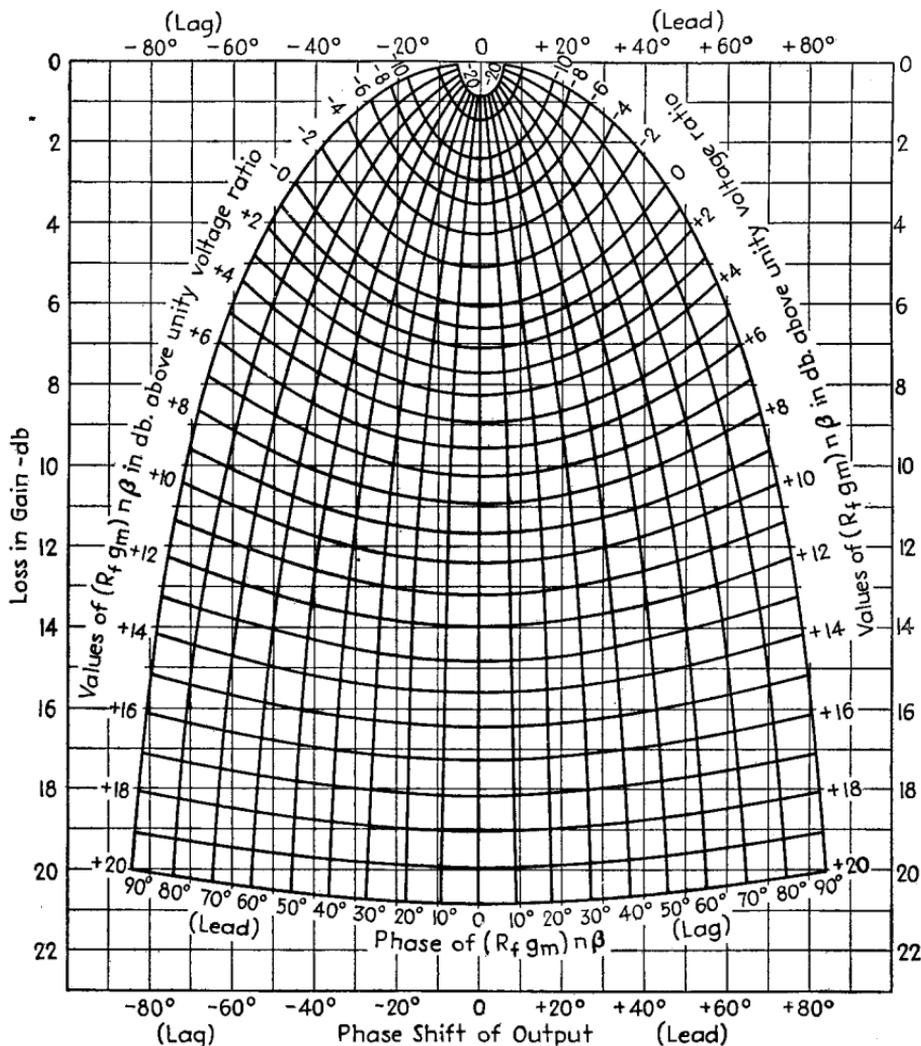
FIG. 8.—Curves from which the loss in gain and phase shift of output at low frequencies resulting from resistance-condenser bias impedance  $R_f C_f$  can be calculated in a resistance-coupled amplifier for the general case where both screen and bias impedances are of importance.
