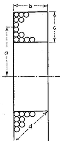
FIG. 27.—Short multiple-layer coil of solenoidal form.
