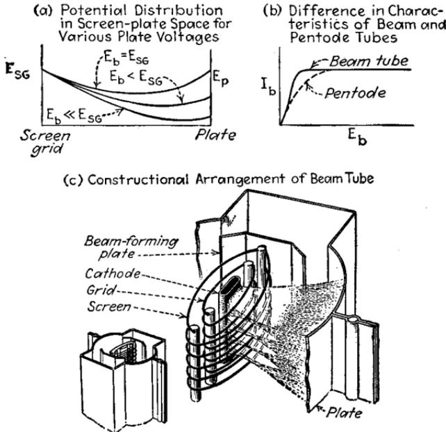
FIG. 20.—Characteristics and constructional features of the beam power tube.
