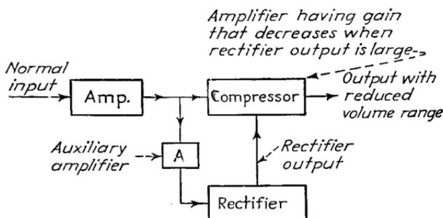
FIG. 46.—Schematic diagram of a volume compressor.
