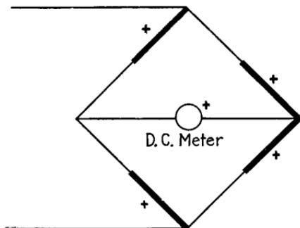
FIG. 34.—Circuit of bridge-type thermocouple instrument.
