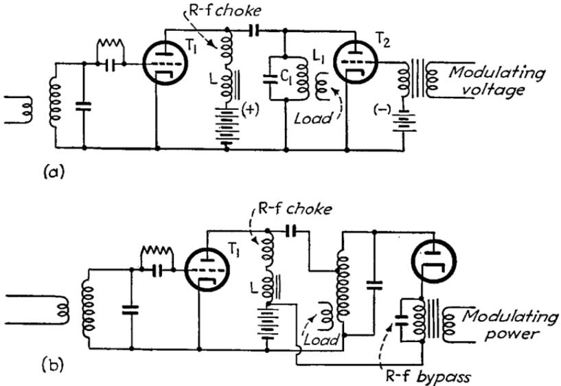
FIG. 12.—Circuits for loss modulation using constant-current choke.
