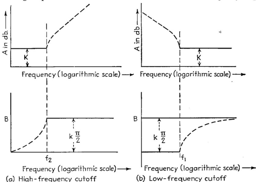
FIG. 87.—Ideal low-frequency and high-frequency cutoff characteristics.
