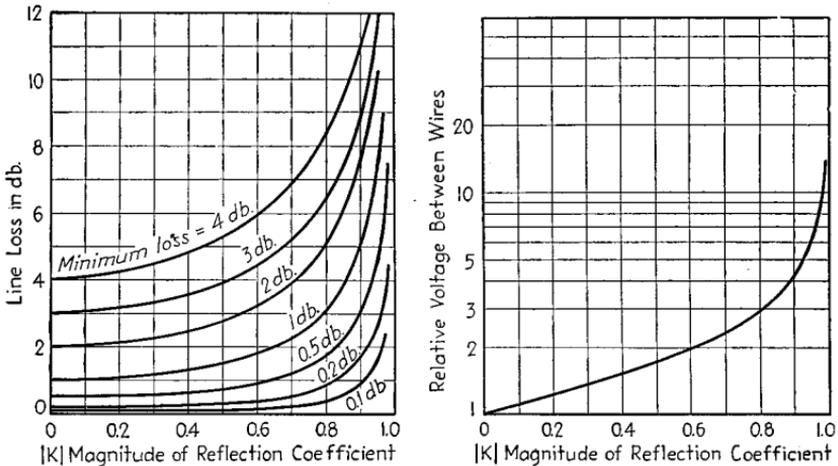
FIG. 48.—Effect of resonance on transmission line loss, and on maximum voltage between wires. The minimum loss is the loss for  $k = 0$ .
