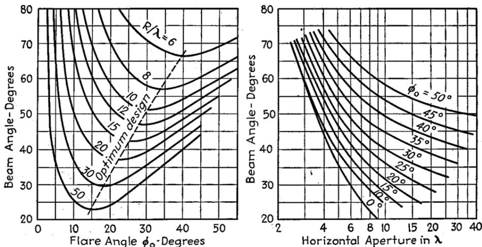
FIG. 70.—Beam angle in horizontal plane for sectoral horn of Fig. 64, excited by  $TE_{0,1}$  wave, as a function of flare angle  $\phi_0$  and horizontal aperture, for various horn lengths  $R$ . The beam angle is here defined as the angle between points at which the field strength has dropped to 10 per cent of that at the maximum of the beam. The dotted curve marked "optimum design" gives the proportions for which a beam of given width is obtained with a horn of minimum length.
