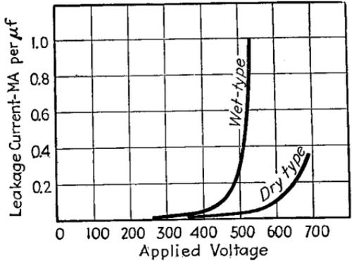
FIG. 84.—Leakage current in typical electrolytic condensers.
