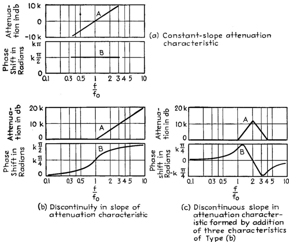
FIG. 86.—Examples of the relationship between phase and attenuation characteristic in several idealized examples.
