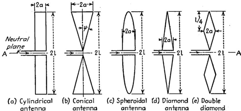
FIG. 100.—Typical wide-band antenna arrangement. All the antennas shown can be considered cross sections of a figure of revolutions. Dash line  $AA$  represents a neutral plane that can be replaced by a conductor (earth) with the omission of the lower half of the radiating system.
