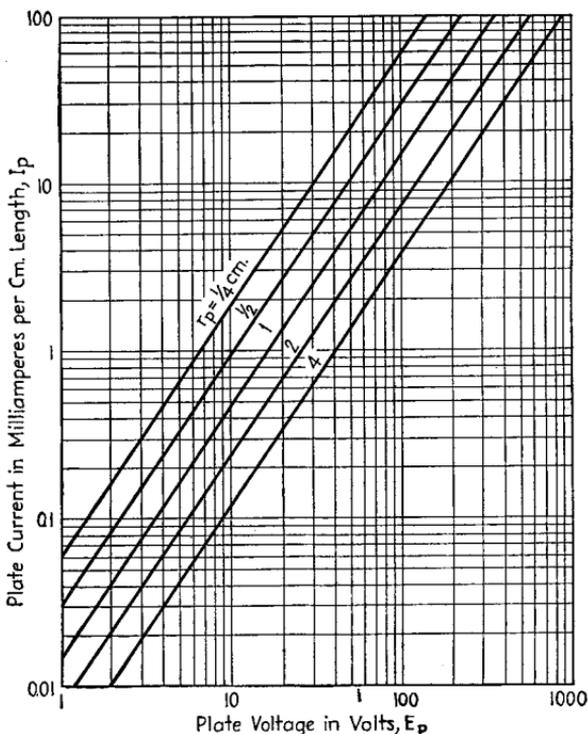
FIG. 11.—Space-charge limited current in a cylindrical electrode diode,  $\beta^2 = 1$ .
