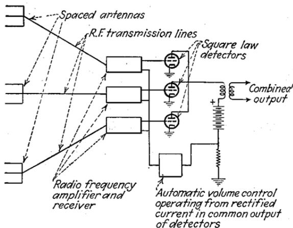
FIG. 28.—Schematic diagram of diversity telephone receiving system.
