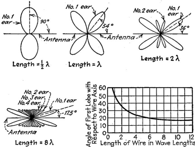
FIG. 19.—Polar diagram showing strength of field radiated in various directions from an antenna consisting of a wire remote from the ground. These diagrams can be considered as cross sections of a figure of revolution in which the axis is the antenna.
