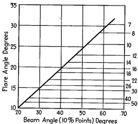
FIG. 72.—Optimum proportions for sectoral horns excited by  $TE_{1,0}$  wave, corresponding to the shortest horn giving the indicated beam width. The beam angle in this curve corresponds to the angle between points at which the field strength of the main lobe is 10 per cent of the maximum.
