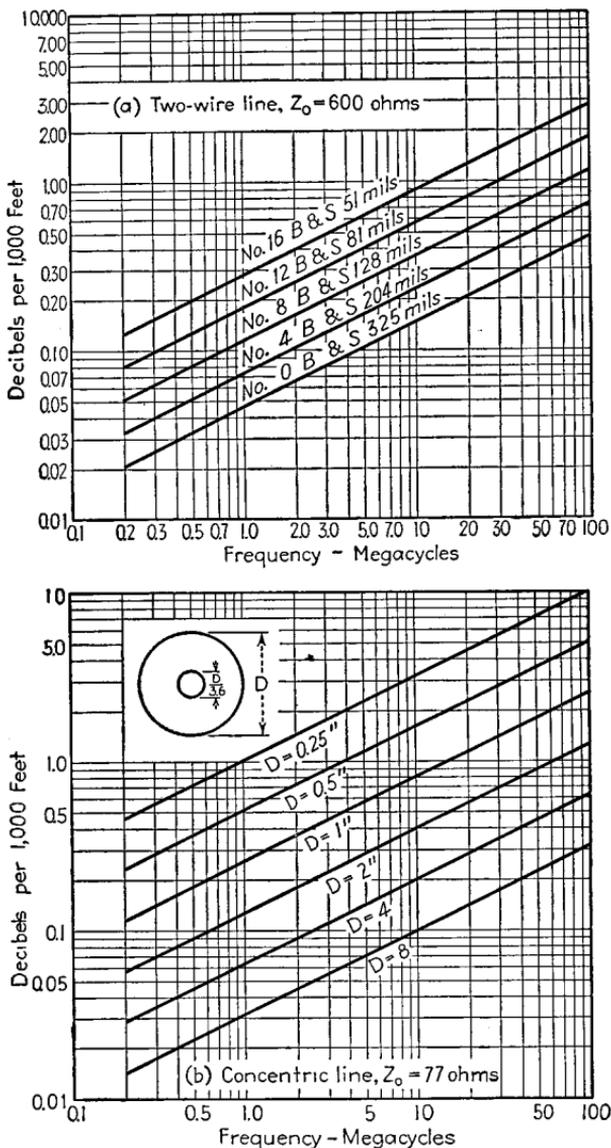
FIG. 40.—Attenuation of two-wire and concentric transmission lines.
