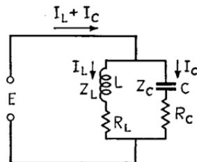
FIG. 5.—Parallel resonant circuit.
