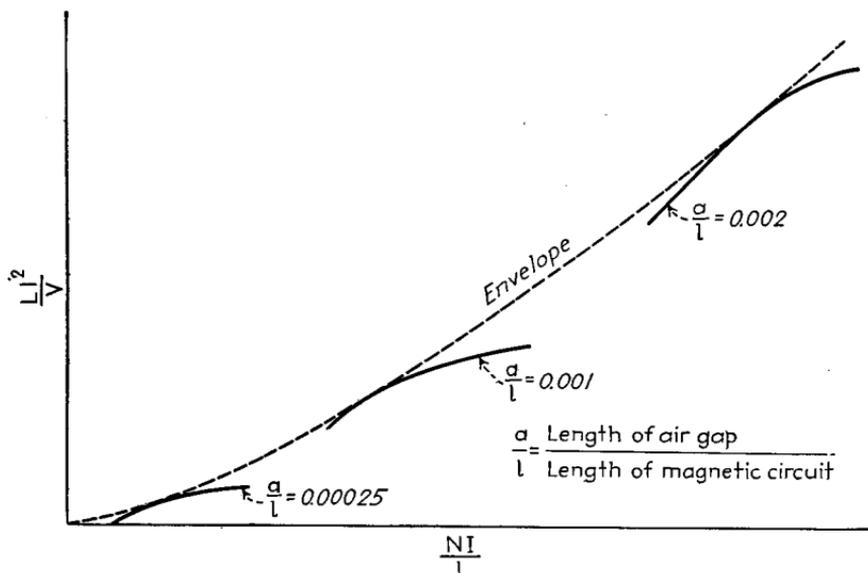
FIG. 73.—Graphical method of determining best air-gap length.
