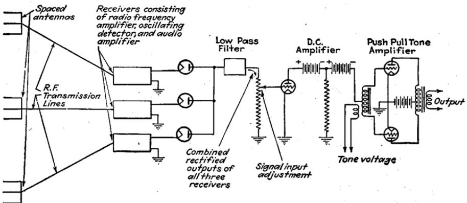
FIG. 27.—Diagram showing circuit of typical diversity receiving system for telegraph signals.
