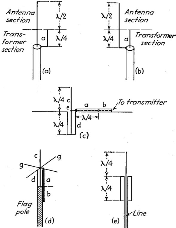
FIG. 97.—Antenna arrangements of the "flagpole" type.
