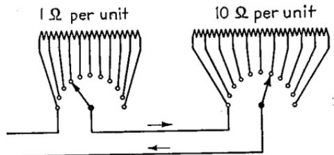
FIG. 12.—Circuit arrangement of decade resistance box.
