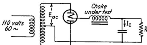
FIG. 16.—Circuit for approximate measurement of incremental inductance at high alternating flux densities.
