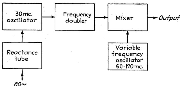
FIG. 92.—Schematic circuit arrangement of test oscillator producing a frequency-modulated wave that can be adjusted to have a carrier frequency up to 60 mc.
