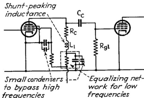
FIG. 62.—Video-amplifier circuit showing combination of high-frequency and low-frequency equalization.
