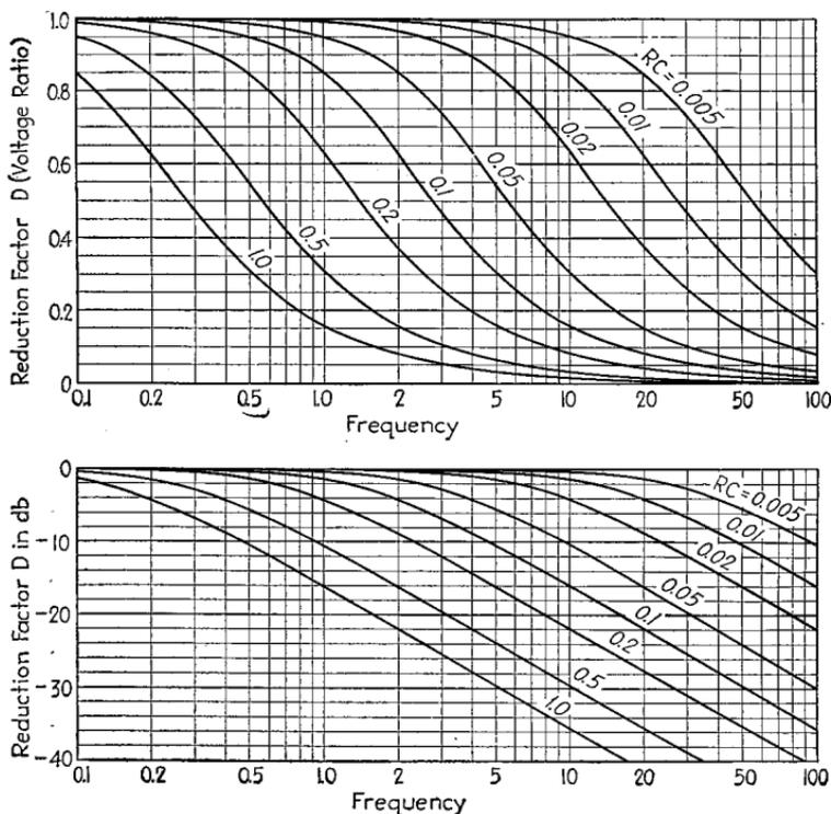
FIG. 43.—Curves giving the reduction  $D$  produced by resistance-capacity filter on the assumption that the impedance on the source side is small compared with  $R_1$ , and that the impedance on the load side is large compared with  $1/\omega C_1$ .
