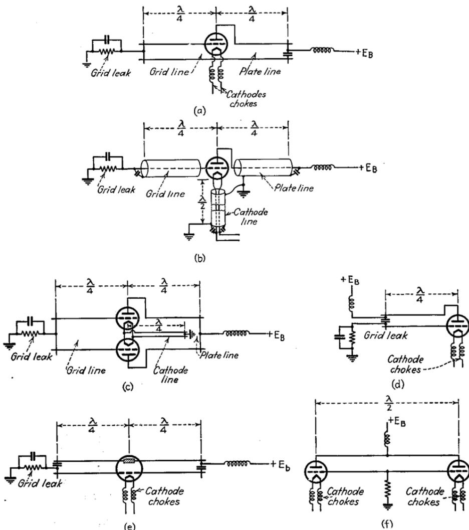
FIG. 37.—Typical circuit arrangement for ultra-high-frequency oscillators.
