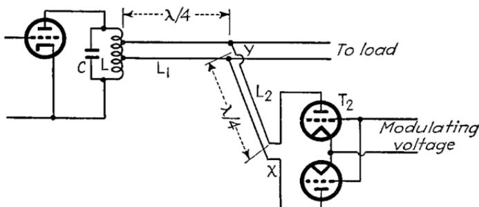
FIG. 13.—Schematic circuit for load-impedance modulation.
