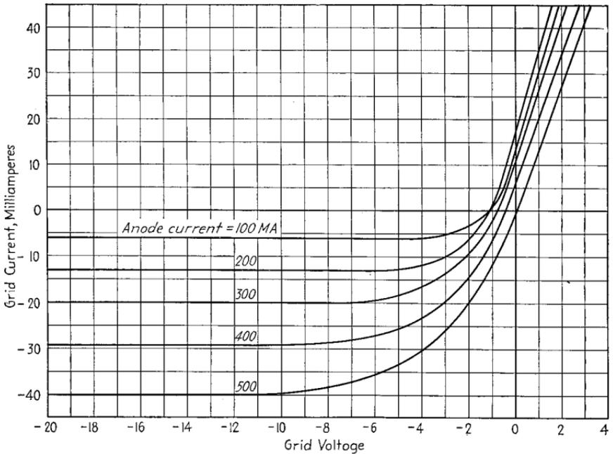
FIG. 57.—Grid-current characteristics of a typical thyatron.
