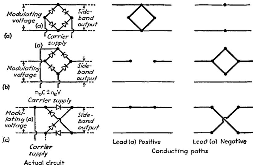
FIG. 24.—Typical copper oxide modulator circuits.
