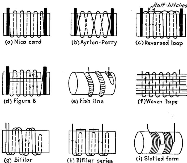
Fig. 10.—Types of resistor windings that minimize reactive effects.
