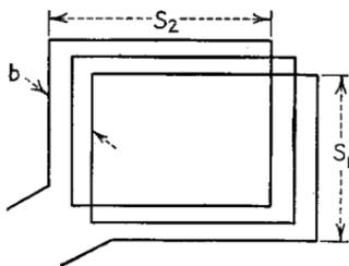
FIG. 20.—Single-layer rectangular coil.
