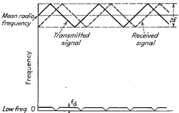
FIG. 20.—Frequency relations in absolute altimeter.
