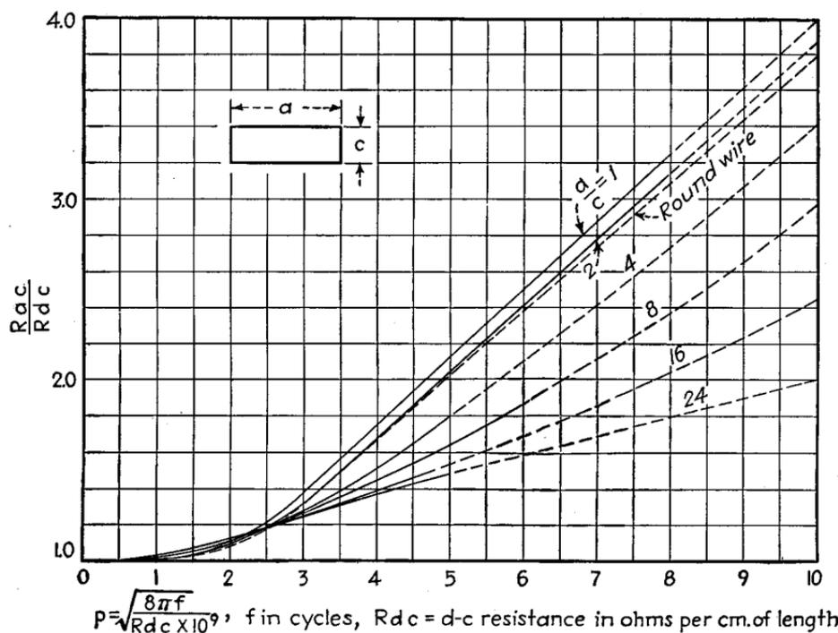
FIG. 3.—Resistance ratio of rectangular conductors in terms of parameter  $p$ , involving the frequency  $f$  in cycles, and  $R_{dc}$  the resistance in ohms per centimeter of length. These curves are a combination of experimental and calculated results, with the dotted portions representing low-frequency results extrapolated to join on with the theoretical results for high frequencies.
