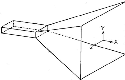
FIG. 74.—A pyramidal horn.
