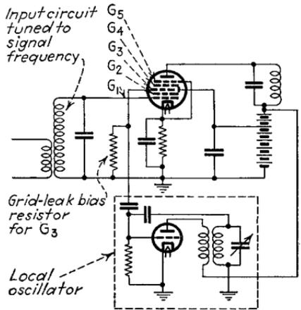
FIG. 41.—Circuit of typical pentagrid-mixer tube.
