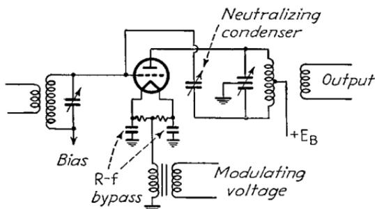
FIG. 11.—A schematic circuit of cathode-modulated amplifier.
