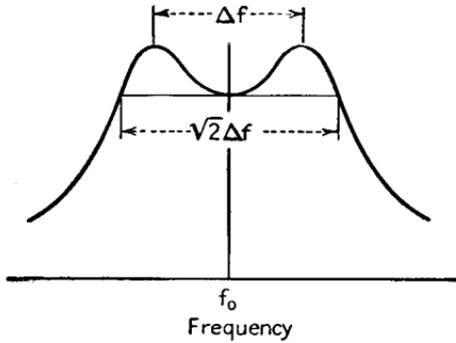
In practical work, one is commonly interested in the frequency band over which the response in the secondary circuit equals or exceeds the response at resonance. This band is illustrated schematically in Fig. 20, and can be shown to be equal to  $\sqrt{2}$  times the width of the frequency band between coupling peaks.<sup>1</sup>
