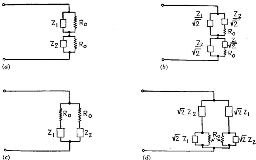
FIG. 116.—Constant-resistance types of dividing network.
