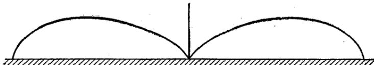
FIG. 56.—Field produced in a vertical plane by a single-ring antenna for  $n = 5$ , corresponding to a gain of 2.1.
