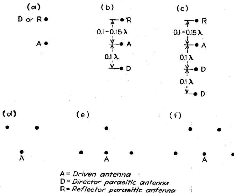
FIG. 47.—Examples of antenna arrays involving parasitic antennas.
