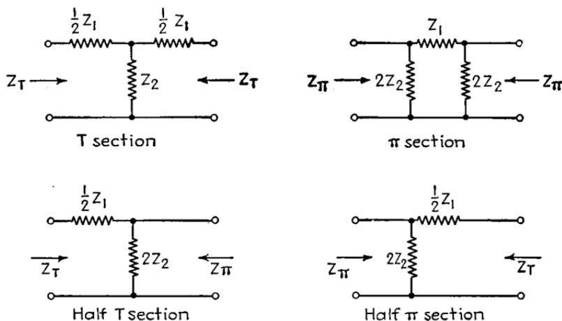
FIG. 94.—Filter sections, showing nomenclature.
