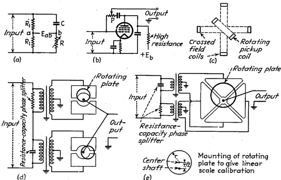
FIG. 56.—Phase-shifting devices.
