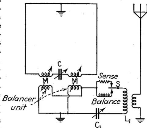
FIG. 6.—Antenna and input circuits of a practical loop direction finder provided with sense determination.
