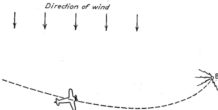
FIG. 12.—Course followed by an airplane homing on a transmitter located at B when there is a strong cross wind. Note that the course followed deviates greatly from the most direct path even though the airplane is always pointing toward B.
