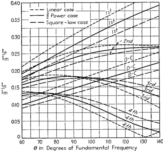
Fig. 86—Curves giving relation of direct-current and harmonic components of the space-current pulse as a function of angle of flow  $\theta$  and the peak amplitude  $I_m$ .
