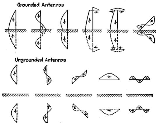
FIG. 7.—Images for common types of antennas.
