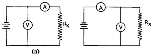
FIG. 1.—Circuit arrangements for measuring resistance by the voltmeter-ammeter method.
