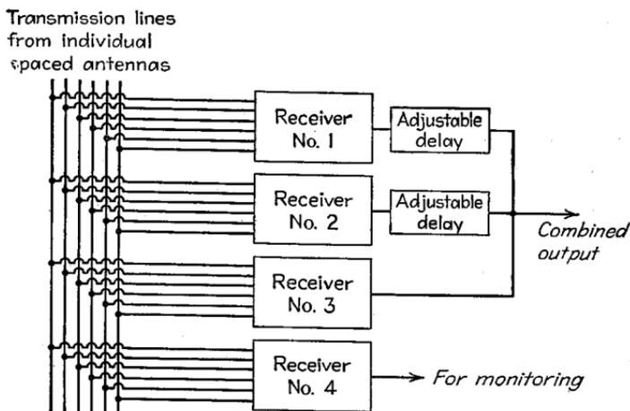
Note: Each receiver includes means for combining the output of the various antennas in the phase relations required for the desired vertical directivity
