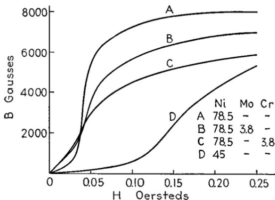
Fig. 65.—Typical magnetization curves of various nickel-iron alloys.
