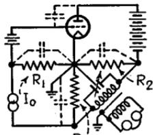
Capacity balance for capacity currents
