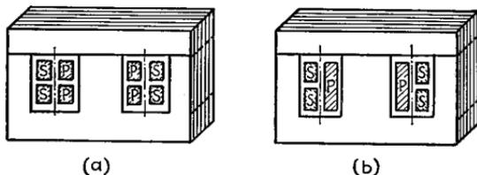
Fig. 71.—Transformers with divided windings.
