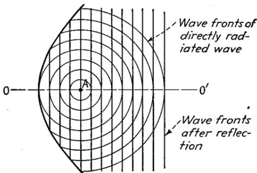
FIG. 80.—Conversion of spherical waves to plane waves by a parabolic reflector. The circles represent the spherical waves radiated from the antenna *A*; while the vertical lines represent the wave front after reflection from the parabolic surface.
