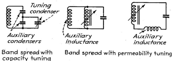
FIG. 17.—Circuit arrangements for obtaining band spread with the regular tuning adjustment.
