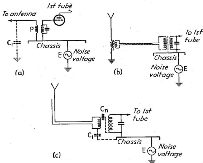
FIG. 99.—Systems for preventing a noise voltage  $E$  existing between chassis and ground, as a result of the power-cord connection, from causing a noise voltage from being applied to the grid of the first tube of the radio receiver.
