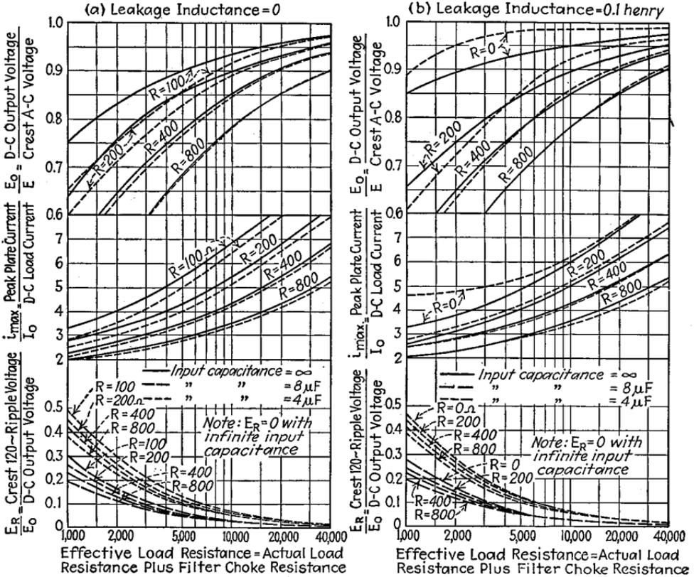
FIG. 9.—Charts giving performance of shunt-condenser filter system for 60-cycle supply source and full-wave rectifier.
