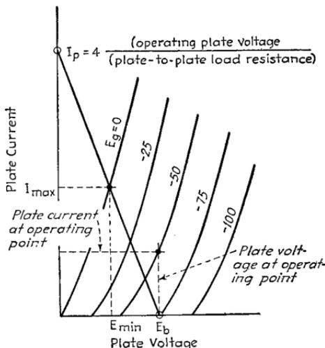
FIG. 23.—Upper half of load line for push-pull amplifier where the minimum plate current of the individual tube reaches zero. This corresponds to the part of the load line above the horizontal axis in Fig. 22.
