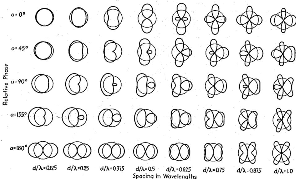
FIG. 38.—Horizontal radiation patterns of arrays of two vertical antennas fed with currents of equal magnitude, showing effect of spacing  $d$  and phase  $a$ . The circle superimposed on each diagram has the same area as the field pattern actually attained.
