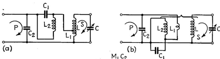
$$m = \frac{M_1 C_1}{C_1 + C_2} + \frac{M_2 - \frac{M_1 C_2}{C_1 + C_2}}{\left(\frac{\omega}{\omega_2}\right)^2 - 1}$$
