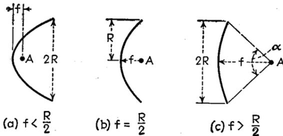
FIG. 82.—Rotational parabolas with same mouth diameter but different focal lengths.
