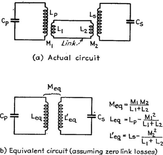
FIG. 24.—Actual and equivalent circuits for link coupling.
