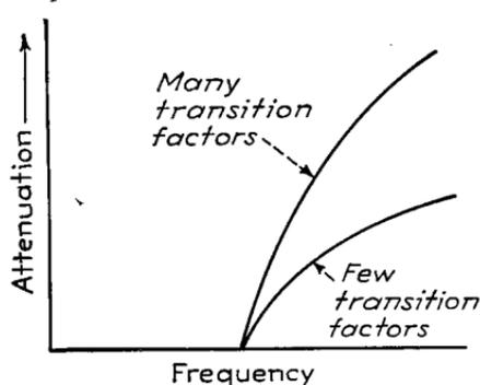
FIG. 107.—Attenuation characteristics of Bode-type lattice filter.
