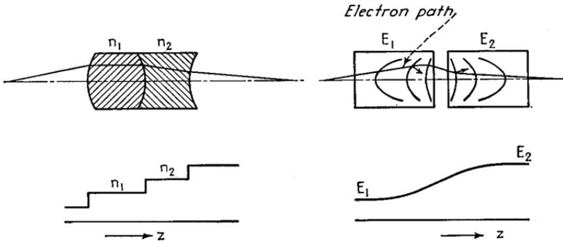
FIG. 42.—Equal-diameter cylinder lens and physical equivalent.
