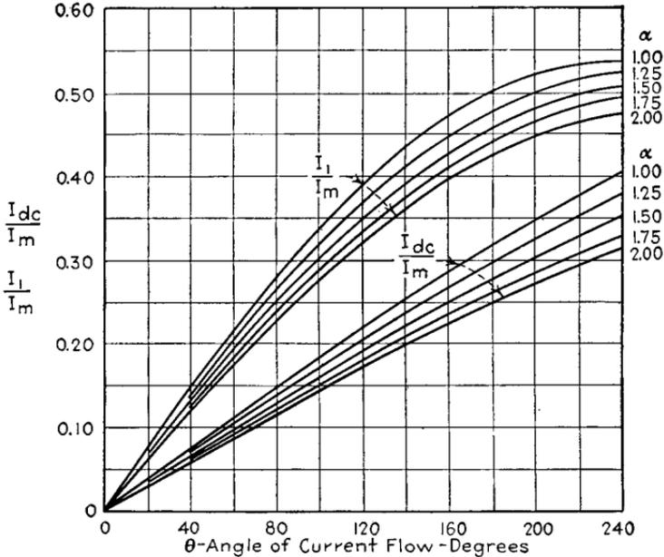
FIG. 77.—Curves giving relation of direct-current and fundamental-frequency components of the space-current pulse as a function of angle of flow  $\theta$  and the peak amplitude  $I_m$ .
