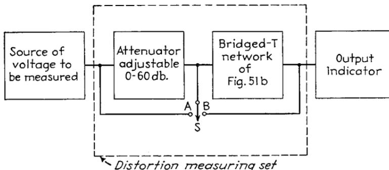
FIG. 52.—A practical distortion meter based on the network of Fig. 51b.
