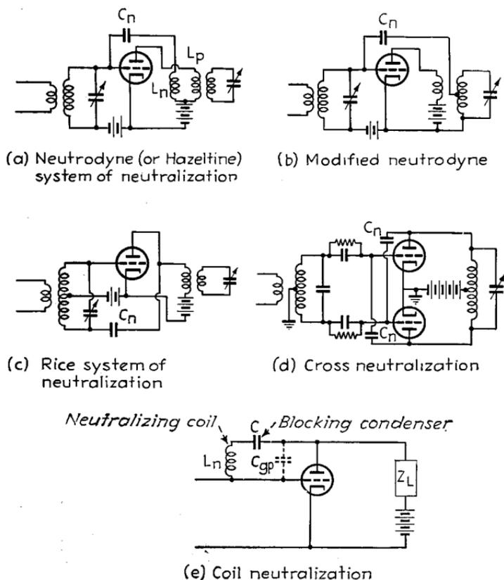
FIG. 91.—Typical neutralizing circuits.
