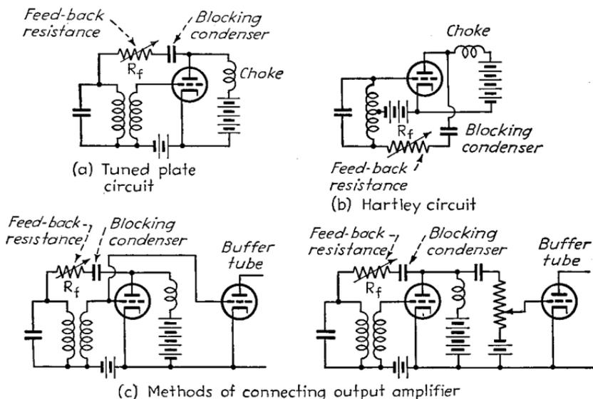
FIG. 22.—Typical laboratory oscillators with resistance stabilization.
