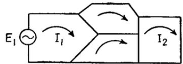
FIG. 62.—Network for illustrating meanings of driving point and transfer impedances.
