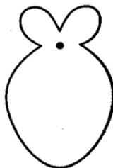
FIG. 48.—Field distribution in horizontal plane obtained from an array of vertical antennas, one of which is driven and three of which are parasitic, arranged as shown.
