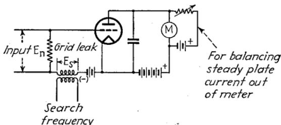
Fig. 54.—Vacuum-tube voltmeter method of analyzing wave forms.
