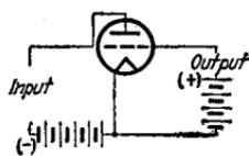
FIG. 33.—Circuit of inverted tube.
