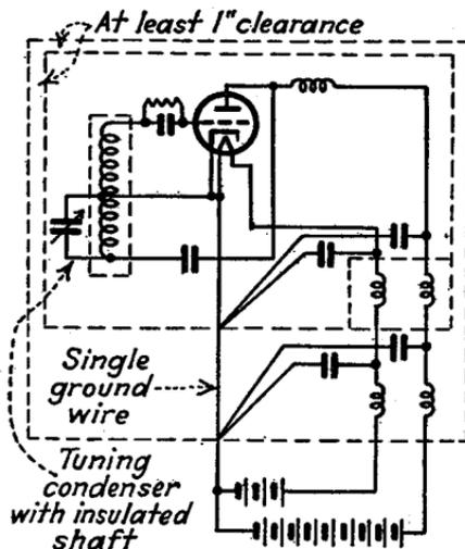
FIG. 83.—An oscillator provided with complete shielding, such as might be used in a signal generator.
