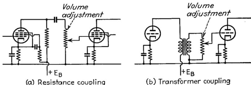
FIG. 44.—Common methods of controlling volume in resistance- and transformer-coupled amplifiers.
