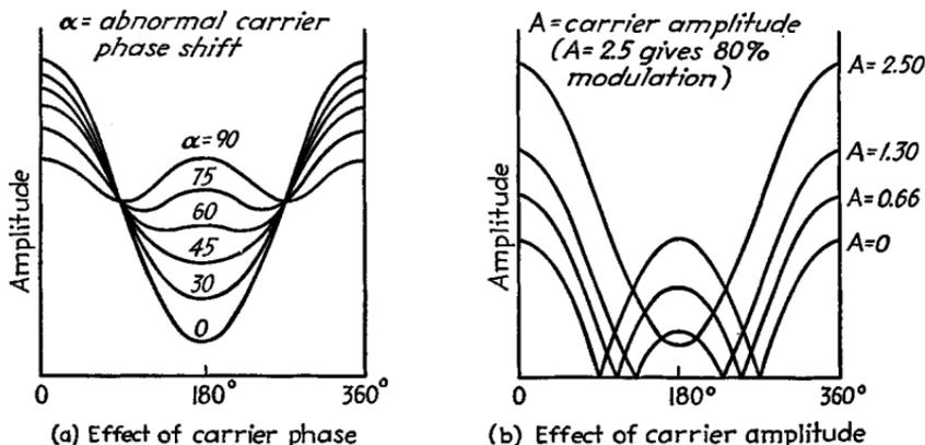
FIG. 46.—Envelope shapes for one modulation cycle, showing effect of varying carrier phase and carrier amplitude (amplitude of individual side-band components constant in all cases).
