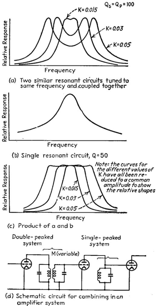
FIG. 37.—Diagram illustrating how band-pass action can be realized by combining a double-humped curve obtained from a pair of coupled circuits, with a simple resonant curve. By using proper circuit proportions, band-pass action is realized irrespective of the coefficient of coupling between the pair of coupled circuits.
