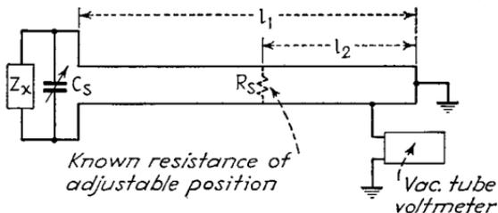
FIG. 25.—Transmission-line arrangement for measuring impedance.
