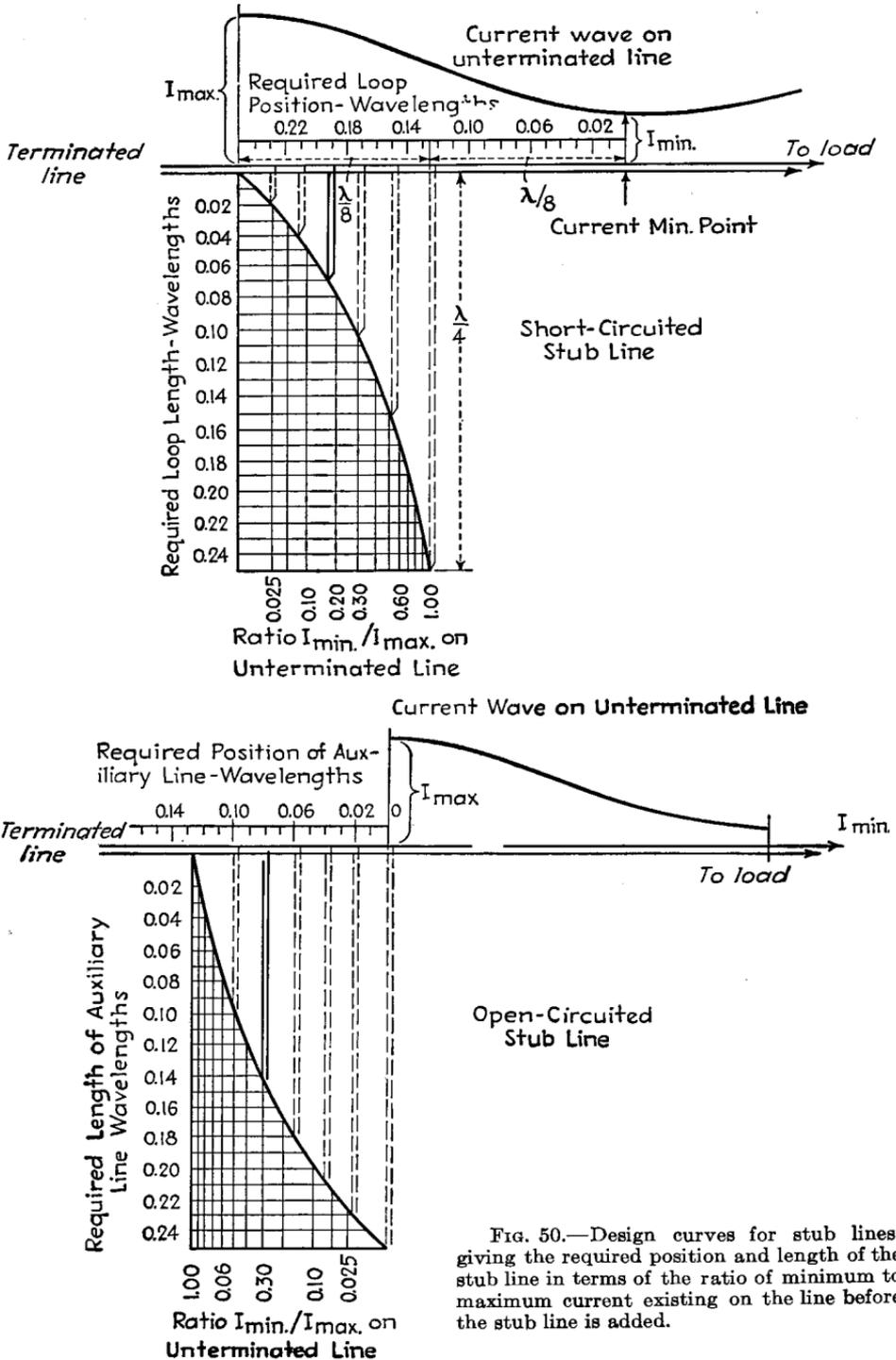
FIG. 50.—Design curves for stub lines, giving the required position and length of the stub line in terms of the ratio of minimum to maximum current existing on the line before the stub line is added.
