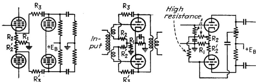
(a) Resistance coupling two-stages (b) Transformer coupling one stage (c) Phase inverter
