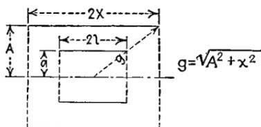
FIG. 42.—Coaxial solenoids not concentric.
