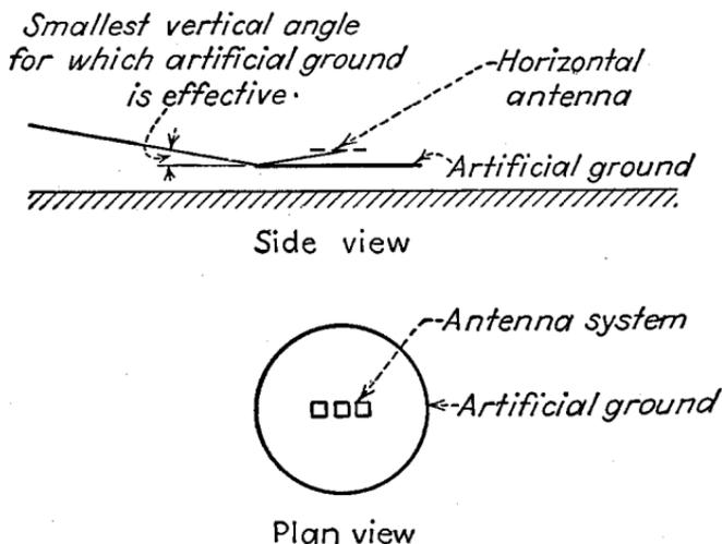
FIG. 18.—Schematic diagram, showing the arrangement of horizontal ultra-high-frequency radio range with artificial ground plane.
