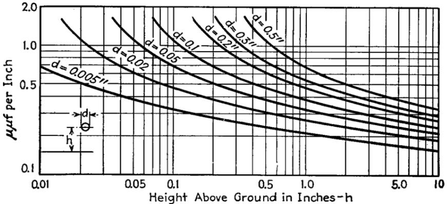
FIG. 76.—Capacity per inch of single-wire conductor of various diameters as a function of height above ground.
