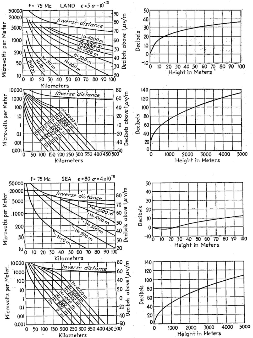
FIG. 68b.—Field-strength curves for 75 mc.
