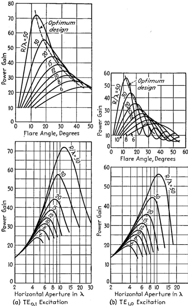
FIG. 73.—Power gain for sectoral horn of Fig. 64 excited by  $TE_{0,1}$  and  $TE_{1,0}$  waves, showing the effect of flare angle and horizontal aperture. These curves are for a vertical aperture of one wave length and give the gain compared with a doublet antenna. For other vertical apertures, the power gain given by the curves should be multiplied by the vertical aperture measured in wave lengths.
