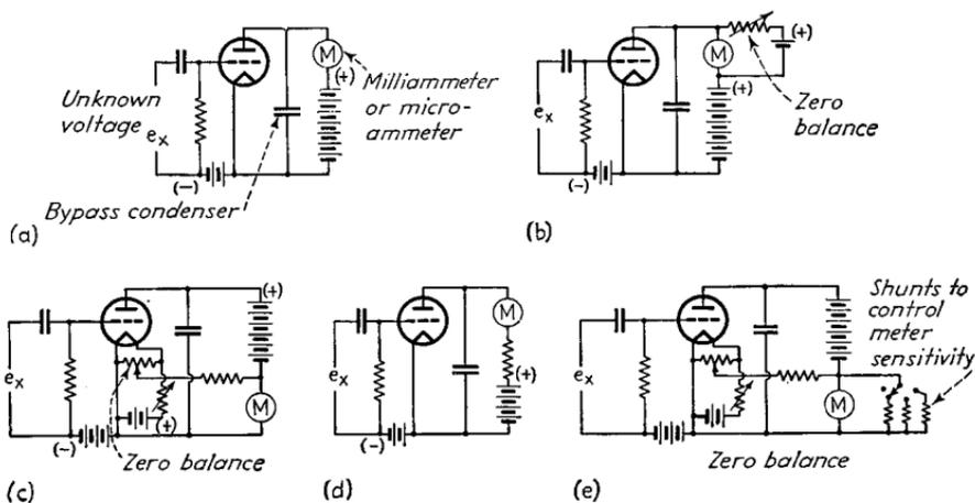
FIG. 38.—Typical vacuum-tube voltmeter circuits.
