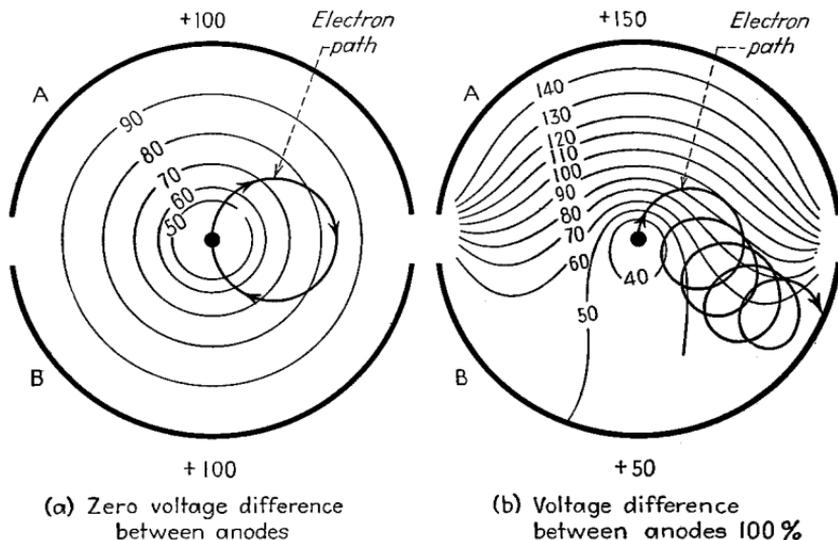
FIG. 44.—Electron paths in split-anode magnetron. The contour lines represent equipotential lines, on the basis that the anode supply voltage is 100 (or 100 per cent).
