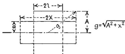
FIG. 44.—Coaxial concentric solenoids, outer coil the shorter.
