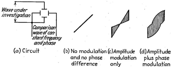
FIG. 97.—Detection of phase modulation accompanying amplitude modulation.
