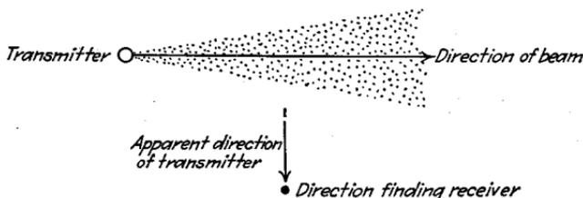
FIG. 45.—Scattering of beam signals in sidewise directions.
