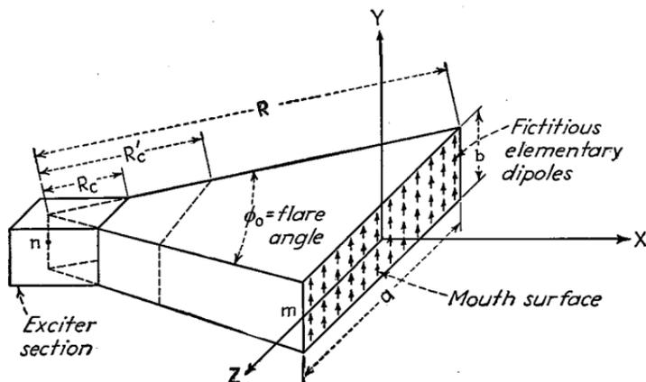
FIG. 64.—Sectoral horn excited by  $TE_{0,1}$  wave. The radiation pattern obtained from the horn can be considered as arising from an array of fictitious elementary dipoles arranged across the mouth of the horn as illustrated and having a strength proportional to  $E(1 + \cos \theta)$ , where  $E$  is the intensity of the electric field at the mouth of the horn and  $\theta$  is the angle with respect to  $XY$  plane.
