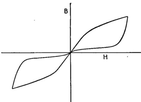
Fig. 66.—Hysteresis loop of permivar at moderate flux density, showing the negligible coercive force and residual magnetization.
