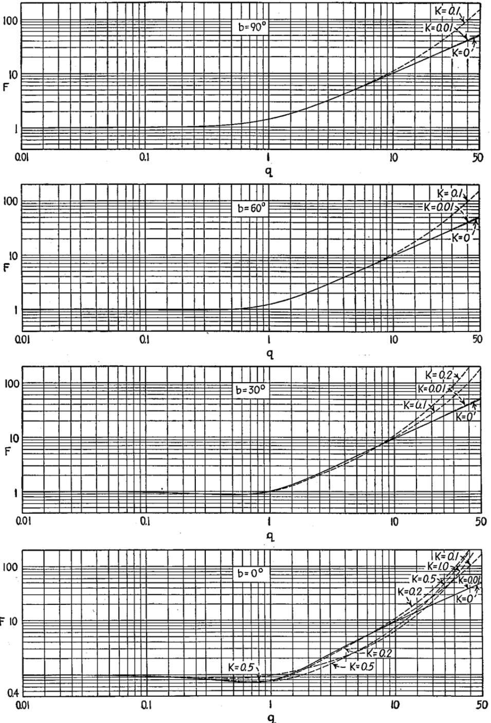
FIG. 16.—Curves giving  $F$  factors for use in Eq. (18) for moderate antenna numerical heights ( $q < 50$ ) when  $K$  cannot be assumed to be negligibly small. (The curves for  $K = 0$  correspond to Fig. 15.)
