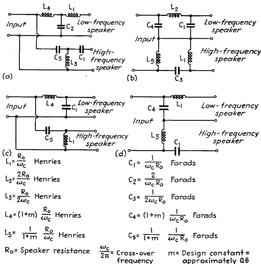
FIG. 115.—Dividing networks of the filter type.
