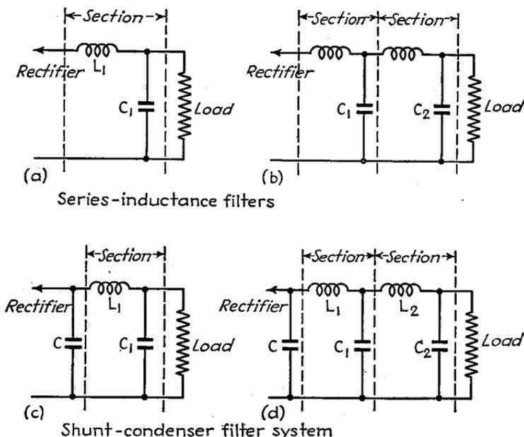
FIG. 11.—Typical inductance-capacity filters.
