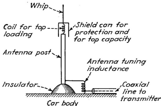
FIG. 94.—Top-loaded antenna for mobile service.
