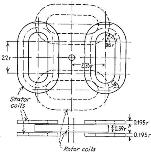
FIG. 57.—Brooks inductometer.
