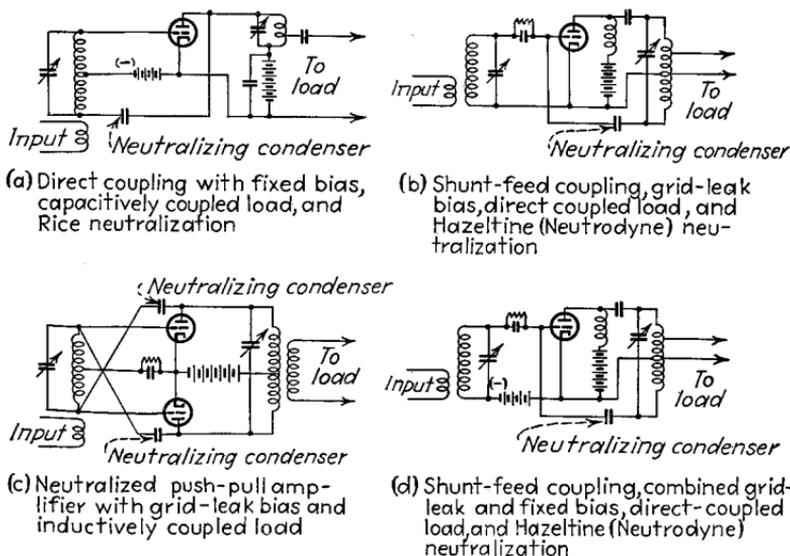
FIG. 75.—Typical circuit arrangements for Class C amplifiers.
