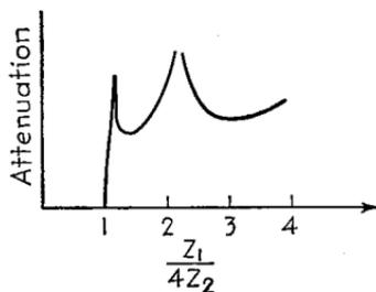
FIG. 102.—Attenuation characteristic of  $MM'$  terminating section.
