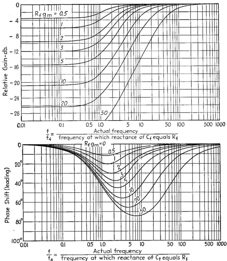
FIG. 6.—Curves giving loss in amplification and phase shift of output voltage occurring at low frequencies in a resistance-coupled amplifier as a result of a resistance-condenser bias impedance  $R_f C_f$  for the case where the screen-circuit impedance has negligible effect upon the amplification, for various values of  $R_f g_m$ .
