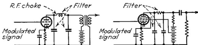
Note: Bias resistors adjusted so that bias approximates cut off with normal rated carrier voltage
