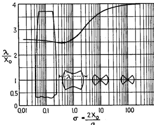
FIG. 133.—Curve giving wave length of ellipsoid-hyperboloid resonators of the type shown in Fig. 131g for different values of the shape factor  $\sigma_0$ . The little drawings show resonator cross sections corresponding to different values of  $\sigma_0$ , and are so scaled that all give the same wave length. Only the upper half of the drawing corresponding to  $\sigma_0 = 0.1$  is shown.
