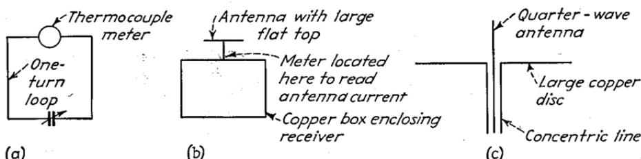
FIG. 99.—Typical antenna arrangements used in standard-field generators.
