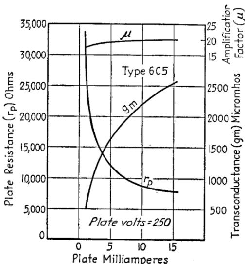
FIG. 17.—Variation of triode constants with plate current.
