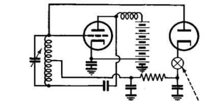
*Introduce modulating voltage here, also bias cathode positively if delay action is desired*
