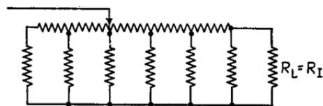
(f) Continuously variable ladder attenuator
