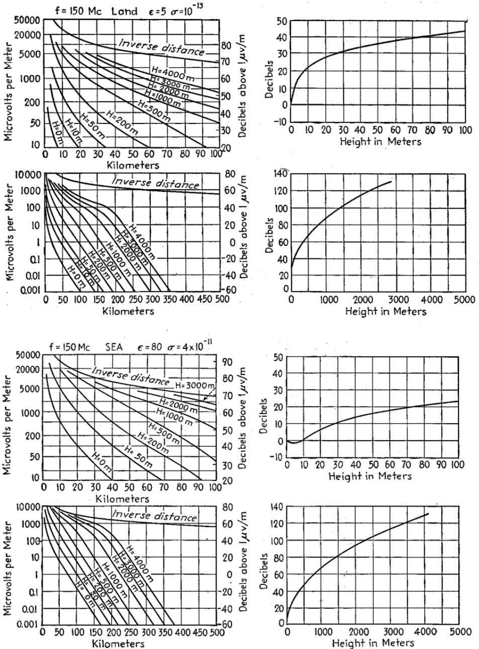
FIG. 68a.—Field-strength curves for 150 mc.
