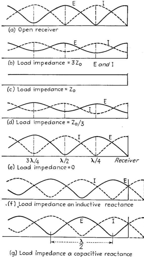
FIG. 43.—Types of voltage and current distributions produced on transmission lines by different load impedances.
