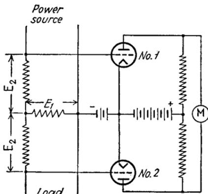
FIG. 44.—Circuit diagram of vacuum-tube wattmeter.
