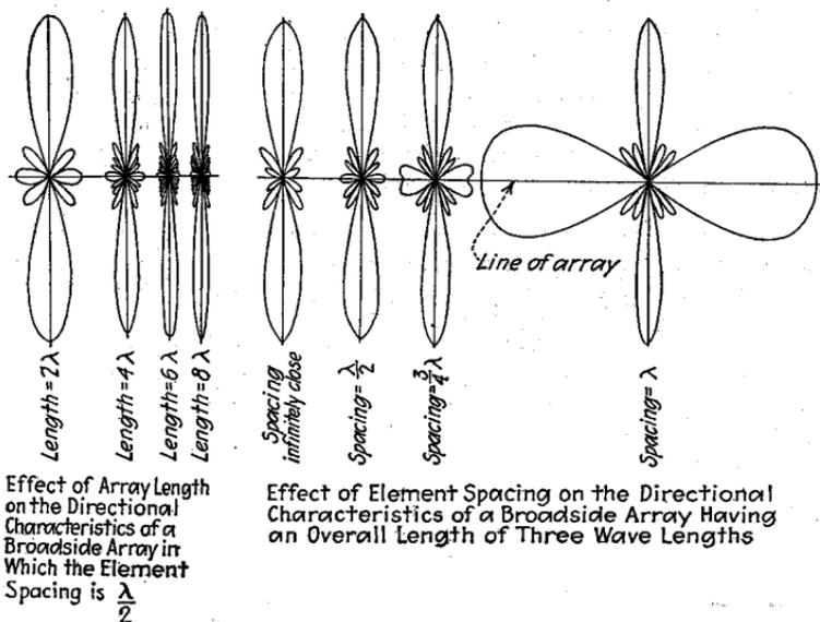
FIG. 31.—Effect of array length and element spacing on directional characteristics of the field radiated from a broadside array under conditions where the individual radiator has a circular pattern in the plane under consideration.
