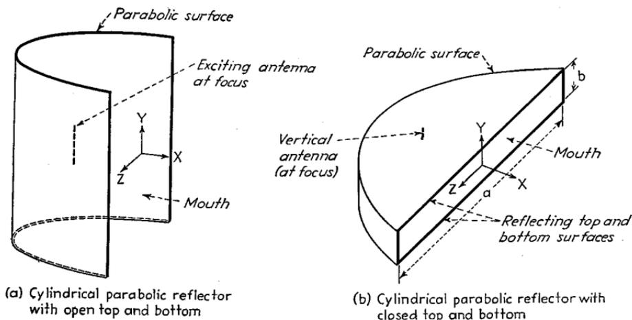
FIG. 84.—Cylindrical paraboloids with open and closed ends.
