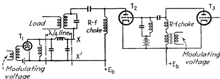
FIG. 15.—High-efficiency modulation system developed by Dome.
