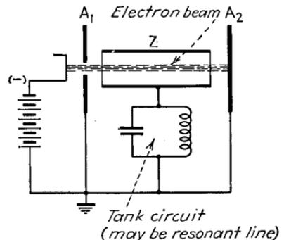
FIG. 46.—Schematic diagram of Heil tube.
