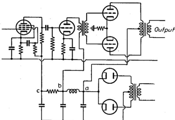
FIG. 15.—Example of graded filter in which the amplifier stages operating at lower power level are provided with progressively increased filtering.
