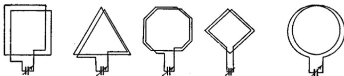
FIG. 49.—Typical loop antennas.
