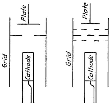
FIG. 58.—Typical thyatron electrode structures.
