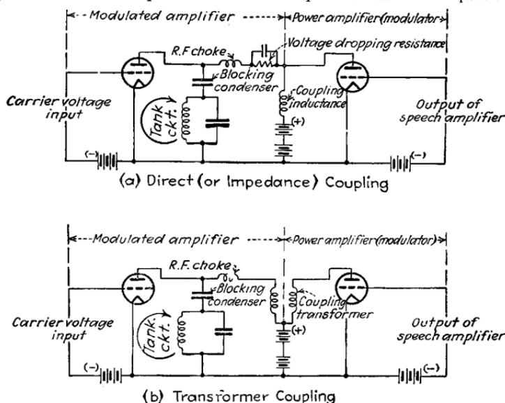
FIG. 2.—Circuit diagrams of typical plate-modulated Class C amplifiers. For the sake of simplicity the neutralizing arrangement for the modulated amplifier is omitted.
