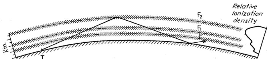
FIG. 27.—Schematic diagram drawn approximately to scale showing location of various ionosphere layers, approximate distribution of ionization, and typical path of a wave refracted from the *F*<sub>2</sub> layer.
