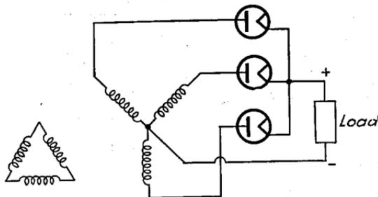
(a) Three-phase half-wave rectifier circuit
