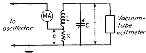
FIG. 21.—Schematic diagram of Q meter.
