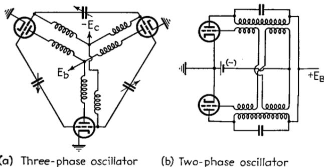
FIG. 36.—Polyphase oscillator circuits.
