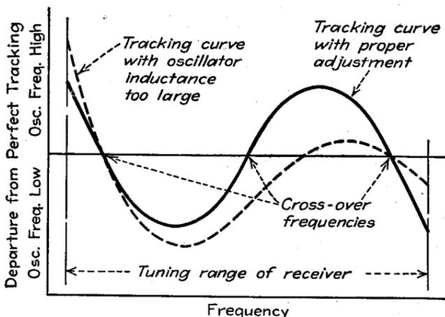
FIG. 20.—Typical tracking curves of superheterodyne oscillator.
