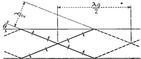
(b) Wave fronts corresponding to Fig. 119 c
