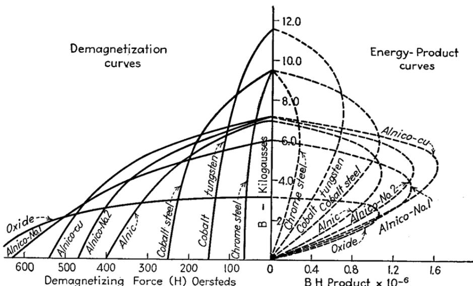
FIG. 68.—Demagnetization curves for permanent magnet materials.
