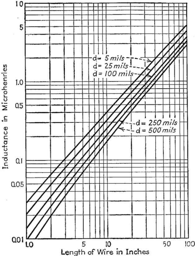
FIG. 15.—Self-inductance of a straight round wire at high frequencies.
