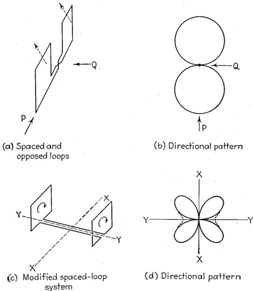
FIG. 11.—Spaced-loop direction-finder systems with corresponding directional patterns.
