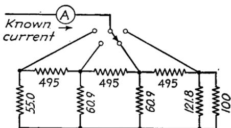
(e) Ladder attenuator with adjacent shunt arms merged, showing numerical values for  $R_1=100$  and a voltage reduction factor  $\alpha$  of 10 per section
