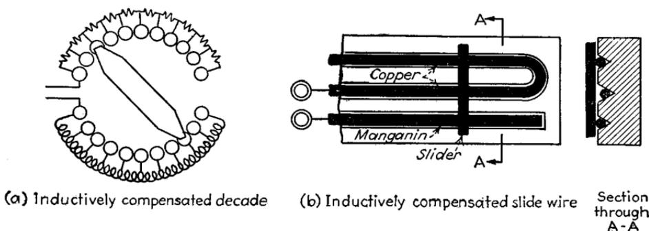
FIG. 14.—Inductively compensated adjustable resistors.
