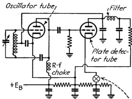
*Introduce modulating voltage here*
