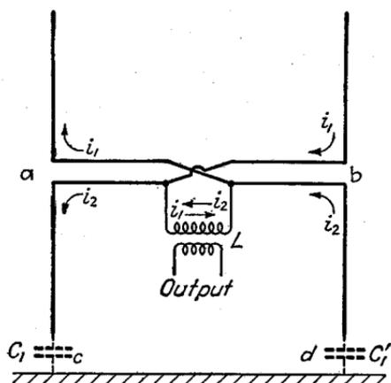
FIG. 8.—Adcock antenna system located close to earth.
