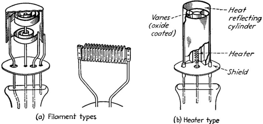
FIG. 55.—Hot-cathode emitting structures.
