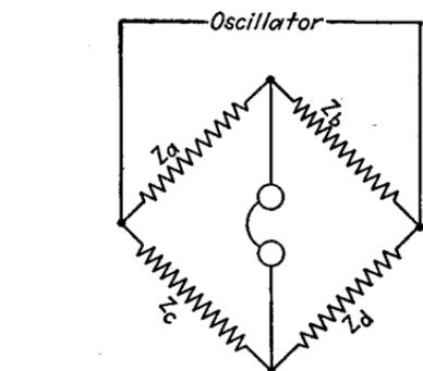
FIG. 4.—Schematic diagram of alternating-current bridge.
