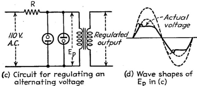
FIG. 21.—Methods of utilizing a neon tube for voltage regulation.
