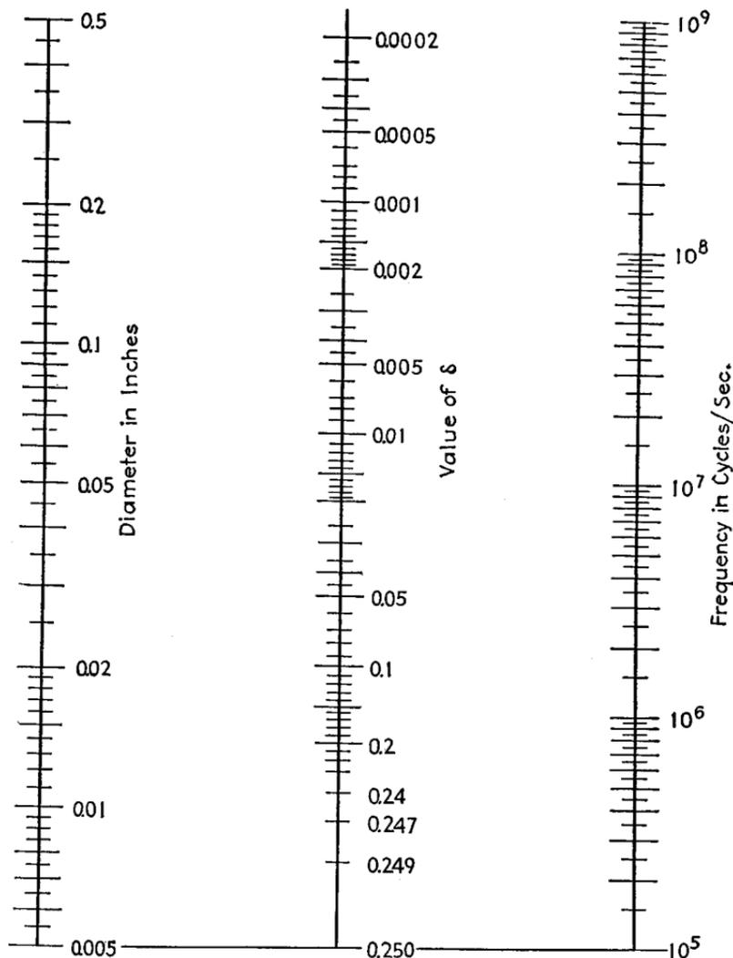
FIG. 16.—Skin-effect correction factor  $\delta$  as a function of wire diameter and frequency.
