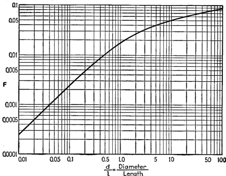
FIG. 19.—Factor  $F$  for single-layer solenoid in Eq. (36).
