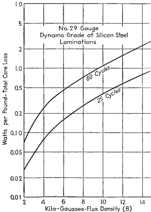
FIG. 63.—Core-loss curves of typical silicon steel sample.
