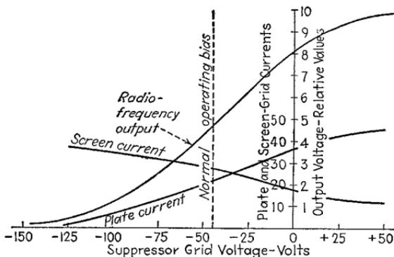
FIG. 10.—Linearity curve of typical suppressor-grid modulated amplifier. Note that it is impossible to obtain complete modulation without introducing appreciable distortion.
