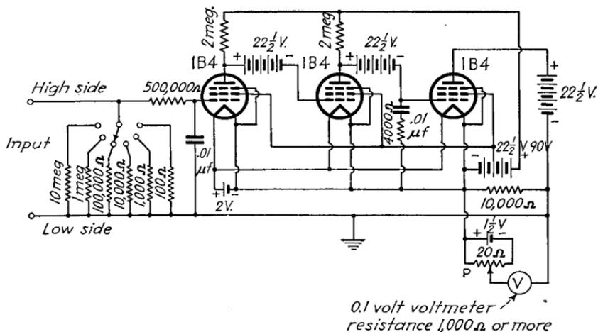
FIG. 43.—Circuit of battery operated vacuum-tube microammeter of feedback type, having full-scale ranges of  $10^{-8}$  to  $10^{-3}$  amperes, suitable for use with ionization gages.
