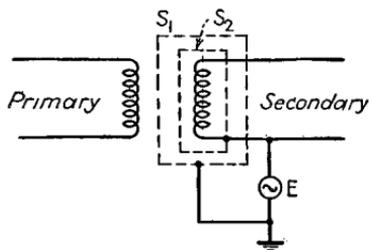
FIG. 94.—Schematic diagram of a double electrostatic shield.
