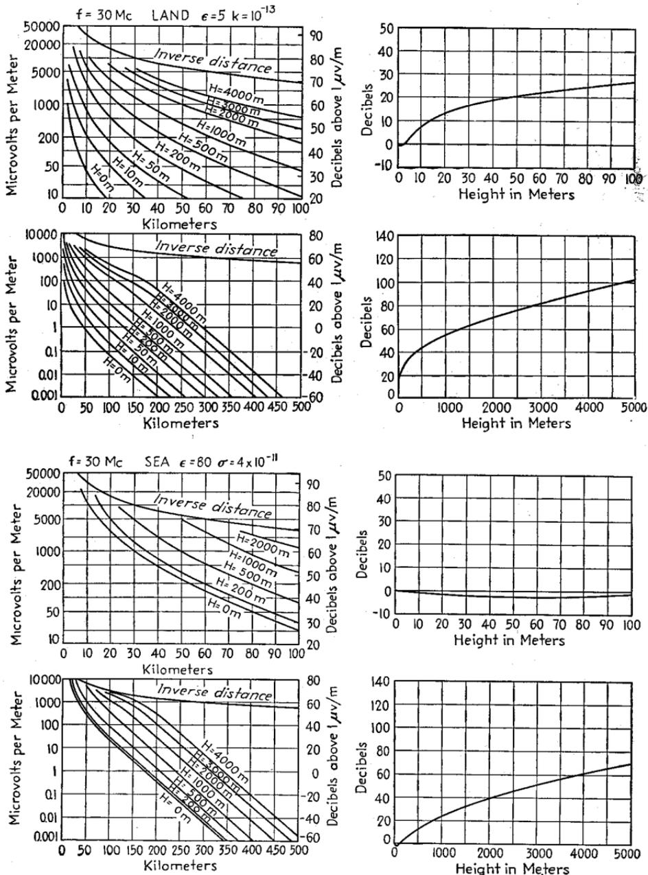
FIG. 68c.—Field-strength curves for 30 mc.
