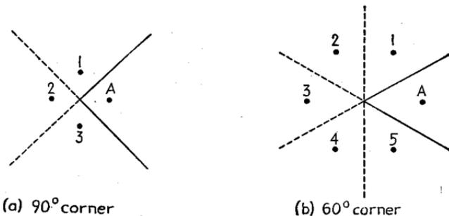
FIG. 58.—Image system for corner antennas. Here *A* represents the exciting antenna, and the numbered antennas are images. The antenna *A*, in conjunction with its associated images (and in the absence of all reflectors), produces the same field in the direction of the reflector mouth as does the system consisting of *A* and the corner reflector.
