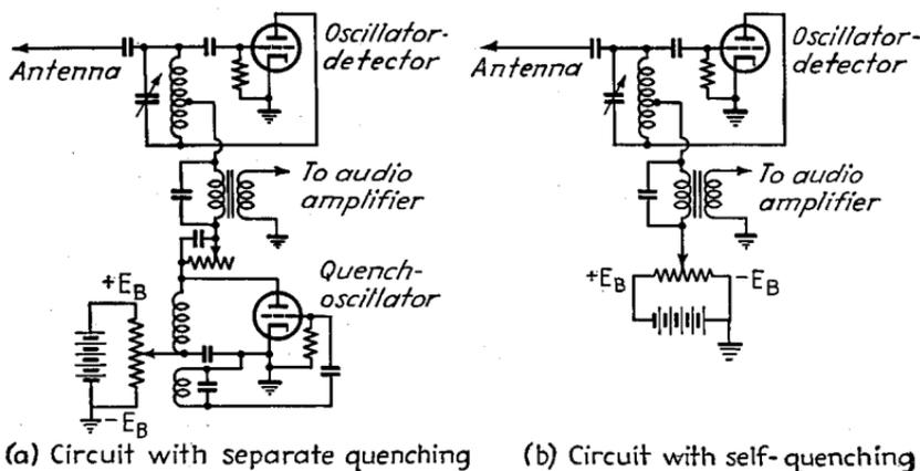
FIG. 32.—Typical circuits of superregenerative receivers.
