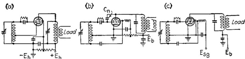
FIG. 4.—Electron-coupled oscillator circuits.
