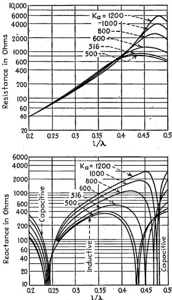
FIG. 101.—Resistance and reactive components of impedance of cylindrical antenna of Fig. 100a as calculated for different values of characteristic impedance  $K_a$ . (After Schelkunoff.) These curves assume that the resistance and reactive components are in series with each other and neglect the effect of any lumped shunting capacity that may be present across the input terminals.
