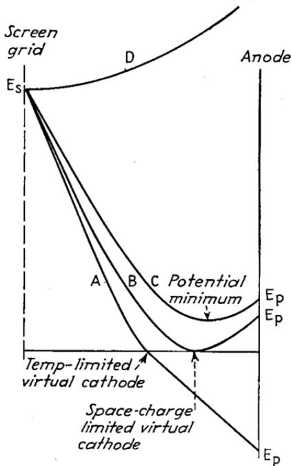
FIG. 12.—Types of potential distributions encountered in the screen-plate region of beam power tubes.
