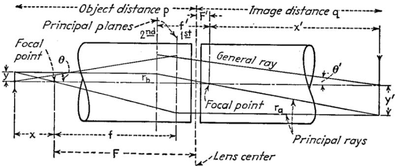
FIG. 44.—Image formation in thick electron lens.
