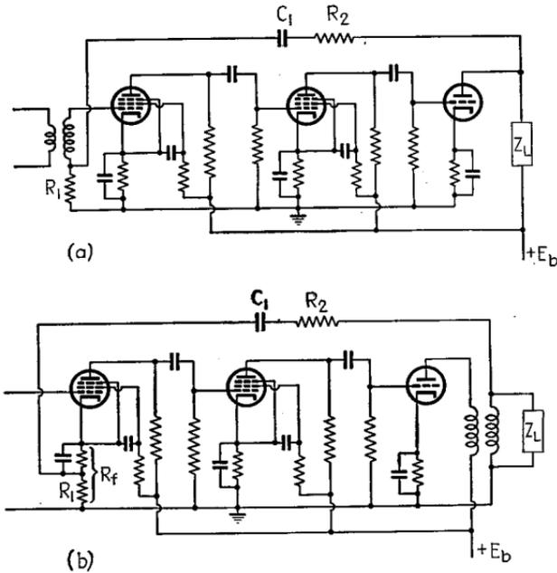
FIG. 36.—Typical feedback circuits involving three stages of amplification. In practice these circuits may be modified by expedients such as shown in Fig. 93, Sec. 3 in order to control  $A\beta$  at high and low frequencies.
