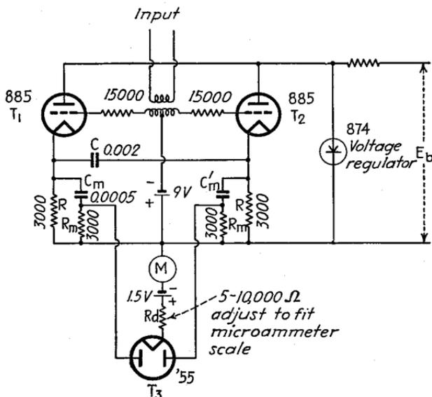
FIG. 63.—Electronic-frequency meter.
