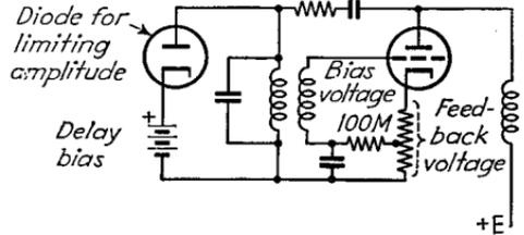
FIG. 26.—Resistance-stabilized oscillator employing feedback, provided with diode for limiting the amplitude.
