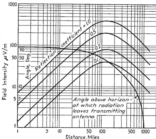
FIG. 55.—Curves useful in the calculation of sky-wave intensity at broadcast frequencies. These curves assume that the wave is reflected from the *E* layer at a height of 100 km and that the transmitting antenna radiates a field 100 mv/m at one mile along the horizontal, with the strength at angles above the horizontal proportional to the cosine of the angle of elevation. The curves take into account the curvature of the earth.
