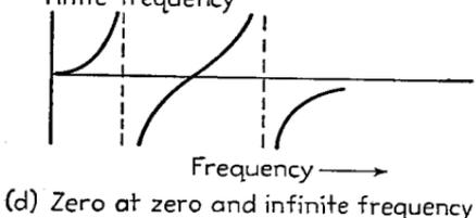
FIG. 63.—Reactance as a function of frequency for various classes of reactive networks.
