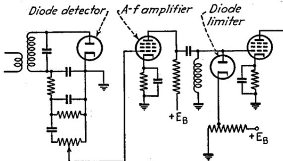
FIG. 25.—Limiter system for noise suppression.
