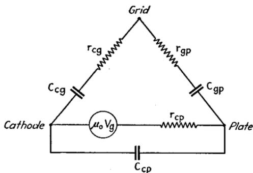
FIG. 29.—Equivalent delta of a triode at ultra-high frequencies.
