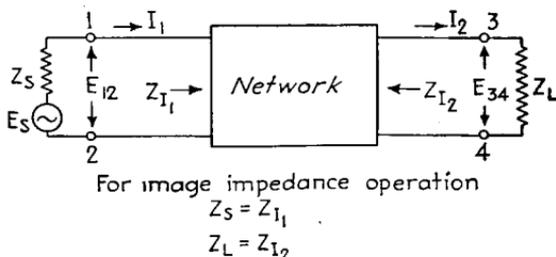
FIG. 67.—Four-terminal network operated with terminal impedances.
