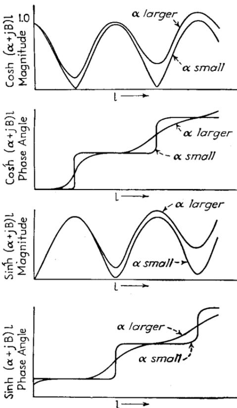
FIG. 41.—Curves showing the nature of the functions  $\text{cosh } (\alpha + j\beta)$  and  $\text{sinh } (\alpha + j\beta)$ .
