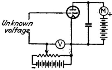
FIG. 39.—Slide-back vacuum-tube voltmeter.
