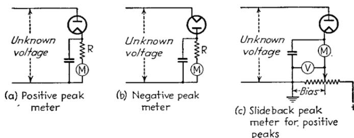
FIG. 41.—Circuits of typical diode vacuum-tube voltmeter.
