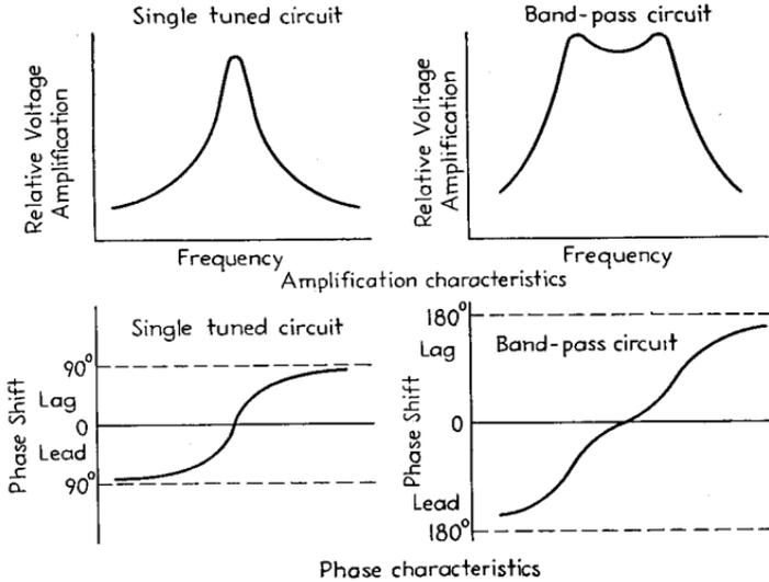
FIG. 69.—Curves showing amplification and phase-shift characteristic as a function of frequency with tuned amplifiers having a single tuned circuit and having a band-pass characteristic.
