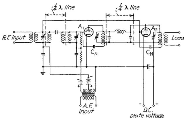
FIG. 7.—Schematic circuit diagram of high-efficiency grid-modulated amplifier.
