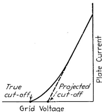
FIG. 30.—Curve illustrating meaning of projected cutoff.
