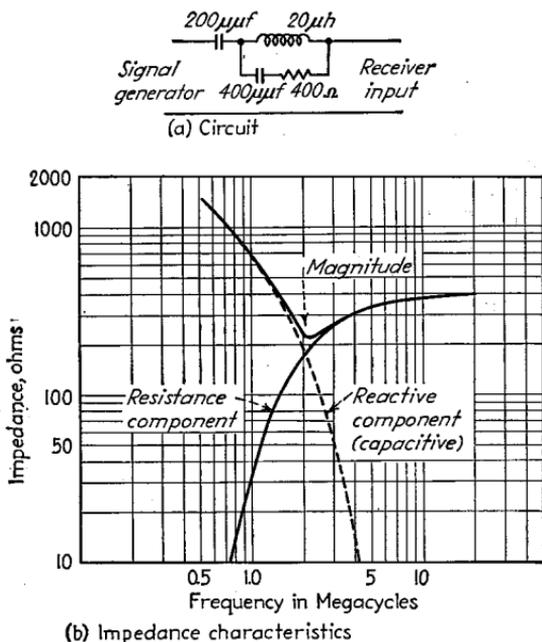
FIG. 78.—Standard dummy antenna used for testing broadcast receivers, together with its impedance characteristic.
