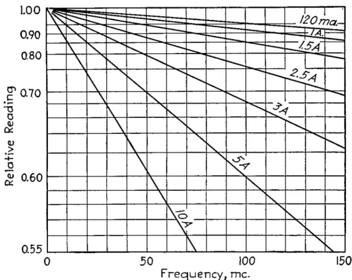
FIG. 35.—Curves giving high-frequency correction for certain commercial thermocouple instruments.
