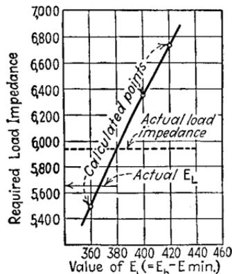
FIG. 81.—Determination of the actual output voltage for a known load impedance by plotting a curve of load impedance required for several assumed values of output voltage.
