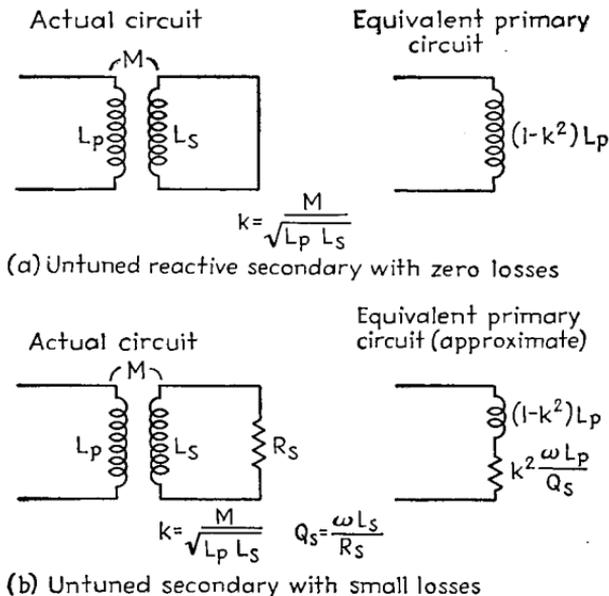
FIG. 14.—Inductively coupled circuits with untuned secondaries.
