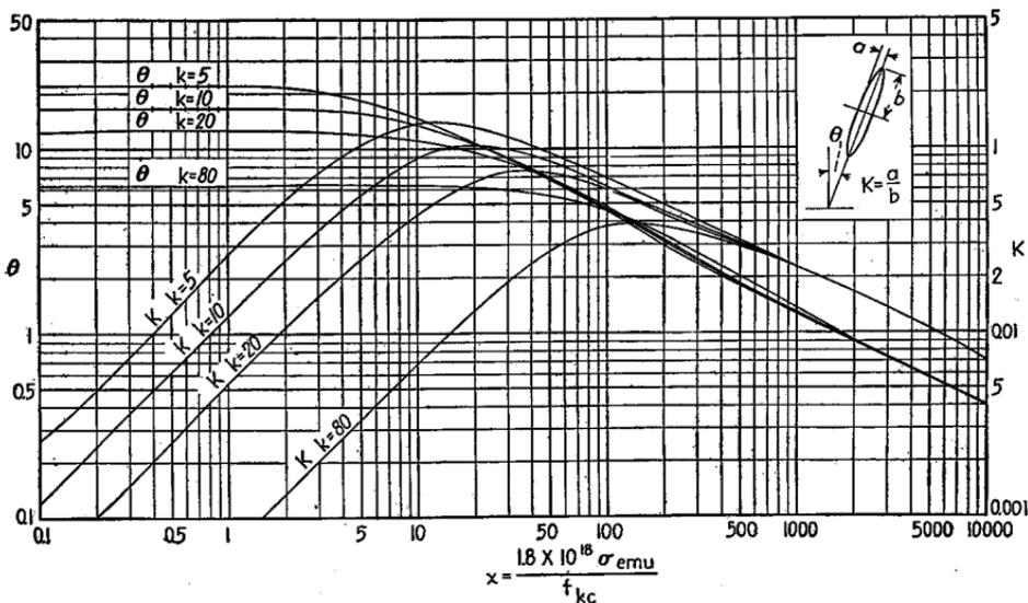
FIG. 23.—Characteristics of wave tilt for different values of dielectric constant  $k$  and ground-conductivity factor  $x$ .
