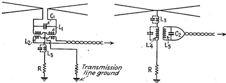
(b) Antenna and equivalent coupling circuit at high frequencies (c) Antenna and equivalent coupling circuit at low frequencies
