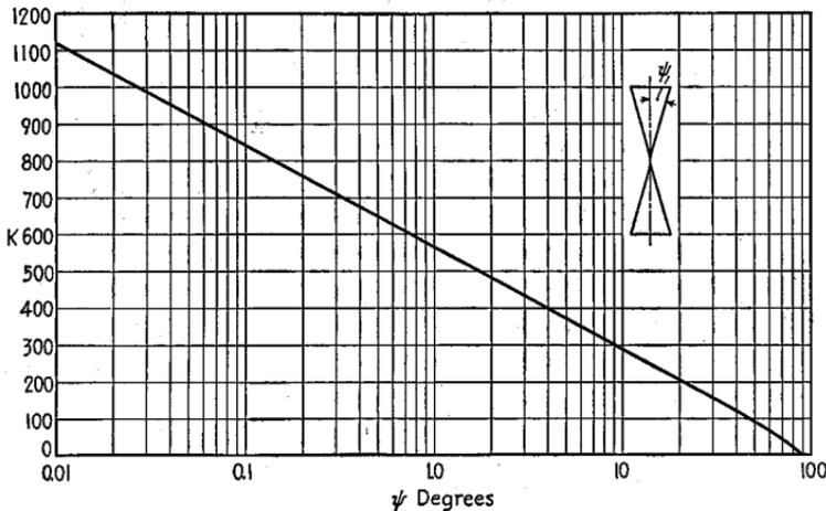
FIG. 108.—Characteristic impedance  $K$  of conical antennas as a function of angle of revolution  $\psi$  (see Fig. 100b).
