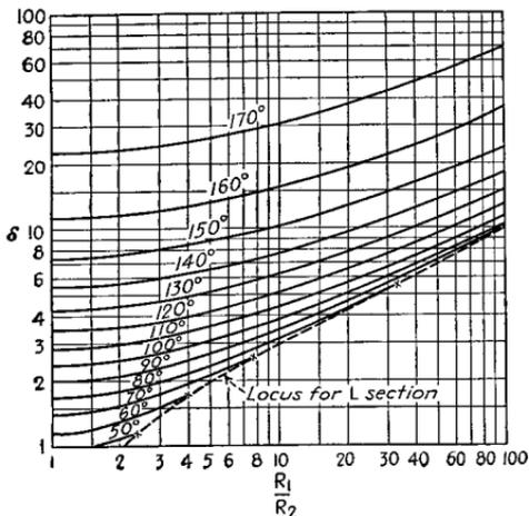
FIG. 79.—Values of  $\delta$  for use in Eq. (115), applicable for Type 1 and Type 3 networks of Fig. 74. The angles are values of  $\beta$ .
