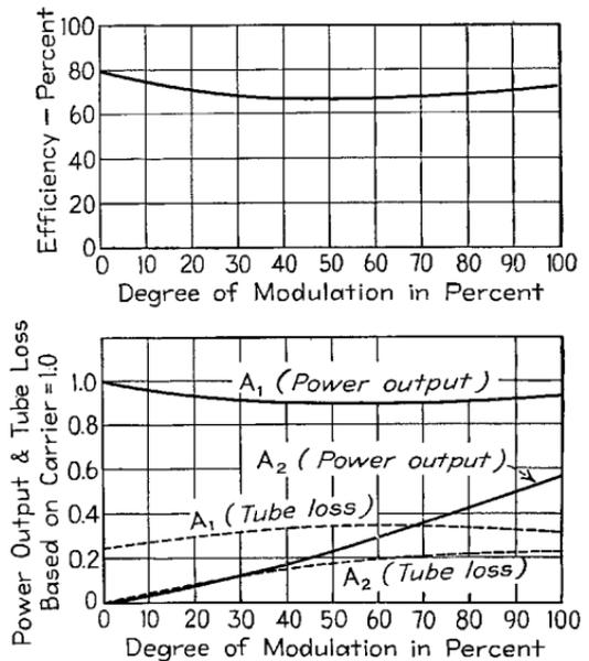
FIG. 8.—Performance of ideal grid-modulated amplifier, on the basis of a Class C amplifier efficiency of 80 per cent.
