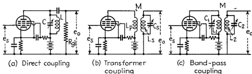
FIG. 67.—Typical tuned-amplifier circuits.
