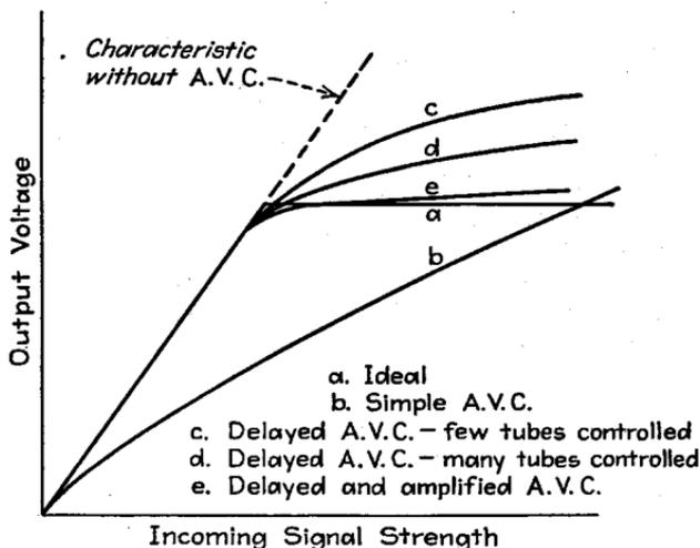
FIG. 12.—Automatic-volume-control characteristics under different conditions.
