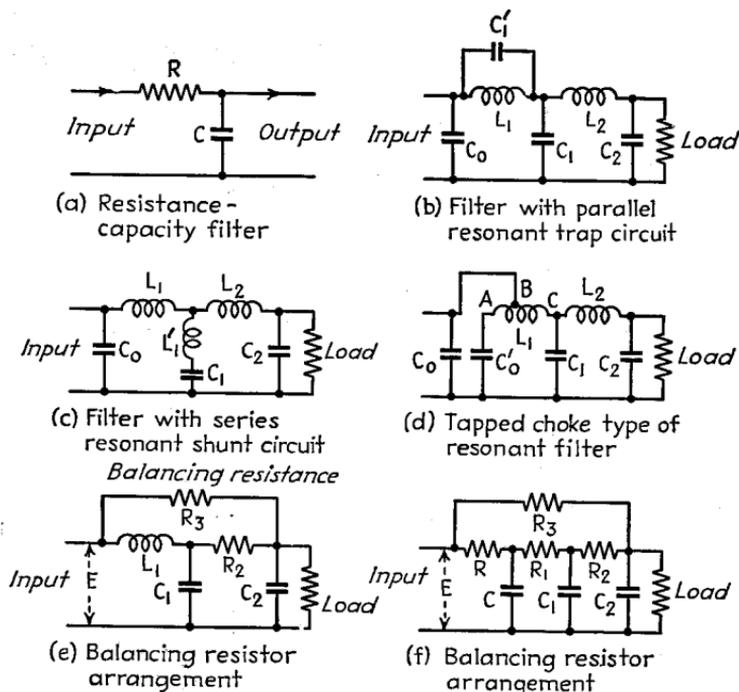
FIG. 13.—Miscellaneous filter circuits.
