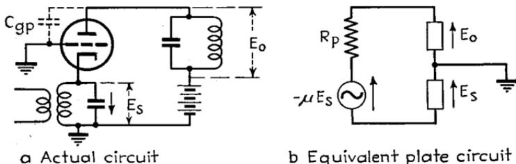
FIG. 93.—Grounded-grid self-neutralized circuit.
