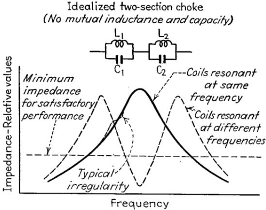
FIG. 56.—Impedance characteristics of idealized radio-frequency choke coils.
