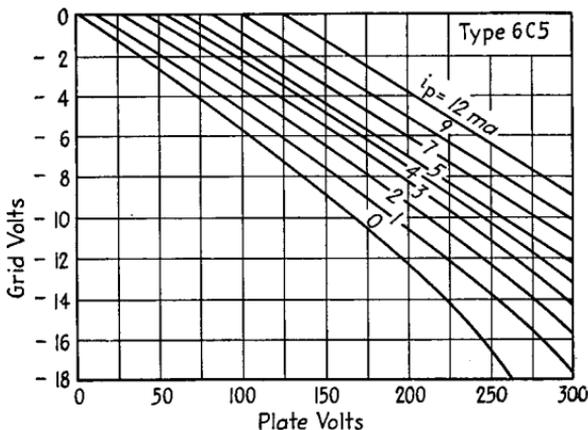
FIG. 16.—Constant-current curves of a triode.
