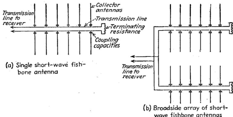
FIG. 44.—Plan view of single fishbone antenna and of an array consisting of two such antennas in broadside.
