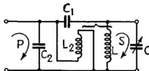
$$m = \frac{LC_1}{C_1 + C_2} + \frac{M_2 + \frac{LC_1}{C_1 + C_2}}{\left(\frac{\omega}{\omega_2}\right)^2 - 1}$$
