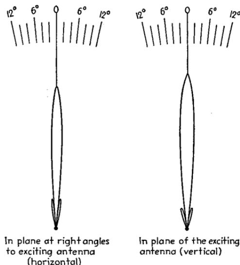
FIG. 81.—Directional pattern of rotational parabola excited by doublet antenna having a mouth diameter of  $12\lambda$  and a focal length of 0.625 times the mouth radius. The amplitudes of the minor lobes are exaggerated for clarity.
