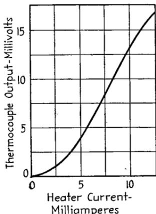
FIG. 33.—Typical calibration curve of a vacuum thermocouple.
