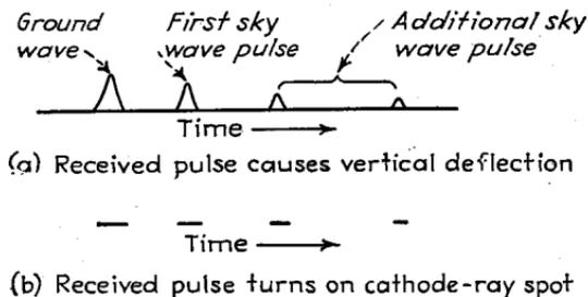
FIG. 38.—Example of oscillograms received when a transmitter is within ground-wave range, and the transmitted signal consists of a short wave train. The additional sky-wave pulses may be either multiple reflections of the first pulse or waves returned from higher layers. In many cases the additional sky-wave pulses are absent.
