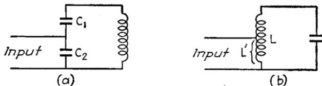
FIG. 11.—Tapped parallel resonant circuits.
