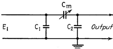
FIG. 89.—Equivalent circuit of capacity attenuators.
