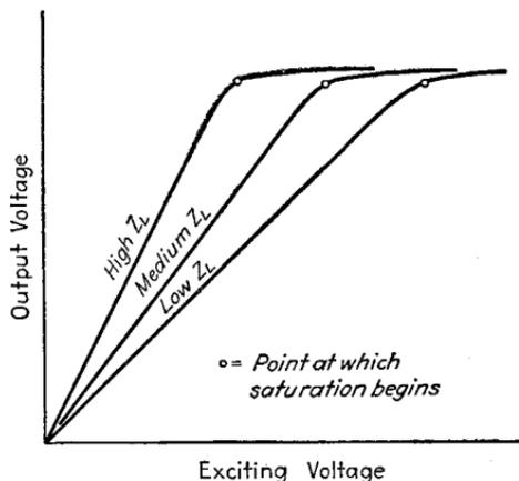
FIG. 79.—Typical linearity curves of linear amplifier with different load impedances in the plate circuit.
