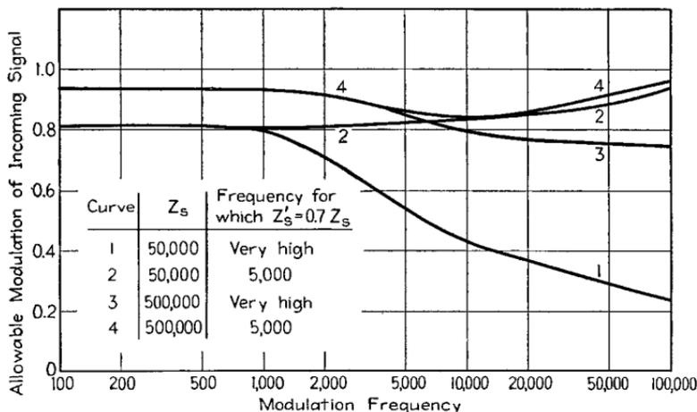
FIG. 30.—Typical curves showing effect of source impedance and of  $Q$  of source impedance on the allowable degree of modulation a signal may have without peak clipping. This figure assumes the detector circuit of Fig. 29c.
