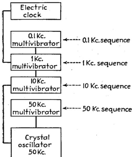
FIG. 57.—Primary standard of frequency with typical multivibrator arrangement.
