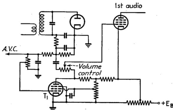
FIG. 21.—Circuit diagram of typical muting system.
