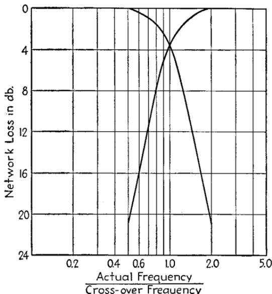
Fig. 114.—Characteristics of a typical dividing network.
