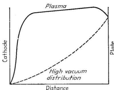
FIG. 53.—Potential distribution in a gas diode.
