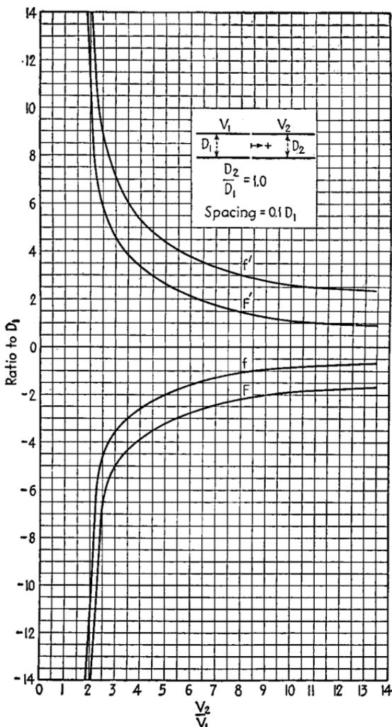
FIG. 45.—Focal characteristics of two-diameter cylinder lenses as a function of electrode voltage ratio. Figure continued on pages 327–330.
