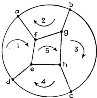
FIG. 60.—Network illustrating meshes, branches, and branch points.
