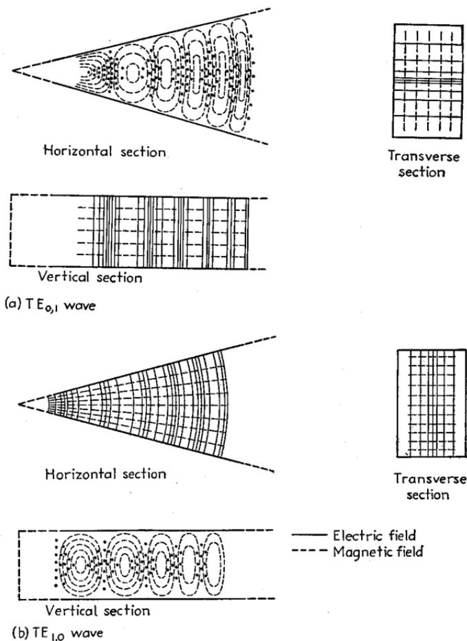
FIG. 66.—Field distributions corresponding to  $TE_{0,1}$  and  $TE_{1,0}$  waves in the sectoral horn of Fig. 64.
