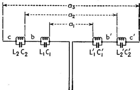
FIG. 95.—Multifrequency antenna.
