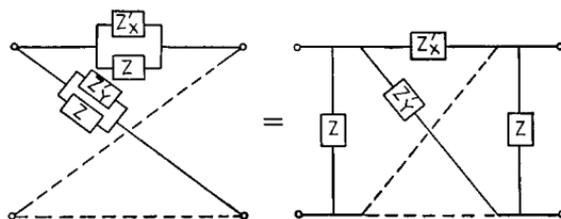
(b) Lattice structure with developed shunt impedances
