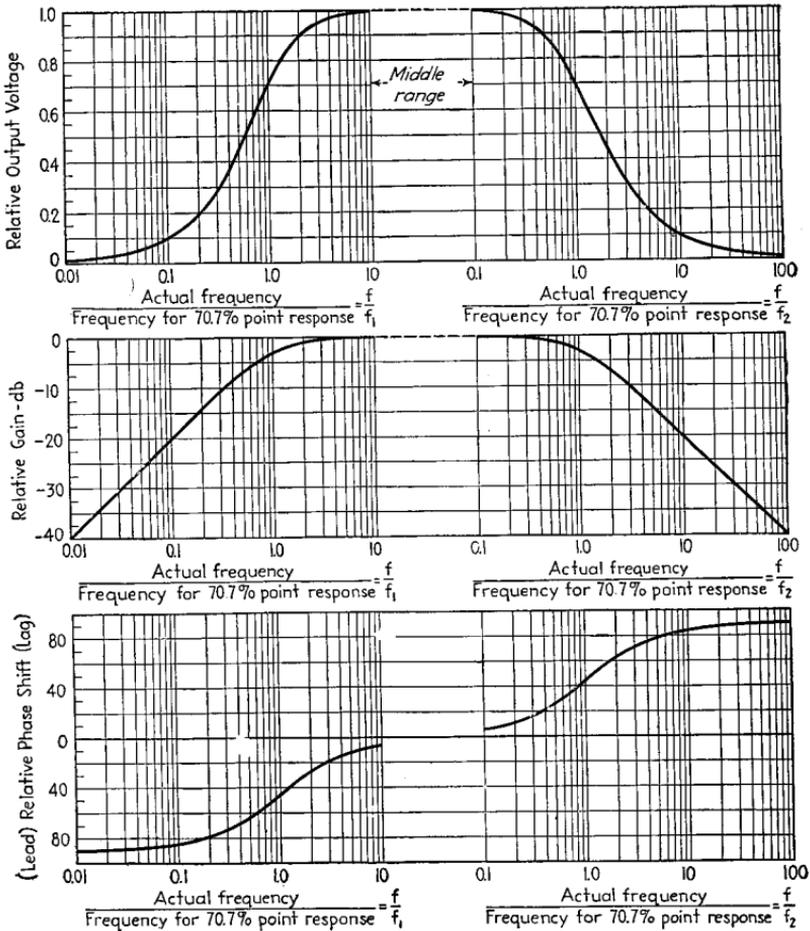
FIG. 25.—Universal amplification curve of transformer-coupled power amplifier.
