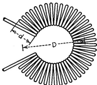
FIG. 22.—Toroidal coil of circular cross section showing notation of Eq. (42).
