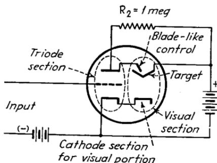
FIG. 38.—Circuit illustrating operation of visual indicator tube.
