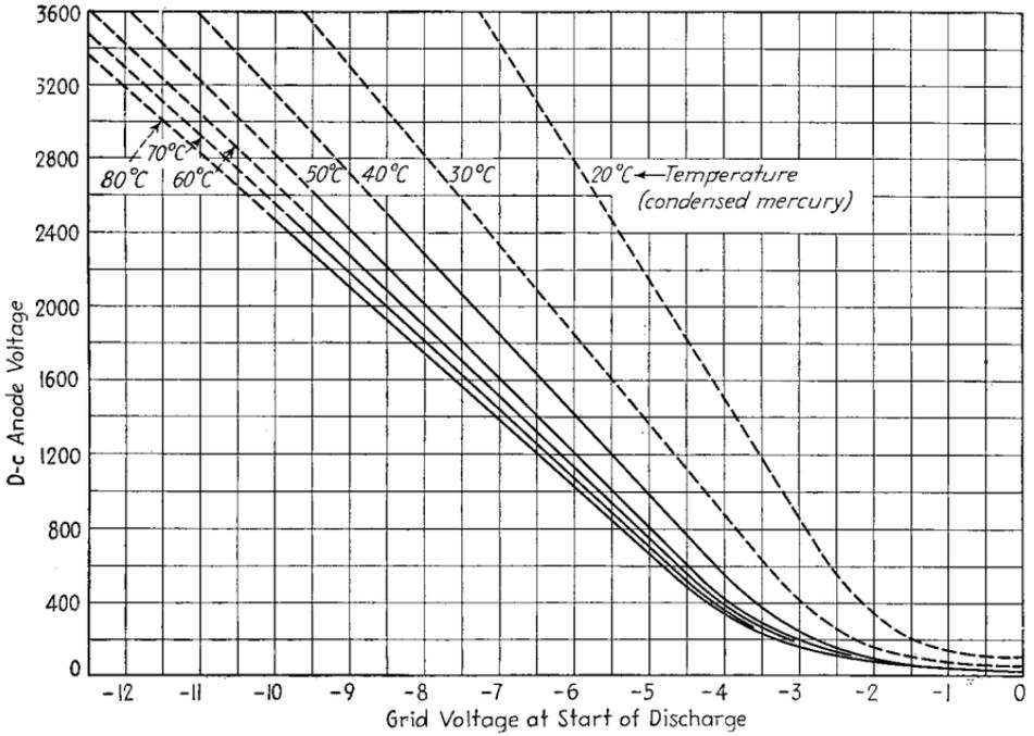
FIG. 56.—Starting characteristics of a typical thyatron using mercury.
