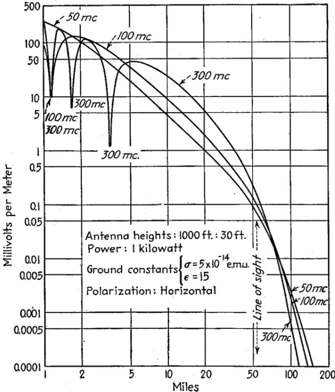
Fig. 67.—Effect of frequency on ground-wave field intensity.
