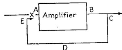
FIG. 88.—Schematic feedback amplifier diagram.
