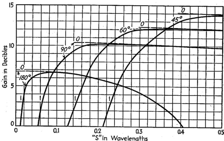
FIG. 59.—Power gain of corner-reflector antenna systems compared with a half-wave antenna in free space for different values of the corner angle  $\alpha$ . The curves marked "0" are for zero loss resistance; those marked "1" are for an assumed loss resistance of the exciting antenna of 1 ohm.
