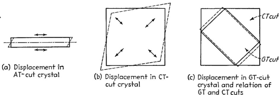
FIG. 9.—Displacements produced by the vibrations in various crystal cuts.
