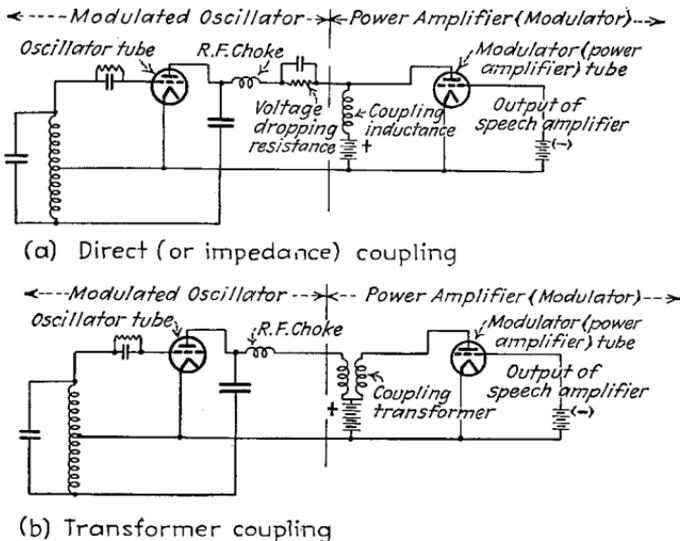
FIG. 20.—Circuit diagrams of typical plate-modulated oscillators.
