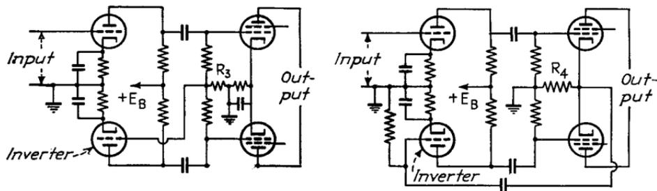
(d) Inverter excited from unbalance in grid-leak currents (e) Inverter excited from unbalanced current in cathode resistance  $R_4$
