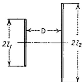
FIG. 36.—Two parallel symmetrically placed wires.
