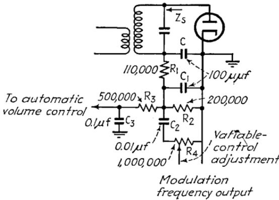
(c) Typical circuit constants used for (b) suitable for broadcast receivers
