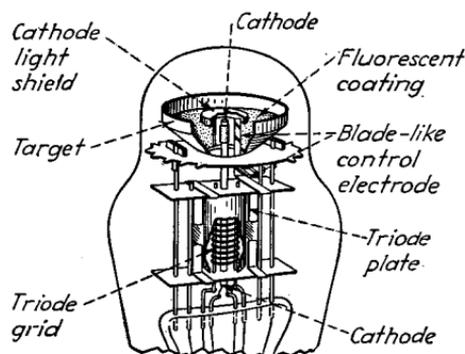
FIG. 37.—Cutaway view of visual indicator tube.
