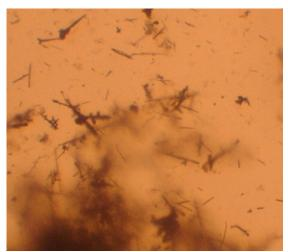
*Microscopic close-up of Pb dendrites in suspension.*
