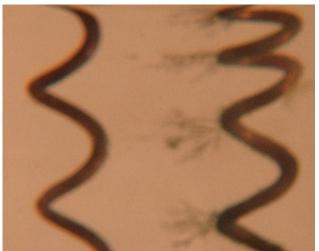
Anode on right showing dendrite growths
