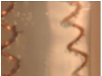
De-ionised water cell electrolysis with DC
