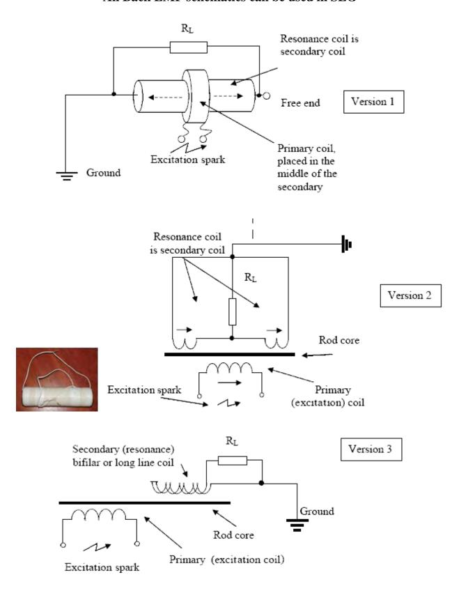
**COMMENTS:** No current will be produced in the load in any of these circuits, unless there is a ground connection. Is excitation possible with just a single spark (???)
