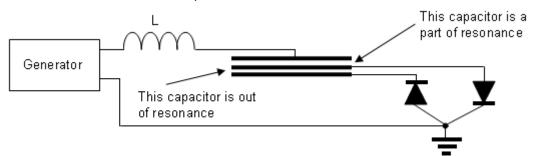
**COMMENT:** You can add an ordinary, very large capacitor in parallel with the "pumping" capacitor for more impressive results.
