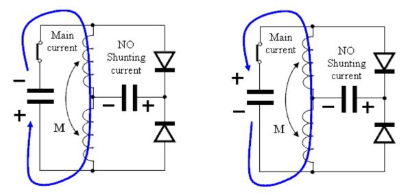
There is no shunting current, if the output capacitor is charged.
