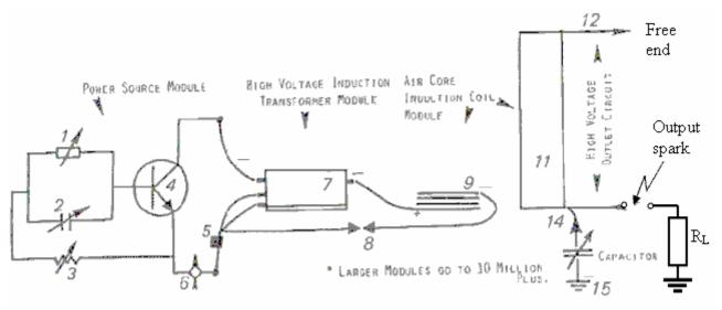
PARTS: 1. COIL, VARIABLE, 2. CAPACITOR, VARIABLE, 3. RESISTOR, VARIABLE, 4. TRANSISTOR, R.F.,
