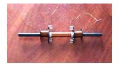
**EXPLANATION:** The central section of the coil and it's two end sections are wound in opposite directions.
