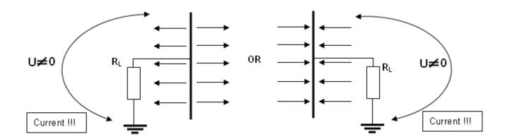
**REMARK:** We get the same situation, if only one plate of an ordinary capacitor is charged. So far, connecting an <u>uncharged plate</u> of an ordinary capacitor to the ground we get a current flowing in this circuit also (because there is an external field).
