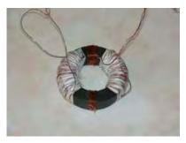
A coil was wound on a toroidal ferromagnetic core with permeability 1000 (not important). Each half-coil was 200 turns (not important), of 0.33 mm diameter wire (not important). The total inductance  $L_{\rm S}$  is about 4 mH (not important).
