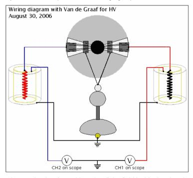
**EXPLANATION:** The charging mechanism is unable to "see" the field inside the charging capacitors.
