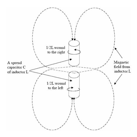
In this case instead of using a capacitor, the capacitance between the two sections of inductor L provides the necessary capacitance.
