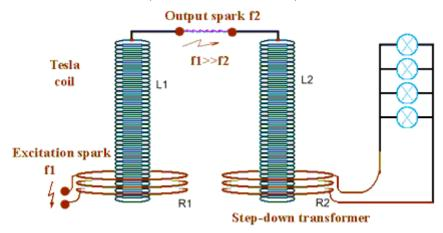
**COMMENT:** The L1 Tesla coil shown above, is energised by spark f1. Resonant, step-down transformer L2 is connected to the L1 Tesla coil by output spark f2. The frequency of f1 is much higher than that of f2.
