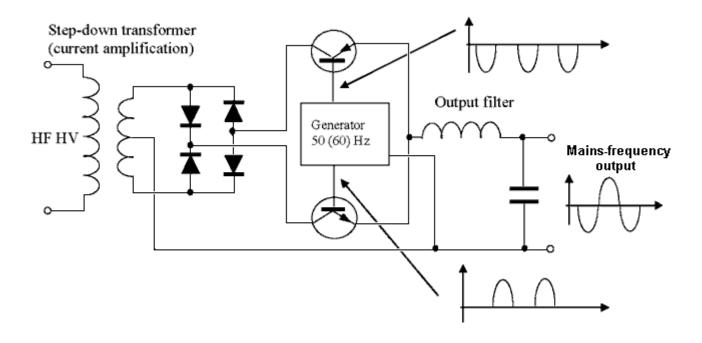
**COMMENTS:** It is possible to use square waves instead of sine waves to ease the loading on the transistors. This is very similar to the output sections of Tariel Kapanadze's patents. This method does not require a powerful transformer with a huge core in order to provide 50 Hz or 60 Hz.
