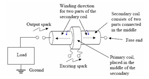
**Explanation:** The exciting (driving) current and the load current in an electromagnetic field, are perpendicular to each other as shown here:
