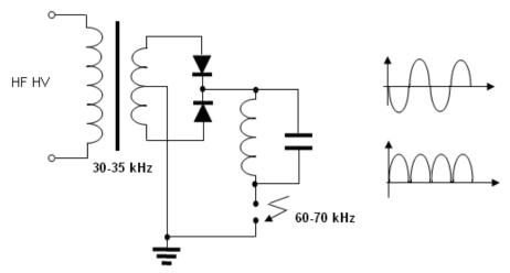
**COMMENTS:** Resonance frequency of the circuit is about 60-70 kHz, but dimmer is for 30-35 kHz. For adjusting the excitation frequency, voltage/frequency technology was used.
