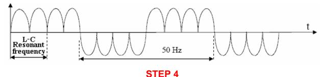
Finally, the oscillations are smoothed by filtering to provide mains-frequency output power.
