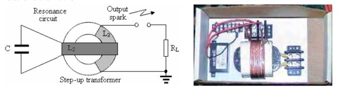
**COMMENTS:** Between sparks, L2 has a voltage on it's ends. If RL is connected directly to L2 then there will be no output current without resonance and there will be no output current without a spark.
