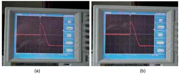
The recharging accuracy was improved to 10 percent. Also, a check measurement was made **without the second diode**. The result was essentially the same as the measurement which used the shunting diode. The missing 10 percent of the voltage can be explained as losses due to the spread capacitor's inductance and in it's resistance.
