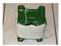
An ordinary laminated iron core transformer intended for 50-60 Hz power supply use (size is not important) was wound with a coil placed on each of it's two halves. The total inductance L<sub>S</sub> is about 100 mH (not important).
