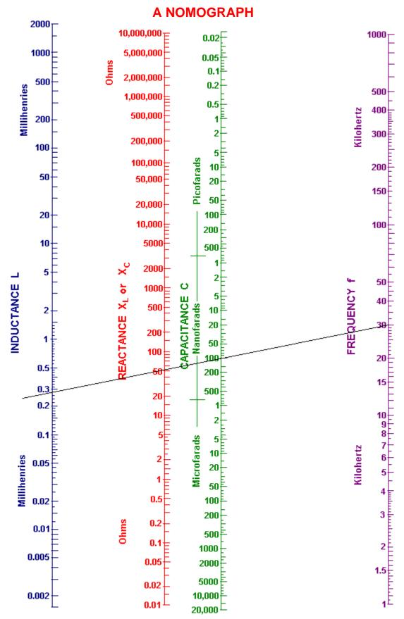
**Using a nomograph:** Draw a straight line from your chosen 30 kHz frequency (purple line) through your chosen 100 nanofarad capacitor value and carry the line on as far as the (blue) inductance line as shown above.
