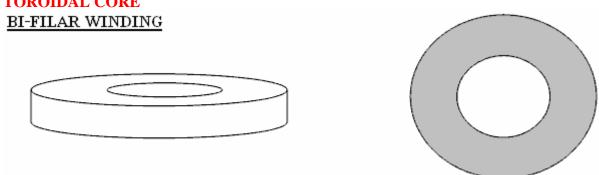
**COMMENTS:** An ordinary excitation winding is wound all of the way around a toroidal core. A bi-filar output winding is wound around the whole of a toroidal core. Remember about the "Hot" and "Cold" ends of a bi-filar coil.
