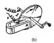
An ordinary unipolar motor consists of a magnetised disk, and a voltage applied between the axis and a point on the circumference of the disc as shown in (a) above. But an ordinary unipolar motor can also consists of an external magnet and a metal disc with a voltage applied between the axis and a peripheral point on the disc as in (b) above. Tesla decided to modify this version of the unipolar motor. He cut the metal disc into helical sections as shown here:
