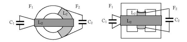
It is very like radio broadcasting, where the receiver is located far away from the transmitter, and has no feedback. The first coil works in **parallel resonance** and the second coil in **serial resonance** (although the two schematic diagrams look alike).
