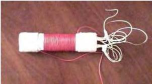
The coils are constructed from 5 sections, made from E-type ferrite core with a permeability of 2500, and wound using plastic-covered wire. The central sections L2 have 25 turns, and edge sections have 36 turns (to equalise the voltage on them). All sections are connected in parallel. The coil Ls has field-flattening turns at it's ends, and a single-layer winding Ls was used, the number of turns depending on the diameter of the wire used.
