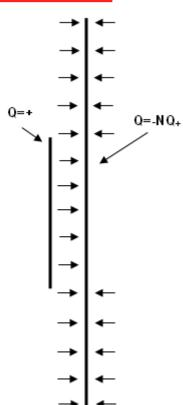
**COMMENT:** Charges from the ground will run on to the right hand plate <u>UNTIL</u> the moment when the external field drops to zero caused by the second spark ("S2"). It takes more charges flowing from the ground to annihilate the external field at the instant of the second spark, because the capacitance of the plate on the right is far greater. 'More charge' means 'more current', so you have achieved current amplification through this arrangement.
