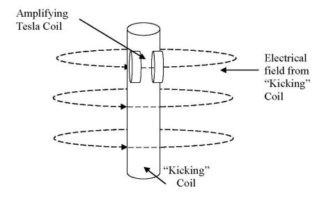
The electrical field of the driving pulse or "kicking" coil will charge the spread capacitors of the inductor, and the process will be started. Use pulses as short as possible in "kicking" coil, because the displacement current depends on the speed of the changes in the magnetic field.
