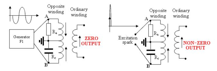
If the circuit is excited by the very sharp, positive-only, DC voltage spike produced by a spark, then the impedances of Ra and Rc are not the same and there is a non-zero output.
