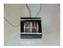
A coil was wound on a transformer ferromagnetic core (the size is not important) with permeability 2500 (not important) which was designed as a power-supply transformer. Each half-coil was 200 turns (not important), of 0.33 mm diameter wire (not important). The total inductance  $L_S$  is about 2 mH (not important).
