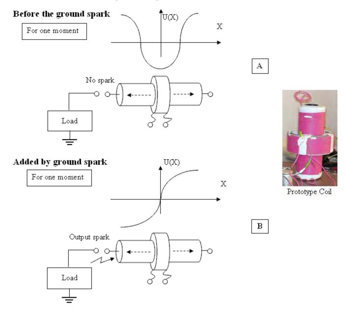
**EXPLANATION** The task of the oscillating circuit is to create a local electromagnetic field with a large electrical component. In theory, it would only be necessary to charge up the high voltage capacitor just once and then a lossless circuit would maintain the oscillations indefinitely without needing any further power input. In reality, there are some losses and so some additional power input is needed.
