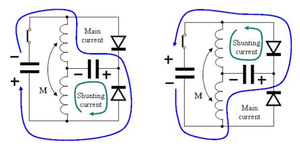
The main and the shunting currents run through the same output capacitor in one direction, if the output capacitor is discharged.
