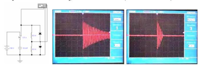
**The result:** A contour (oscillation circuit) is not destroyed, but it is shunted a lot. One can explain it by considering the moments when both diodes are conducting and so, shunt the circuit. As an addition, the voltage on the down diode is shown (the time scale is stretched). The negative voltage is close to maximum.
