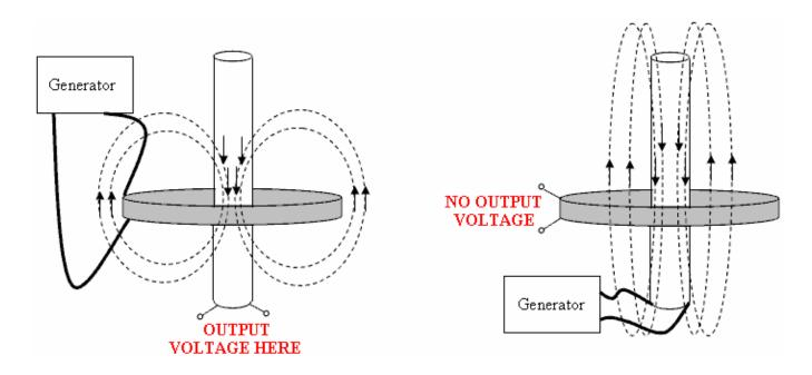
**EXPLANATION:** The "short" coil is not able to see the oscillations in the "long" coil, because the total number of magnetic lines from the "long" coil which are passing through the "short" coil is close to zero (because one half is in one direction and the other half is in the opposite direction).
