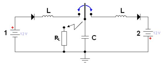
**EXPLANATION:** Batteries 1 and 2 are connected to the capacitor C alternately, through the inductances L. Voltage on capacitor C and the voltage from the batteries are increasing. As a result, there can be unlimited voltage rise. When the voltage on the capacitor reaches the desired level, it is connected to the load.
