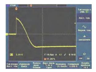
**The result confirms the prediction** – the remaining energy is more than the capacitor gives to the coil (with an accuracy of 20%).
