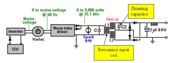
**COMMENTS:** The output coil can be adjusted to resonate with the input coil, but this is not important for understanding the principle. Excitation with just one spark is possible (not in resonance), but the frequency of the sparks influences the output power directly.
