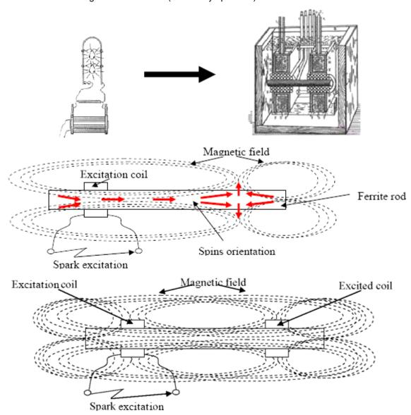
**COMMENT:** Excitation can be arranged in different ways, by coils connection. The frequencies of oscillations in a coil depends on the number of turns in it (a big variation is possible due to this factor).
