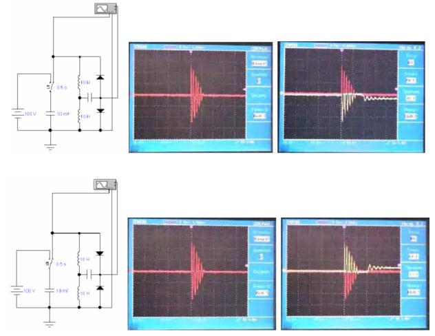
**Conditions:** The addition of a charging capacitor of 47 nano Farads.
