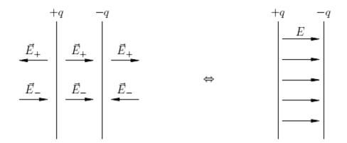
There is an electrical field only inside the capacitor. The electrical field outside the capacitor is zero (<u>because the fields cancel each other</u>).
