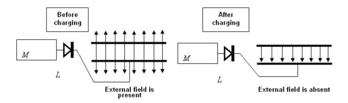
After the second plate of the capacitor has been charged, the external field becomes zero again. The charging system cannot "see" the field inside the capacitor once again and the process repeats again several times, raising the voltage until the spark gap connected to the output load discharges it.
