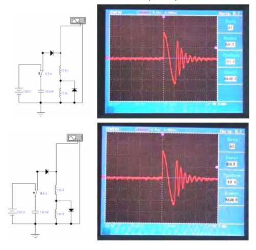
**The result:** The accuracy of capacitor recharging was improved to 5 percent (due to the removal of the influence of the first diode). After the main capacitor was switched off (by the diode), you can see oscillations caused by the spread capacitance of the inductors. Based on the frequency of the oscillations which were 4 to 5 times higher than that of the main capacitor, one can estimate the spread capacitance as being 16 to 25 times lower than the main capacitor.
