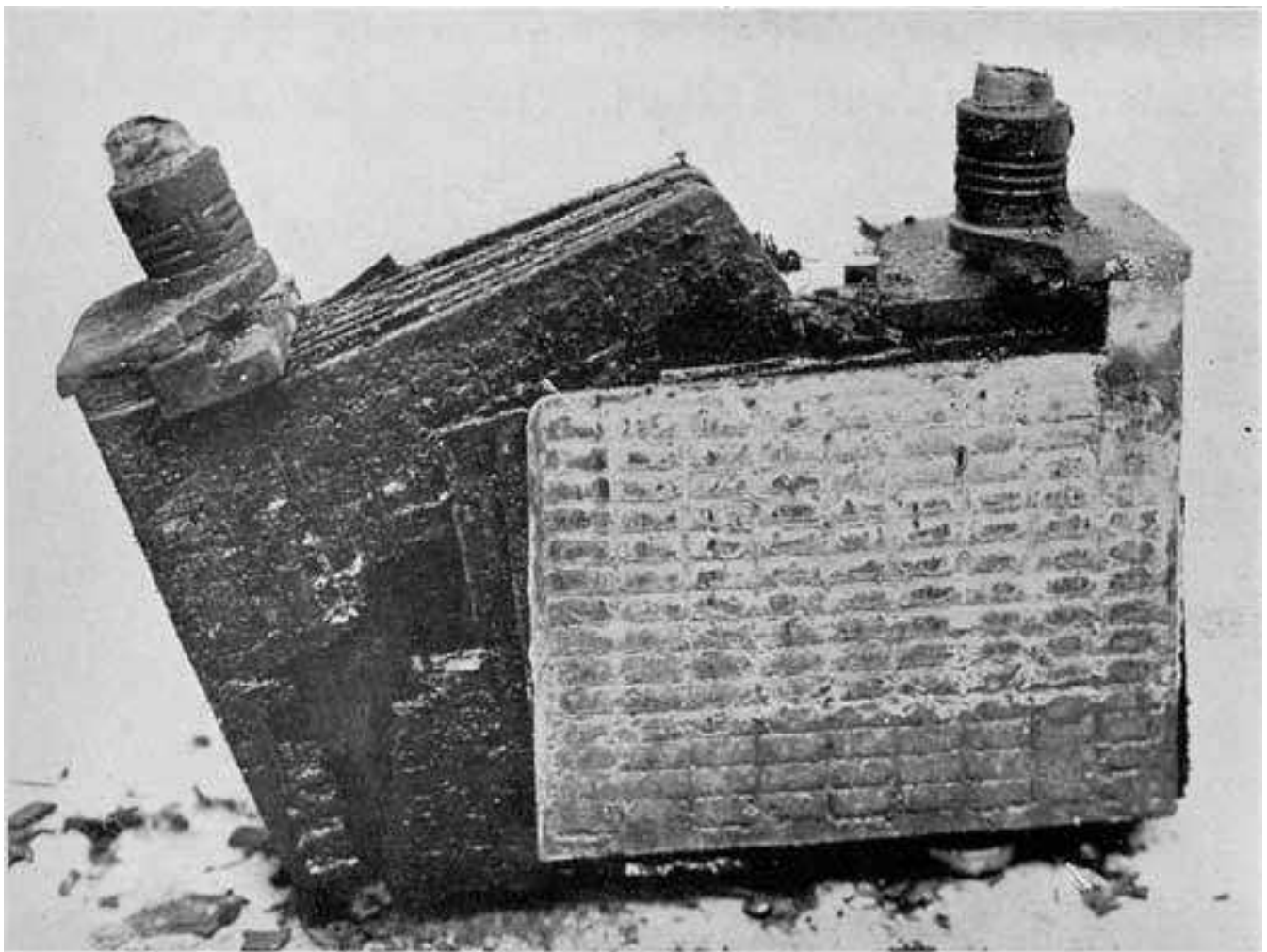
Fig. 209. Corroded, Bulged, and Sulphated Negatives. Disintegrated, Rotten Positives
