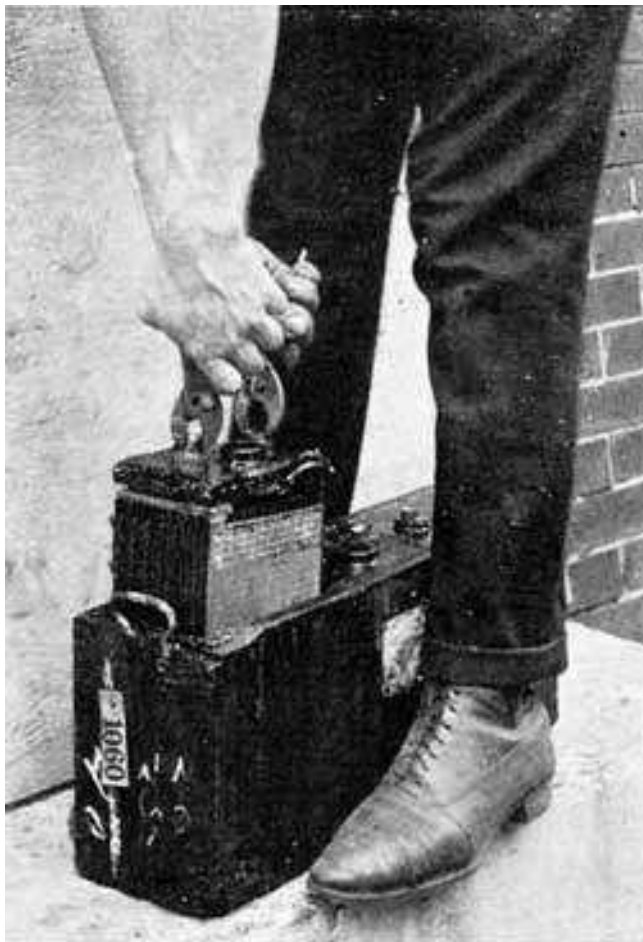
Fig. 196. Drawing up an Element
