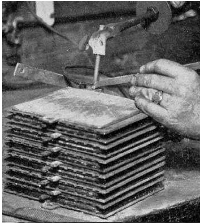
Fig. 322. Burning on Outside Negative Plate. Delco-Light Cell
