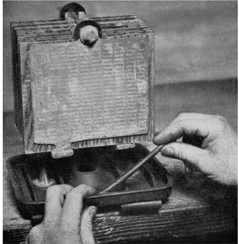
Fig. 314. Preparing Cover for Sealing. Delco-Light Cell
