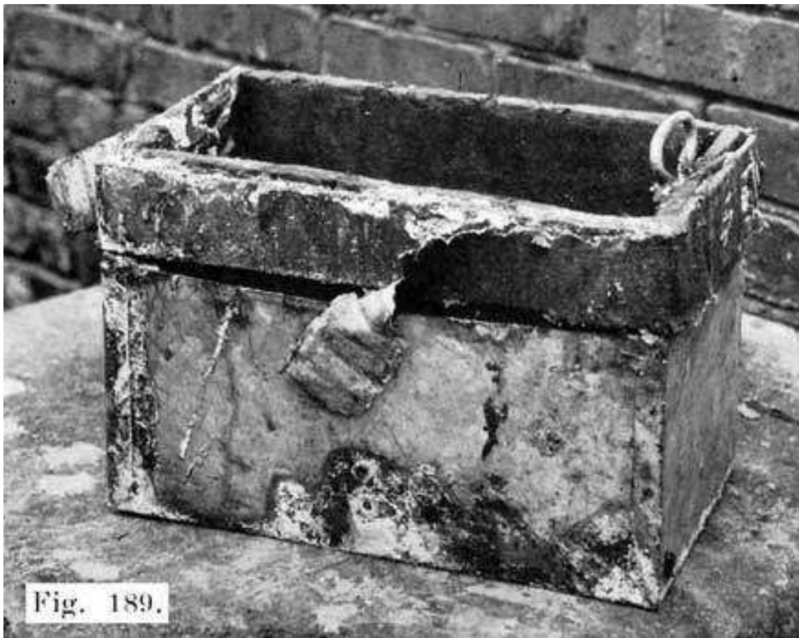
Fig. 189. A Blacksmith and Tinsmith Tried Their Hands on This Case, Lower Part Enclosed in Tin, Strap Iron, Covered with Friction Tape, Around The Top.
