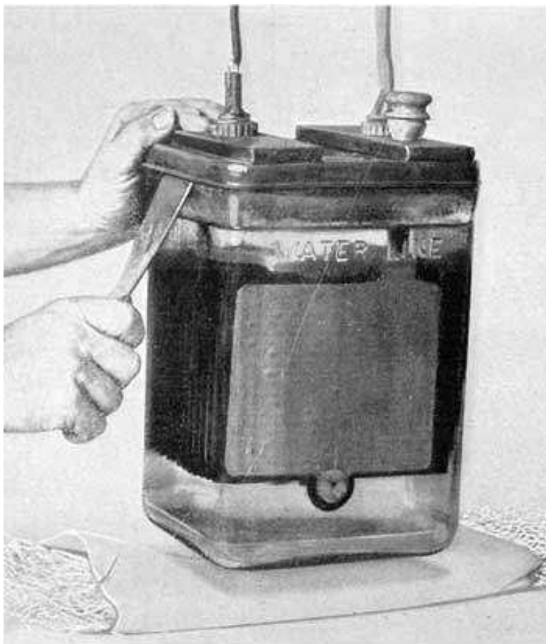
Fig. 306. Removing Delco-Light Cell Cover
