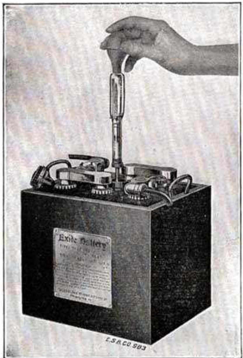
Fig. 35. Taking a Specific Gravity Reading
