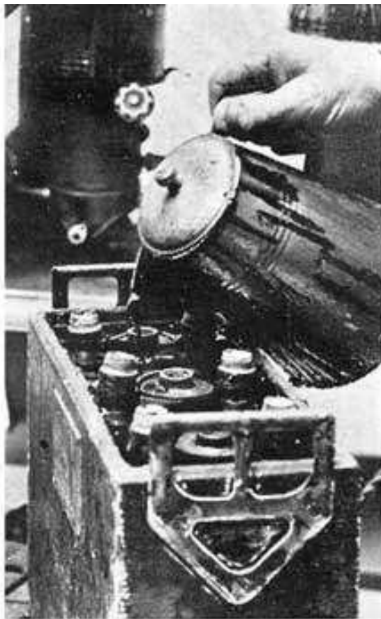
Fig. 229. Pouring Compound on Lower Covers
