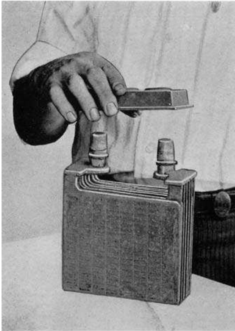
Fig. 252. Replacing Prest-O-Lite Cover on Built Up Posts
