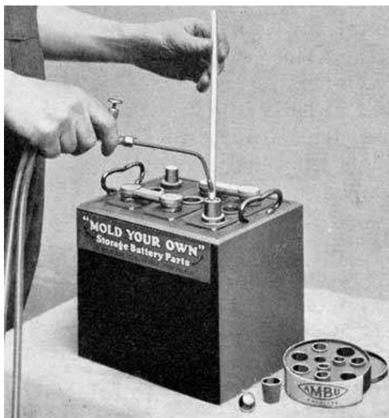
Fig. 101. Illustrating Use of Post Builders
