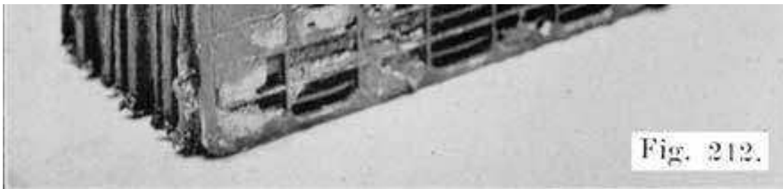
Fig. 212. Element from a "Slopper." Element was Loose in Jar. and Jolting of Car Caused Paste to Fall Out
