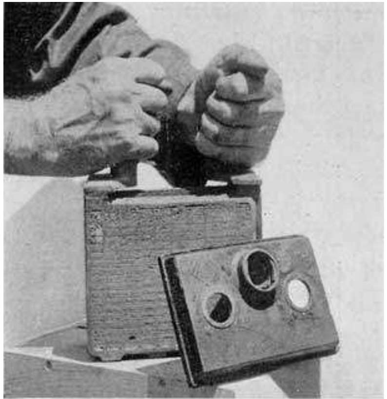
Fig. 227. Shifting Groups to Make Cover Fit
