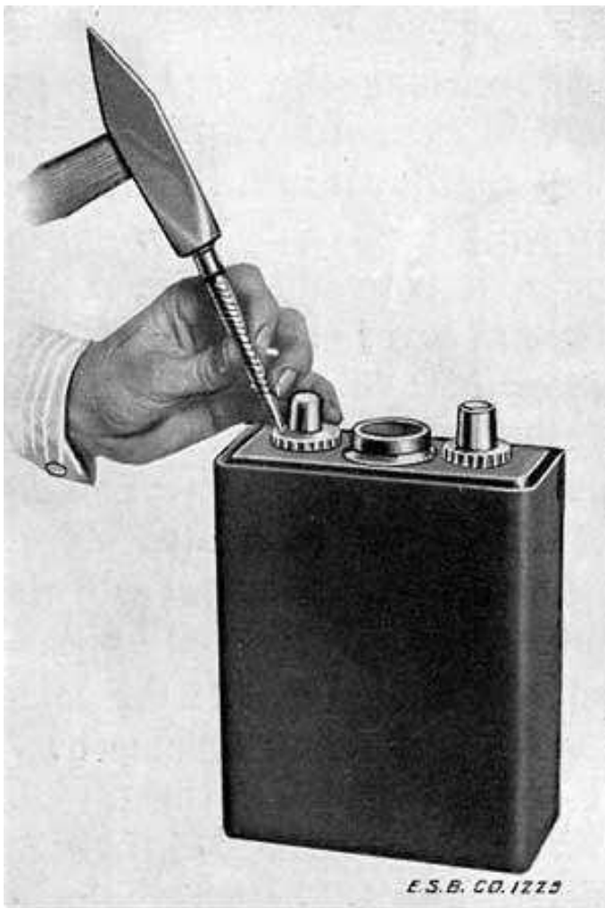
Fig. 241. Upsetting Threads to Prevent Nut from Turning
