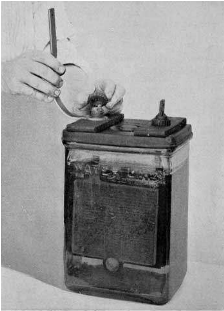
Fig. 321. Fastening Auxiliary Strap. Delco-Light Cell
