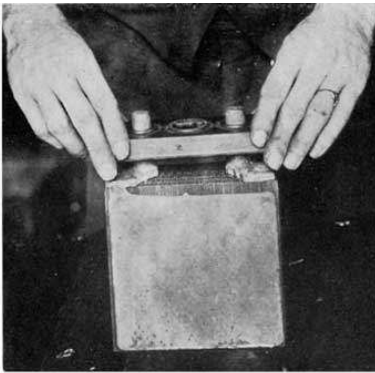
Fig. 258. Replacing Cover of Philadelphia Diamond Grid Battery
