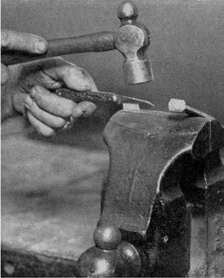
Fig. 318. Splitting End of Strap. Delco-Light Cell
