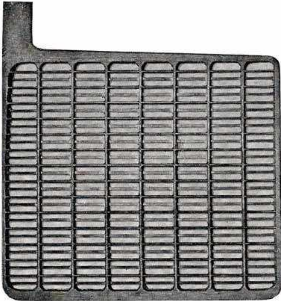
Fig. 4. Grid, Trimmed, and Ready for Pasting
