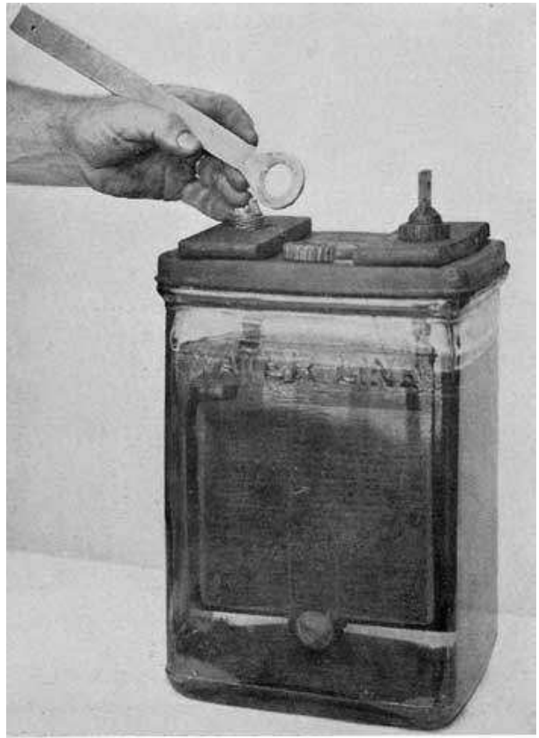
Fig. 320. Auxiliary Strap. Delco-Light Cell
