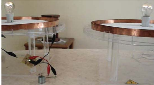
Fig.15: Two energized flat spiral or "pancake" Tesla coil showing streams in the top spherical capacitance lamp bulbs.
