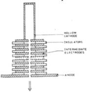
Generates Pulsed Electron Beams
